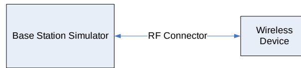
Figure 9-4 Power Measurement Setup
