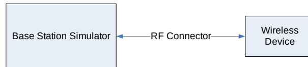
Figure 9-1 Power Measurement Setup
