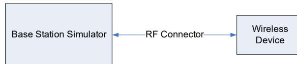
Figure 9-3 Power Measurement Setup
