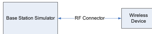
Figure 9-4 Power Measurement Setup
