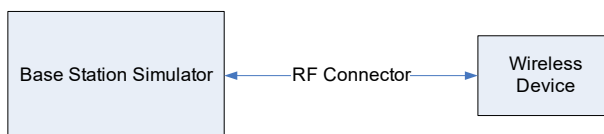
Figure 9-2 Power Measurement Setup
