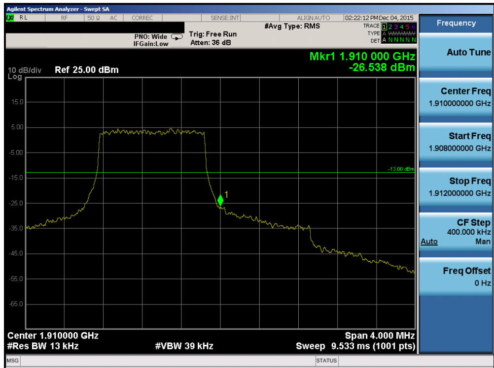
Plot 7-91. Upper Band Edge Plot (Band 2 – 1.4MHz QPSK – RB Size 6)
