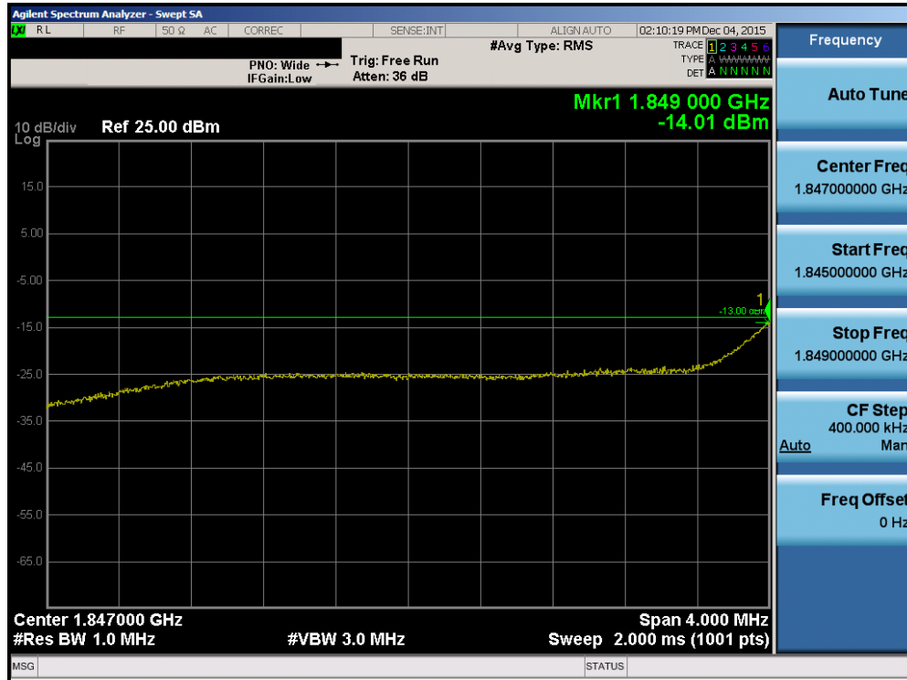
Plot 7-98. Lower Extended Band Edge Plot (Band 2 – 5.0MHz QPSK – RB Size 25)
