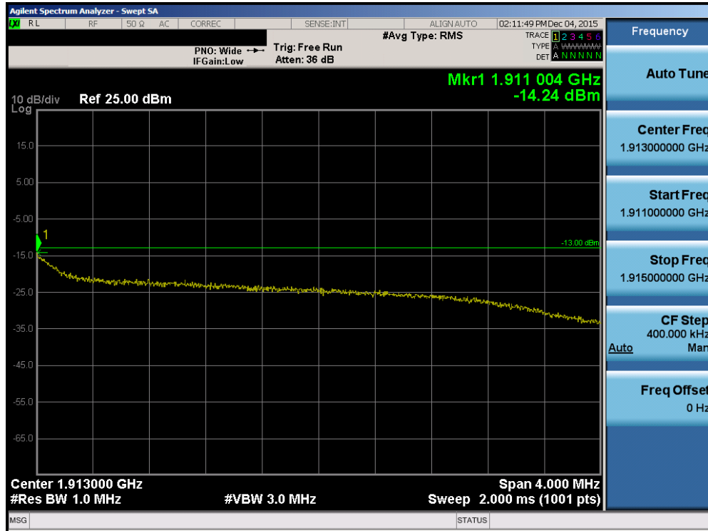
Plot 7-100. Upper Extended Band Edge Plot (Band 2 – 5.0MHz QPSK – RB Size 25)
