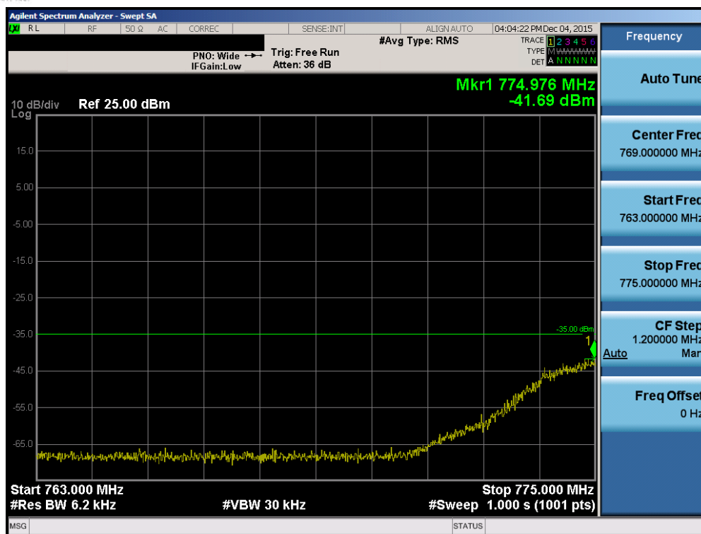
Plot 7-58. Lower Emission Mask Edge Plot (Band 13 – 5.0MHz QPSK – RB Size 25)
