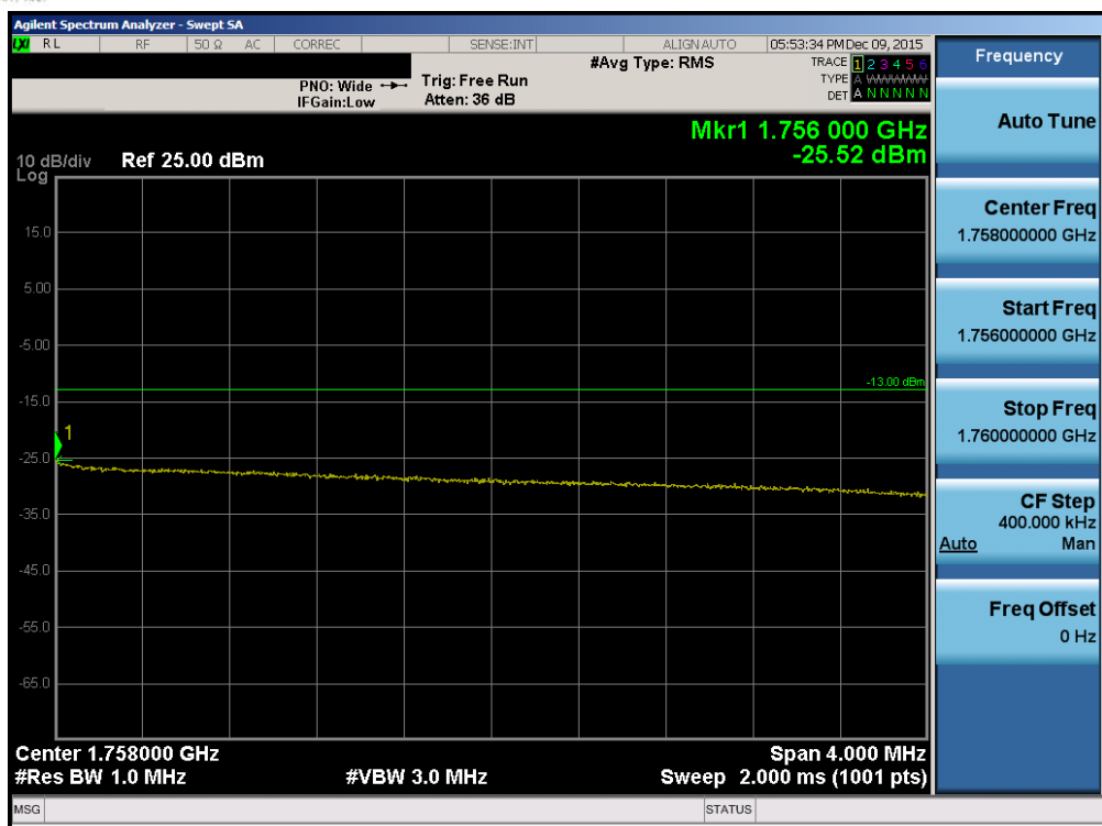
Plot 7-80. Upper Extended Band Edge Plot (Band 4 – 10.0MHz QPSK – RB Size 50)
