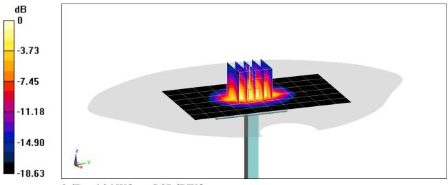
DUT: Dipole 1900 MHz; Type: D1900V2; Serial: 5d149
