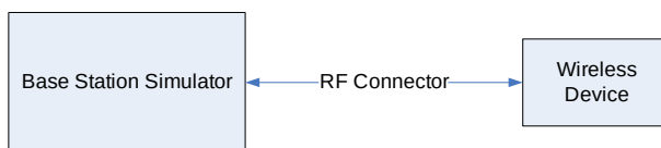
Figure 9-2 Power Measurement Setup
