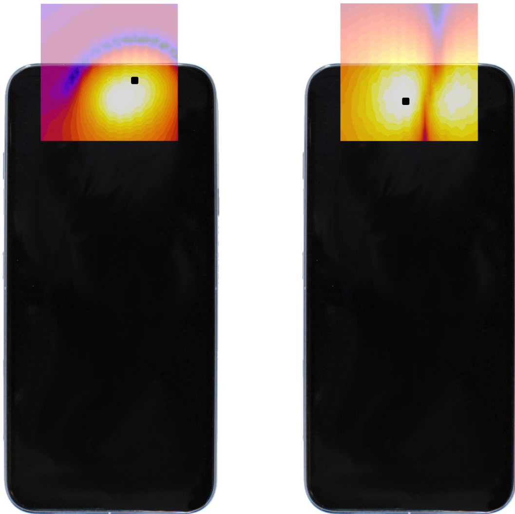
Figure 16-3 T-Coil Scan Overlay Magnetic Field Distributions
