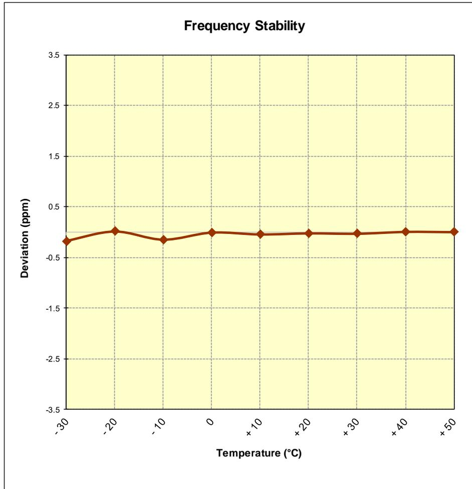
Figure 7-15. Frequency Stability Graph (PCS WCDMA Mode – Ch. 9400)
