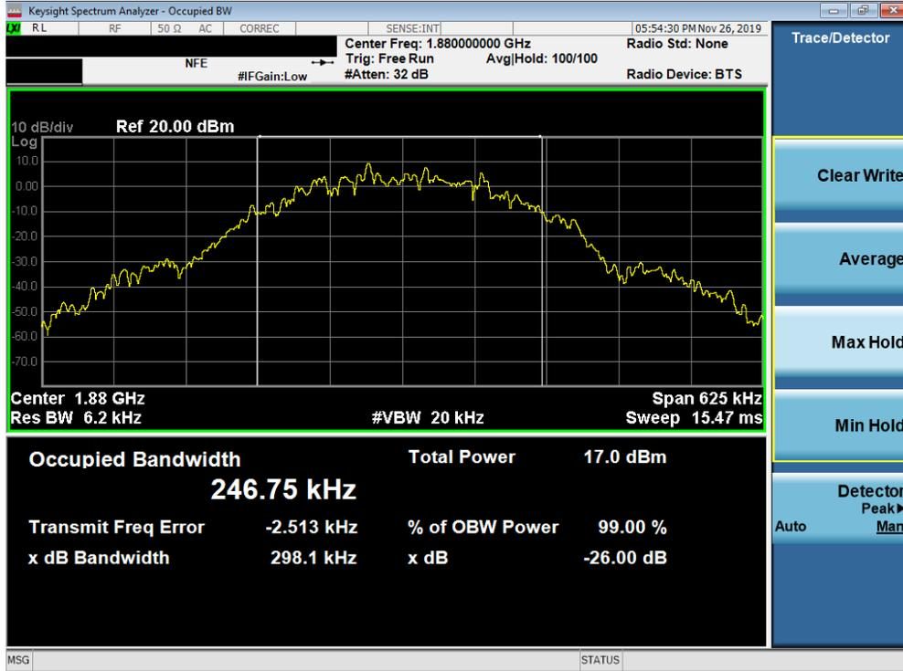
Plot 7-3. Occupied Bandwidth Plot (PCS GPRS Mode)
