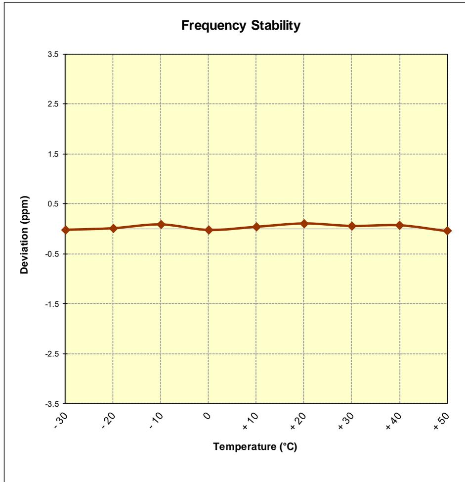
Figure 7-14. Frequency Stability Graph (PCS CDMA Mode – Ch. 600)
