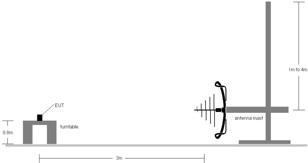
**Figure 7-7. Test Instrument & Measurement Setup < 1GHz**
