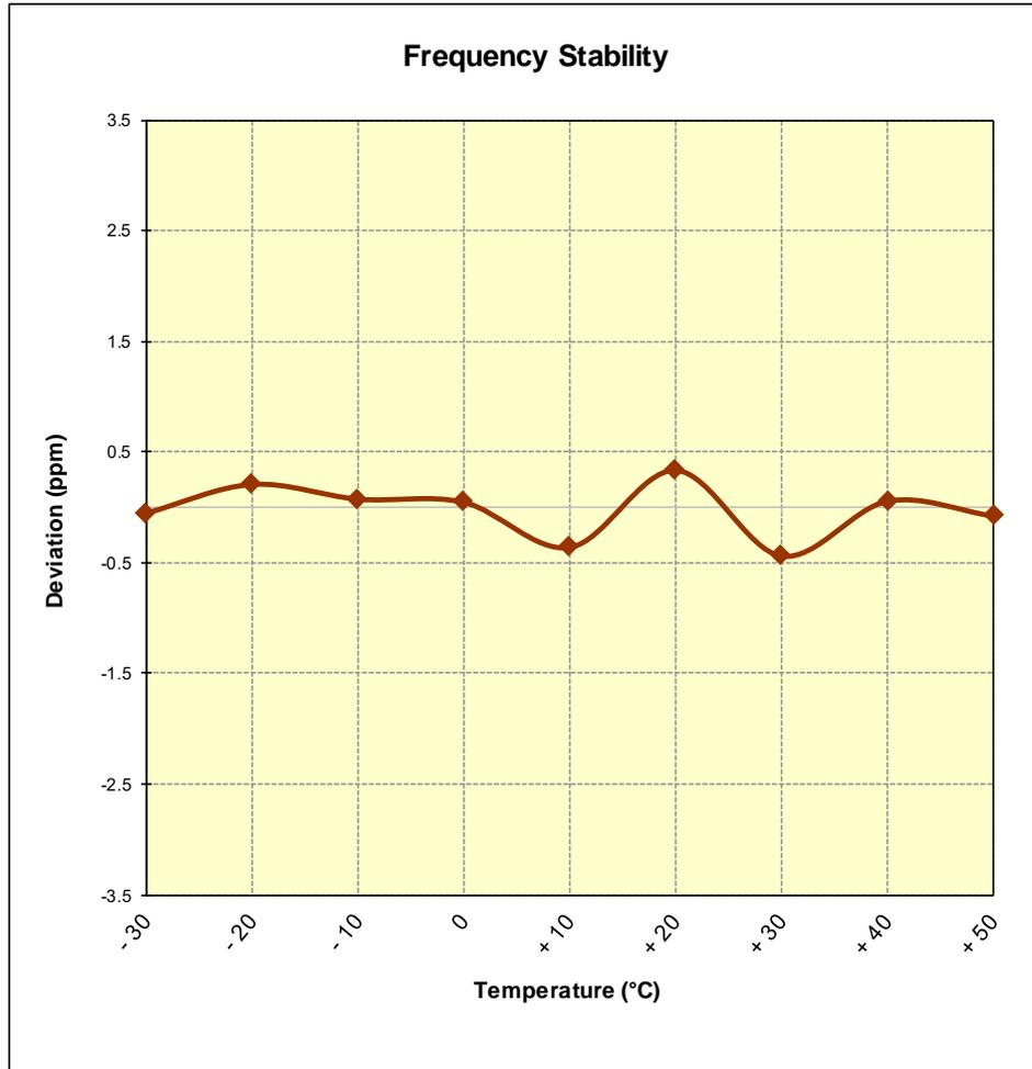
Figure 7-11. Frequency Stability Graph (Cellular WCDMA Mode – Ch. 4183)
