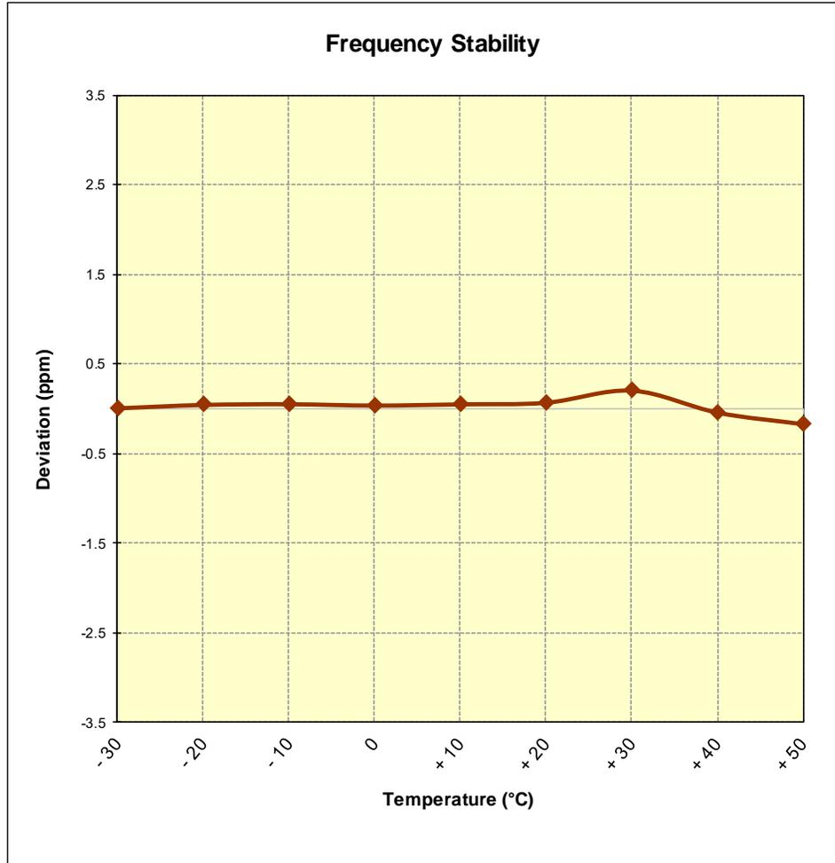
Figure 7-12. Frequency Stability Graph (AWS WCDMA Mode – Ch. 1413)
