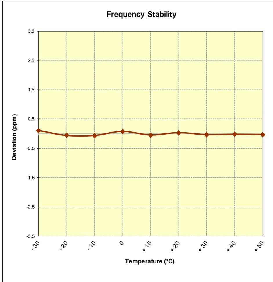
Figure 7-13. Frequency Stability Graph (PCS GPRS Mode – Ch. 661)
