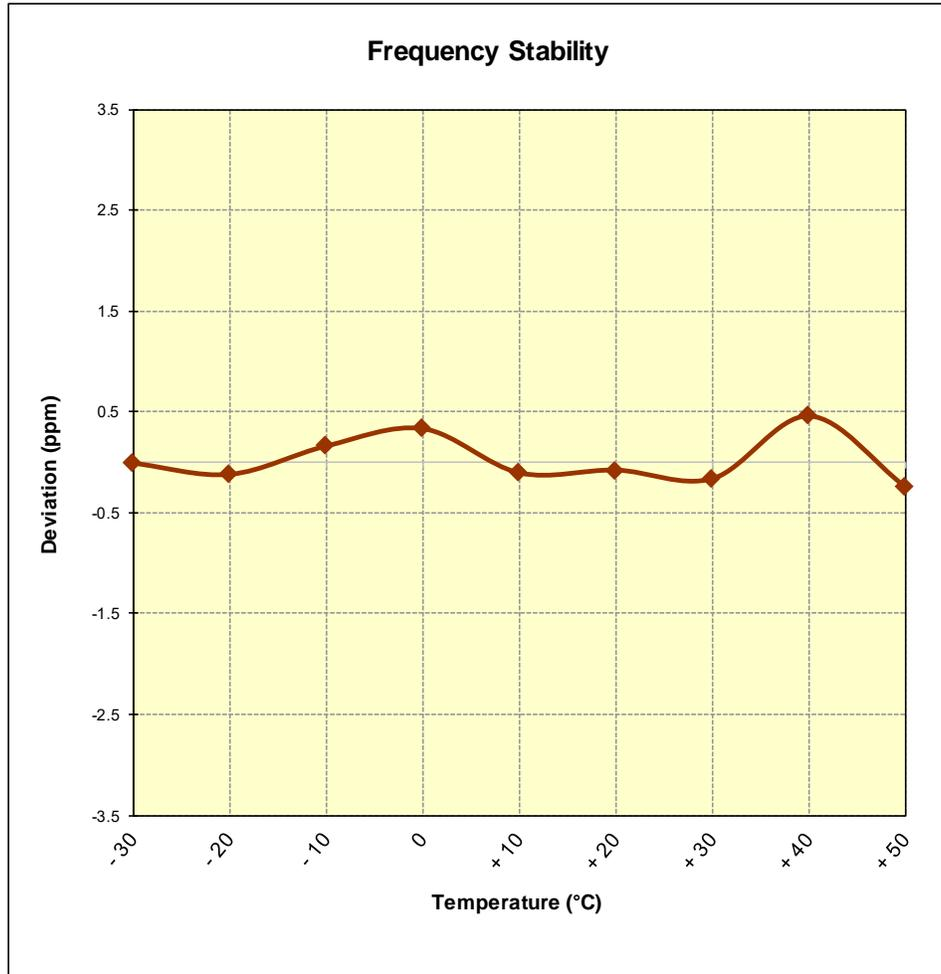
Figure 7-10. Frequency Stability Graph (Cellular CDMA Mode – Ch. 384)
