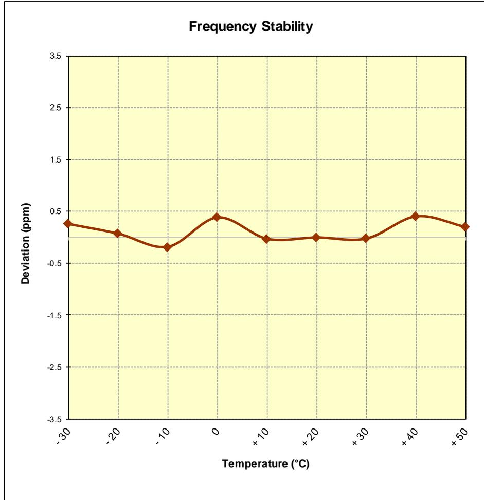
Figure 7-9. Frequency Stability Graph (Cellular GPRS Mode – Ch. 190)
