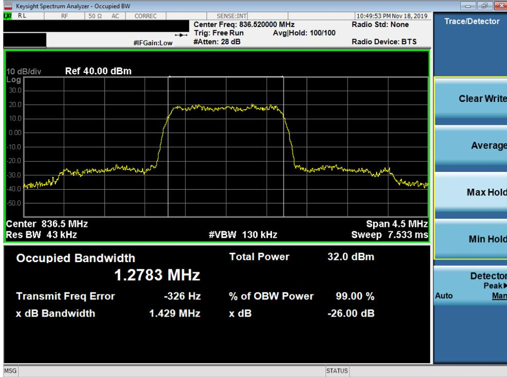
Plot 7-5. Occupied Bandwidth Plot (Cellular CDMA Mode)
