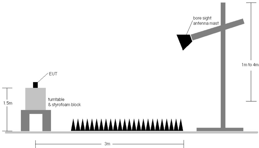
**Figure 7-8. Test Instrument & Measurement Setup >1 GHz**
