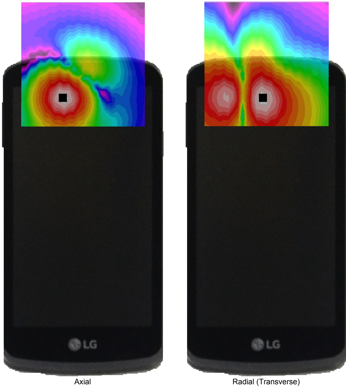
Figure 13-3 T-Coil Scan Overlay Magnetic Field Distributions
