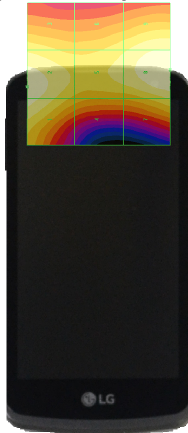
Figure 18-4 E-Field WD Scan overlay
