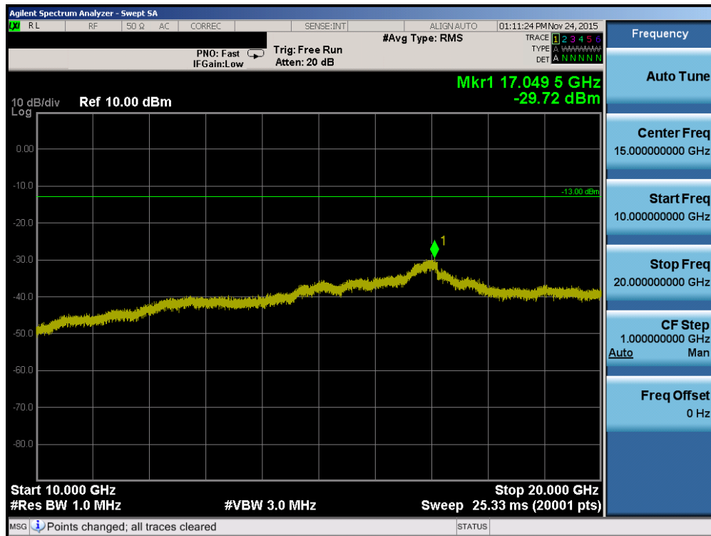
Plot 7-43. Conducted Spurious Plot (AWS WCDMA Mode – Ch. 1513)
