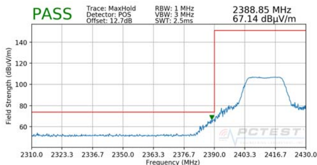
Plot 7-36. Radiated Restricted Lower Band Edge Measurement (Peak)
