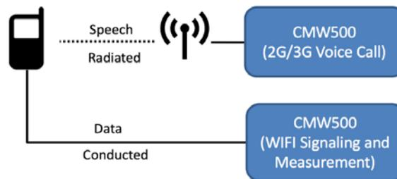
Figure 1 – Verification of WIFI Power Reduction
