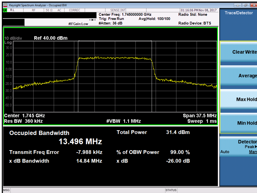
Plot 7-32. Occupied Bandwidth Plot (Band 4/66 - 15.0MHz 16-QAM - Full RB Configuration)
