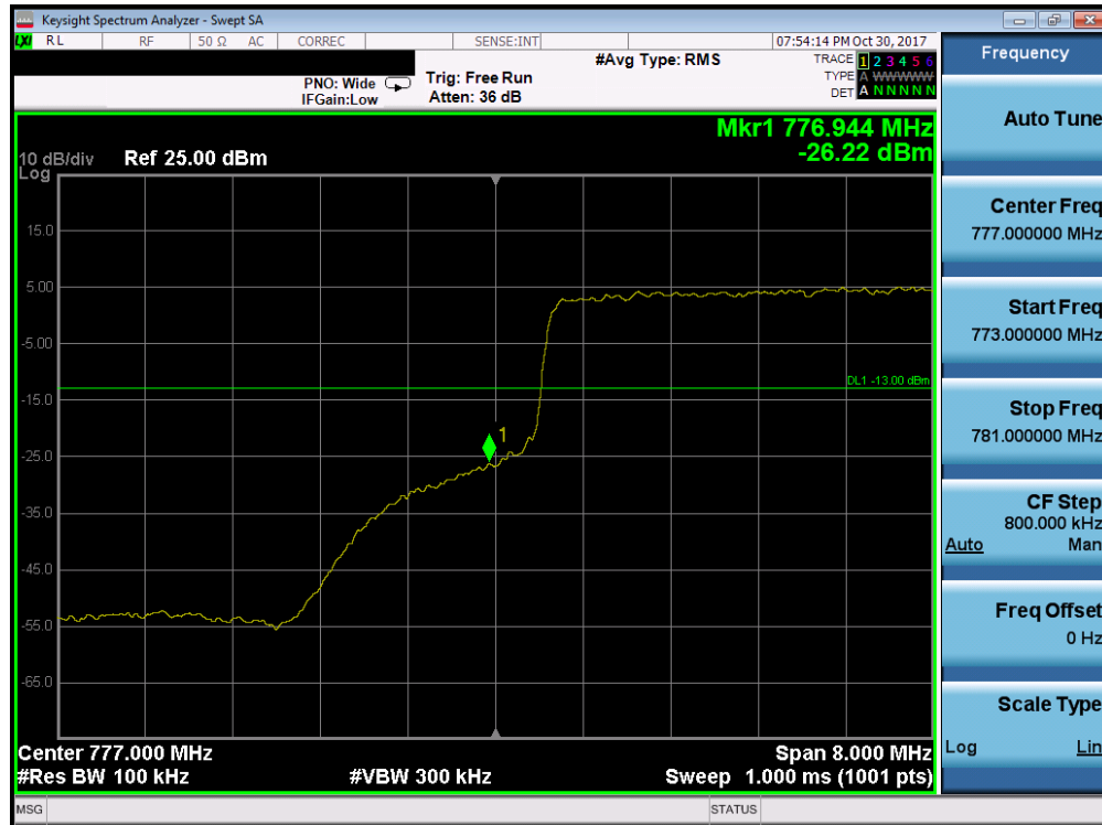
Plot 7-98. Lower Band Edge Plot (Band 13 - 10.0MHz QPSK - Full RB Configuration)
