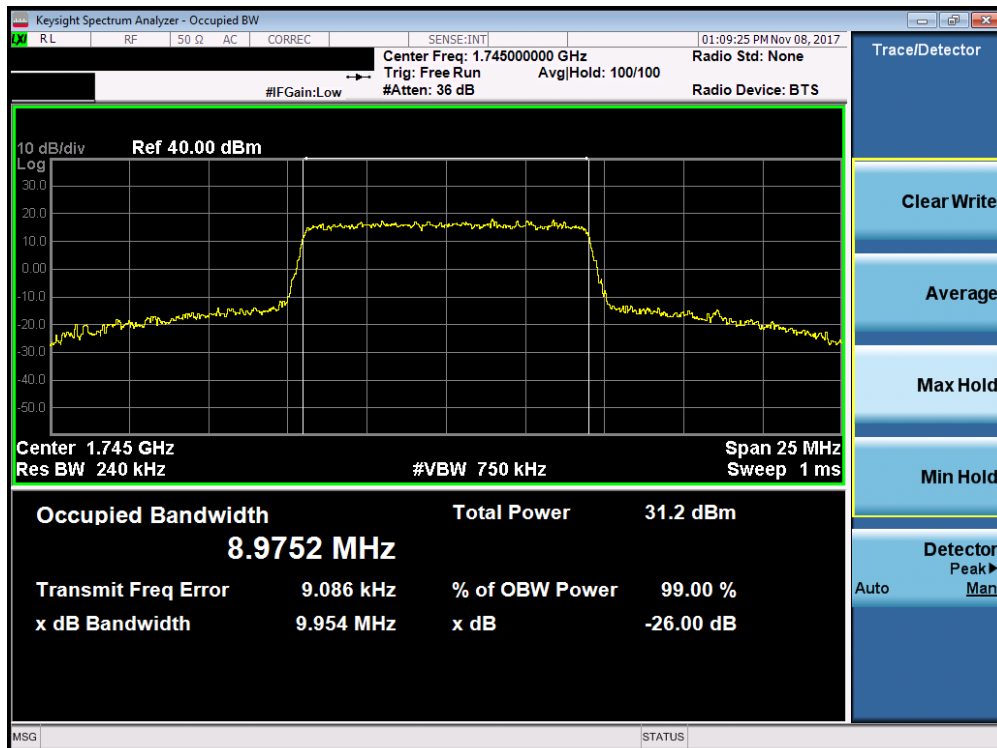
Plot 7-30. Occupied Bandwidth Plot (Band 4/66 - 10.0MHz 16-QAM - Full RB Configuration)
