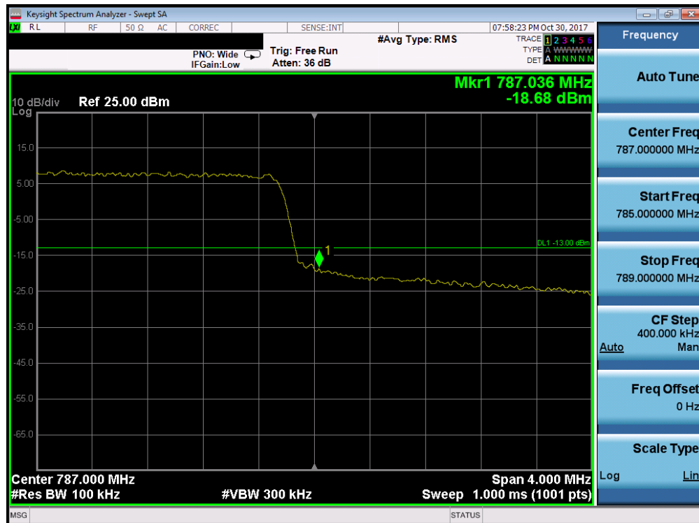
Plot 7-95. Upper Band Edge Plot (Band 13 - 5.0MHz QPSK - Full RB Configuration)
