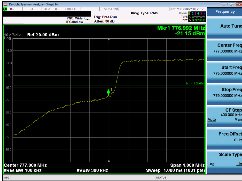
Plot 7-94. Lower Band Edge Plot (Band 13 - 5.0MHz QPSK - Full RB Configuration)
