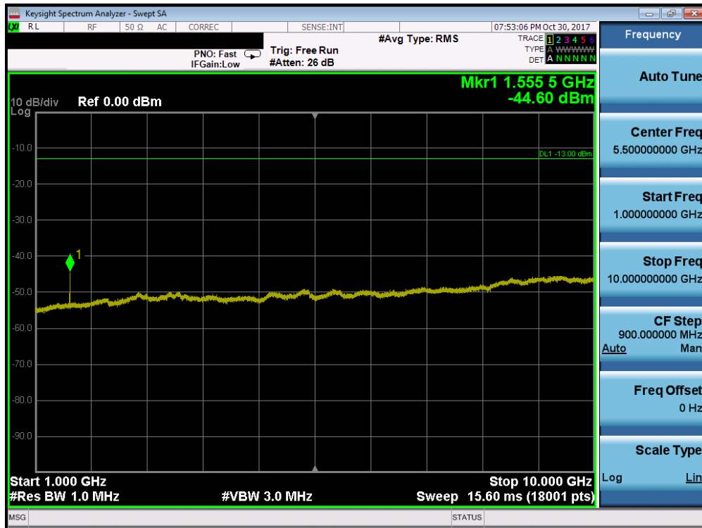
Plot 7-58. Conducted Spurious Plot (Band 13 - 10.0MHz QPSK - RB Size 1, RB Offset 0)
