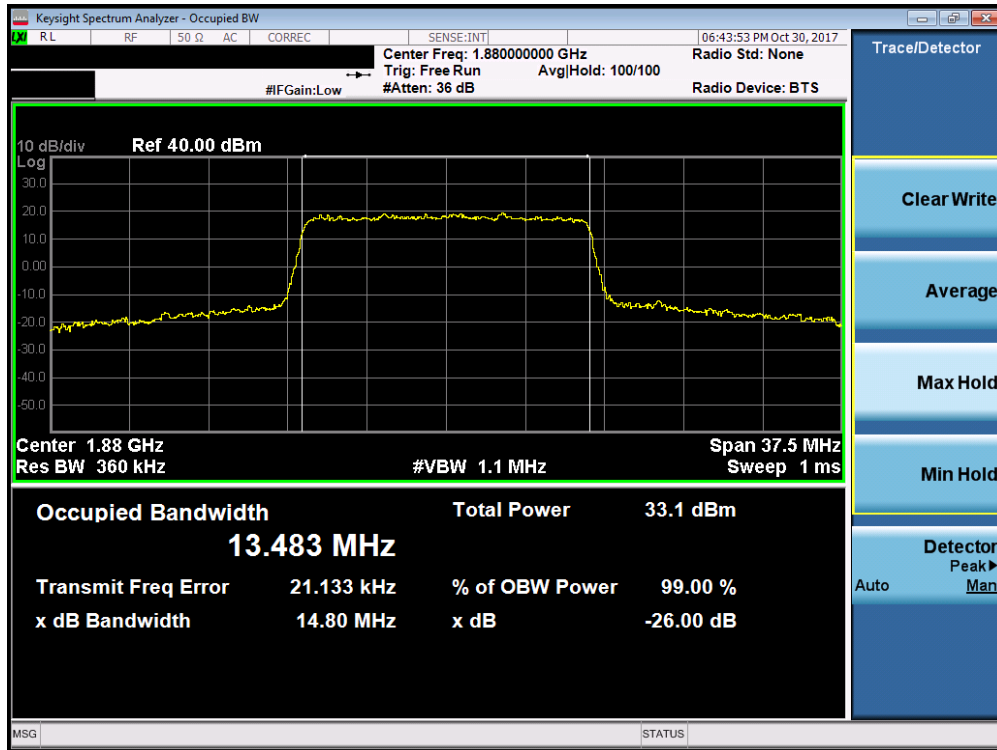
Plot 7-43. Occupied Bandwidth Plot (Band 2 - 15.0MHz QPSK - Full RB Configuration)
