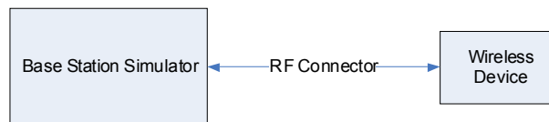
Figure 9-1 Power Measurement Setup
