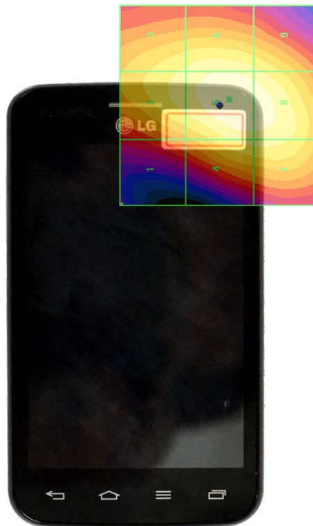
Figure 18-4 E-Field WD Scan overlay (T-coil centered scan grid shown)
