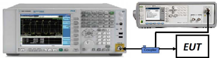
Figure 7-4. Test Instrument & Measurement Setup
