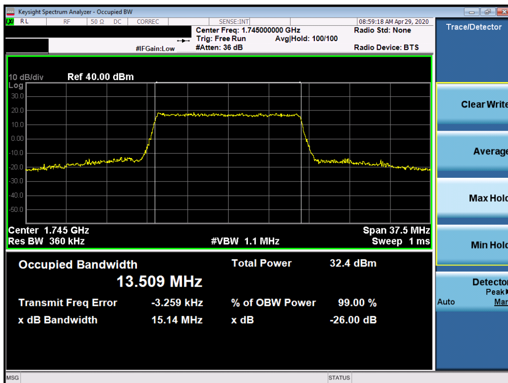
Plot 7-4. Occupied Bandwidth Plot (LTE Band 66/4 - 15MHz QPSK - Full RB Configuration)
