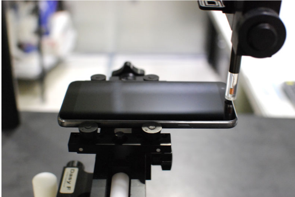
Figure 16-1 Test Setup for Wireless Device
