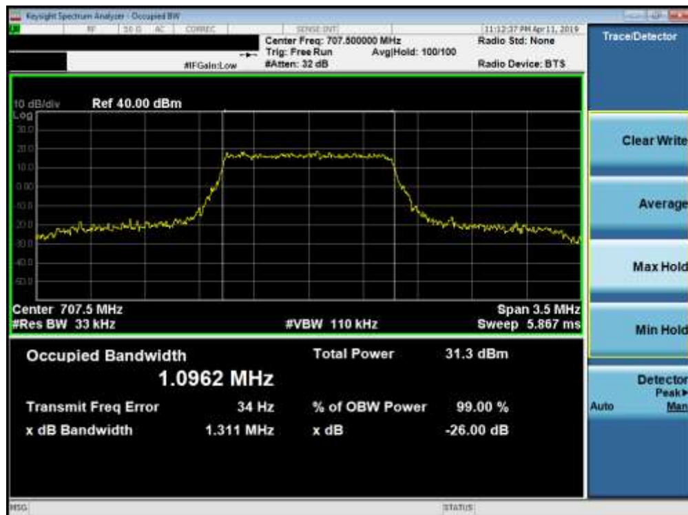
Plot 7-10. Occupied Bandwidth Plot (Band 12 - 1.4MHz 16-QAM - Full RB Configuration)
