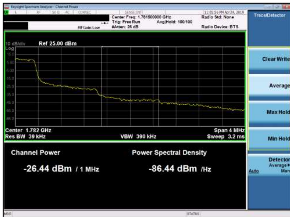
Plot 7-143. Upper Extended Band Edge Plot (Band 66 - 1.4MHz QPSK - Full RB Configuration)
