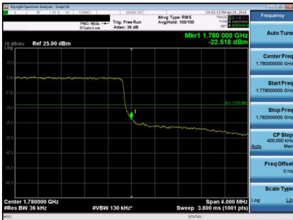
Plot 7-148. Upper Band Edge Plot (Band 66 - 3.0MHz QPSK - Full RB Configuration)
