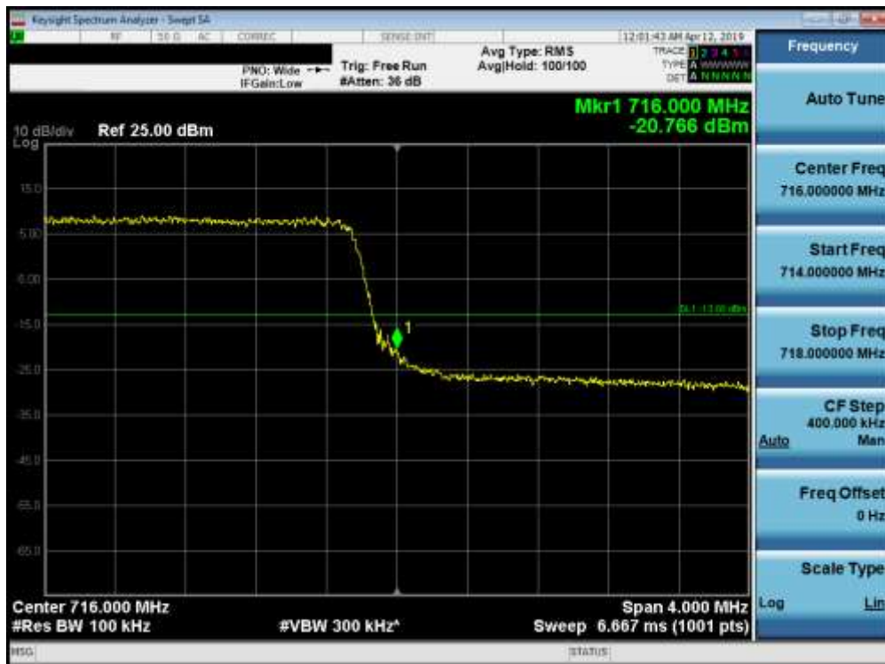
Plot 7-118. Upper Band Edge Plot (Band 12/17 - 5.0MHz QPSK - Full RB Configuration)
