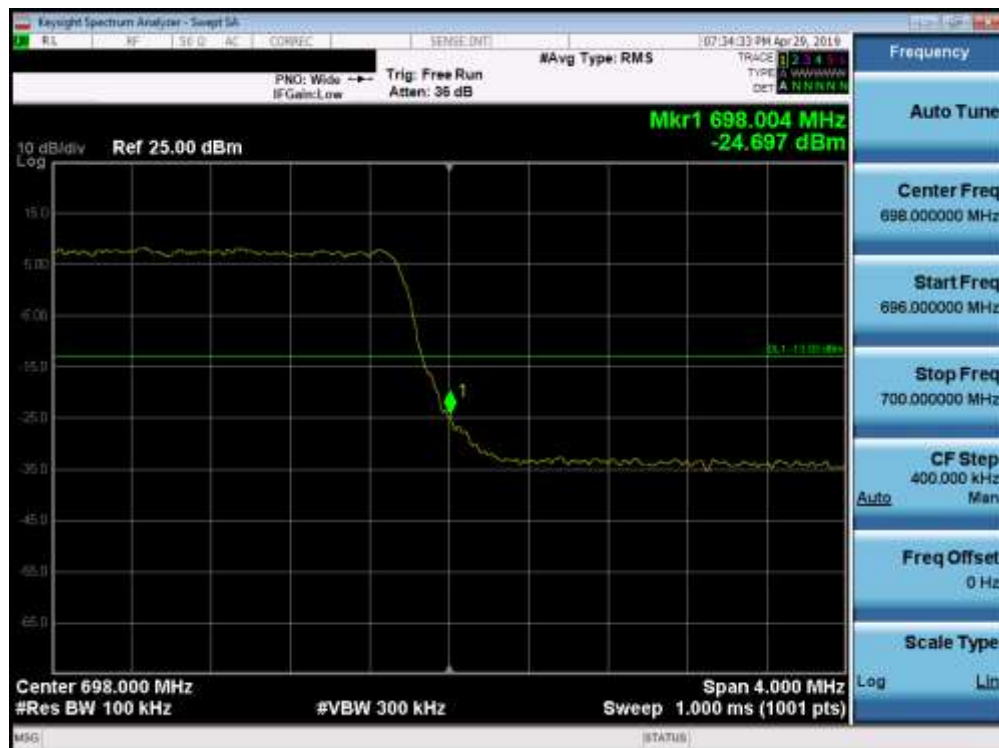
Plot 7-105. Upper Band Edge Plot (Band 71 - 5.0MHz QPSK - Full RB Configuration)
