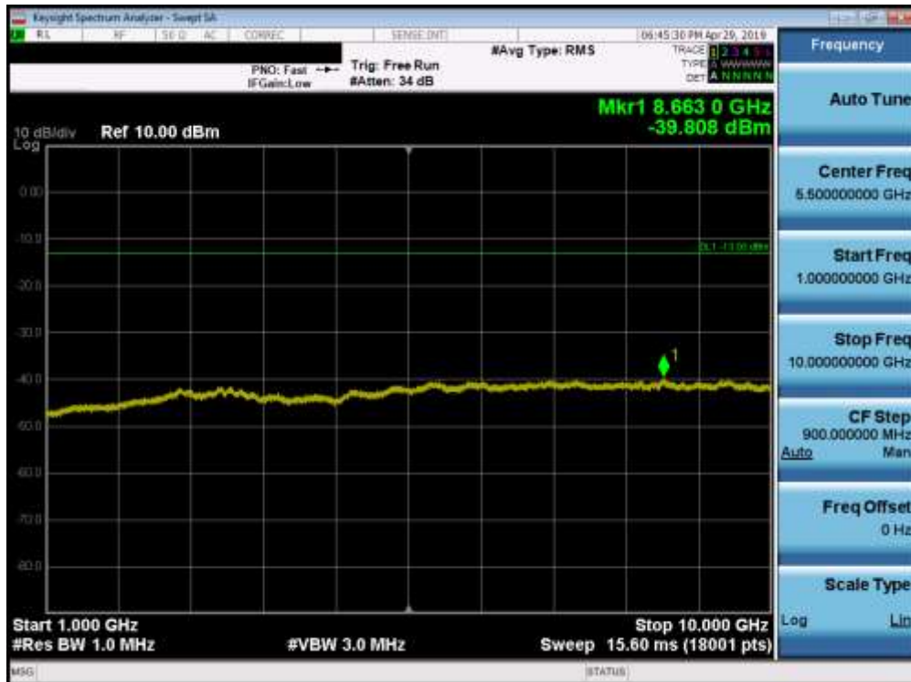
Plot 7-58. Conducted Spurious Plot (Band 71 - 20.0MHz QPSK - RB Size 1, RB Offset 0 - Mid Channel)
