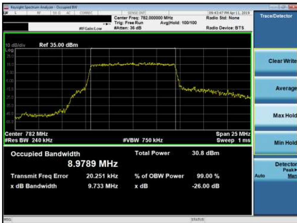
Plot 7-20. Occupied Bandwidth Plot (Band 13 - 10.0MHz 16-QAM - Full RB Configuration)
