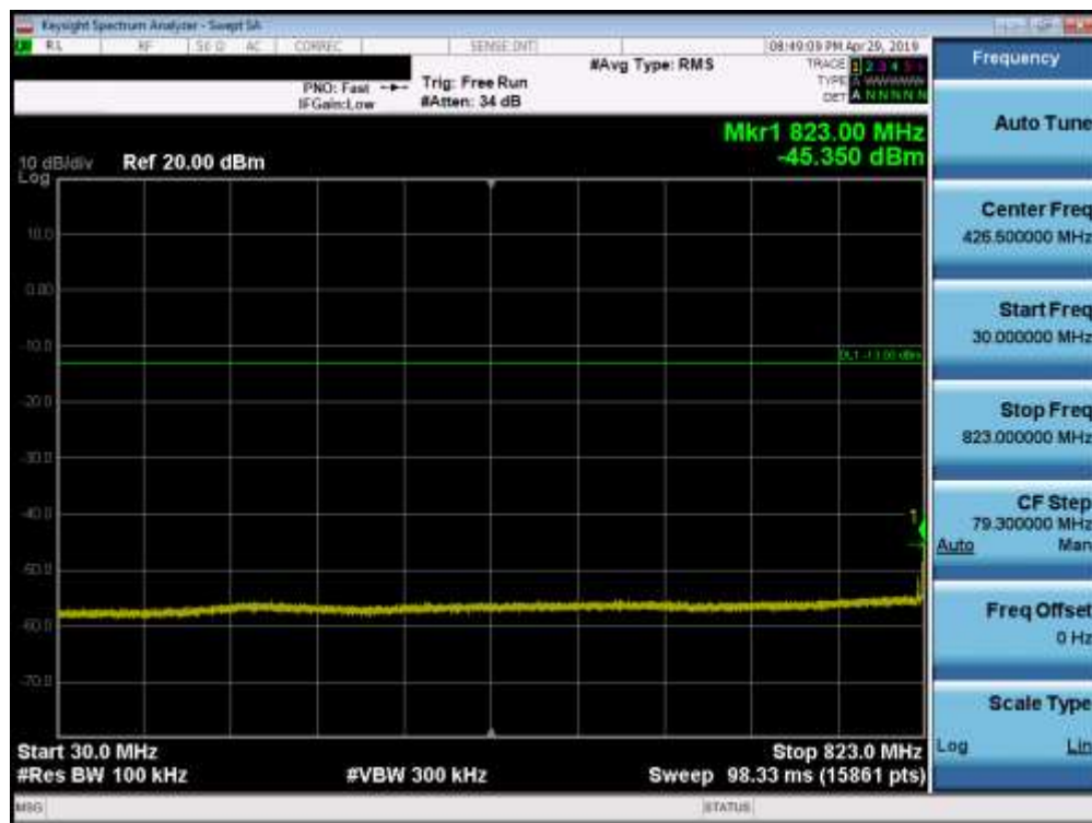
Plot 7-77. Conducted Spurious Plot (Band 5 - 10.0MHz QPSK - RB Size 1, RB Offset 0 - Low Channel)
