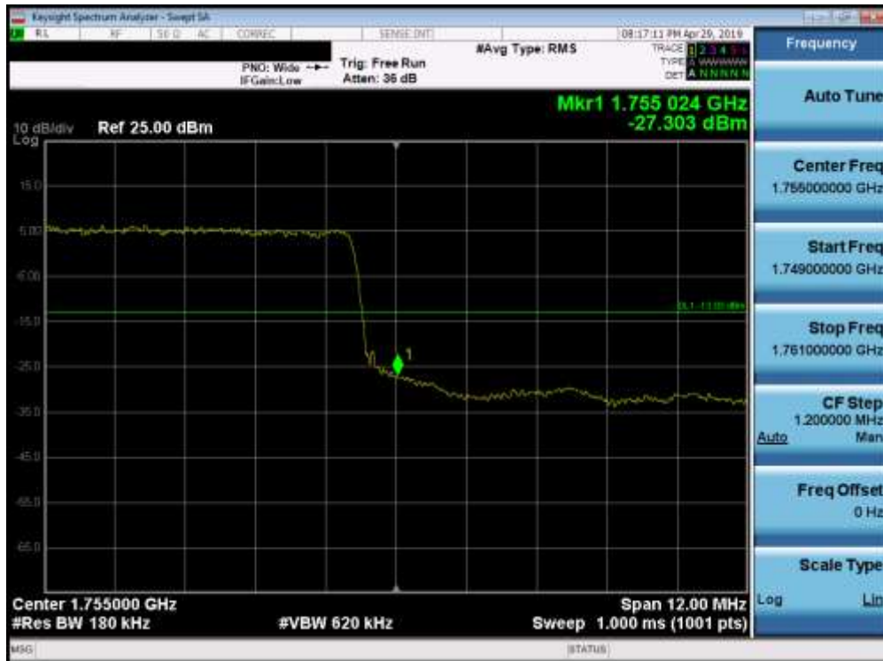
Plot 7-164. Upper Band Edge Plot (Band 4 - 15.0MHz QPSK - Full RB Configuration)
