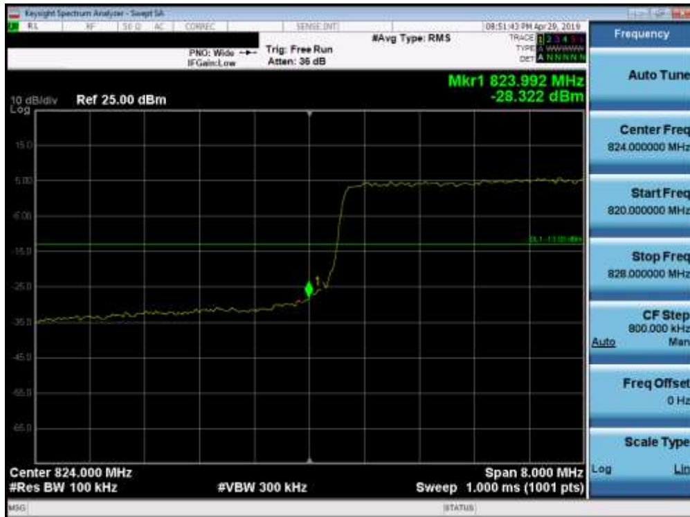
Plot 7-136. Lower Band Edge Plot (Band 5 - 10.0MHz QPSK - Full RB Configuration)
