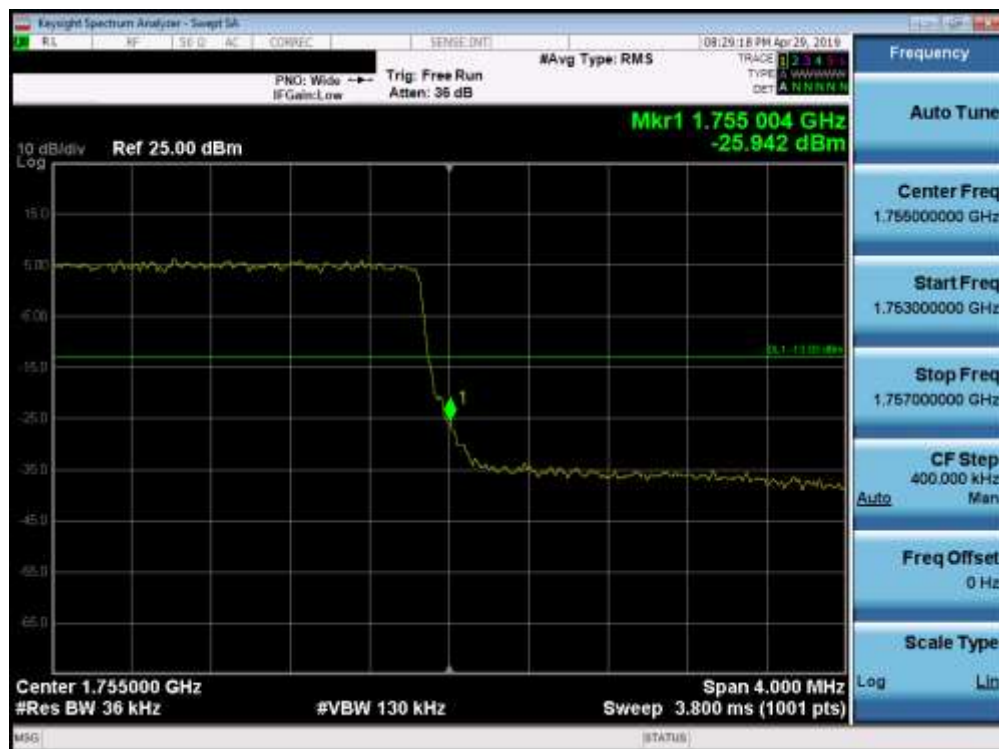
Plot 7-146. Upper Band Edge Plot (Band 4 - 3.0MHz QPSK - Full RB Configuration)
