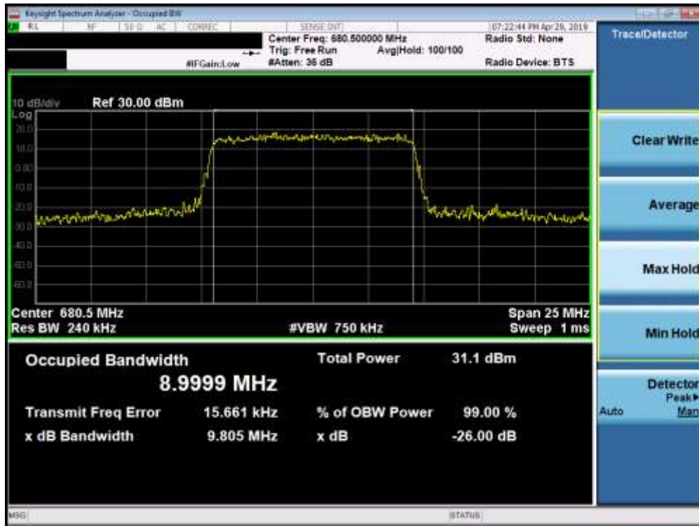
Plot 7-3. Occupied Bandwidth Plot (Band 71 - 10.0MHz QPSK - Full RB Configuration)
