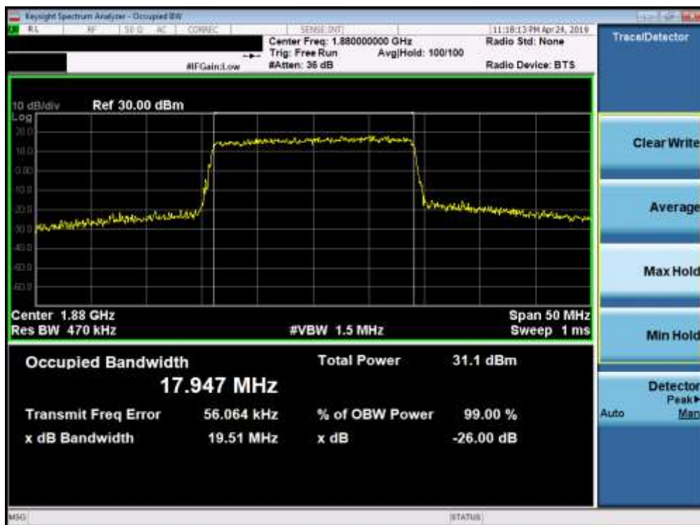
Plot 7-51. Occupied Bandwidth Plot (Band 2 - 20.0MHz QPSK - Full RB Configuration)
