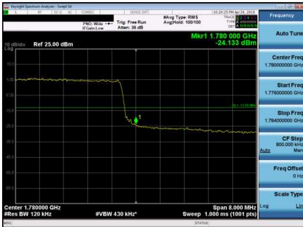
Plot 7-160. Upper Band Edge Plot (Band 66 - 10.0MHz QPSK - Full RB Configuration)
