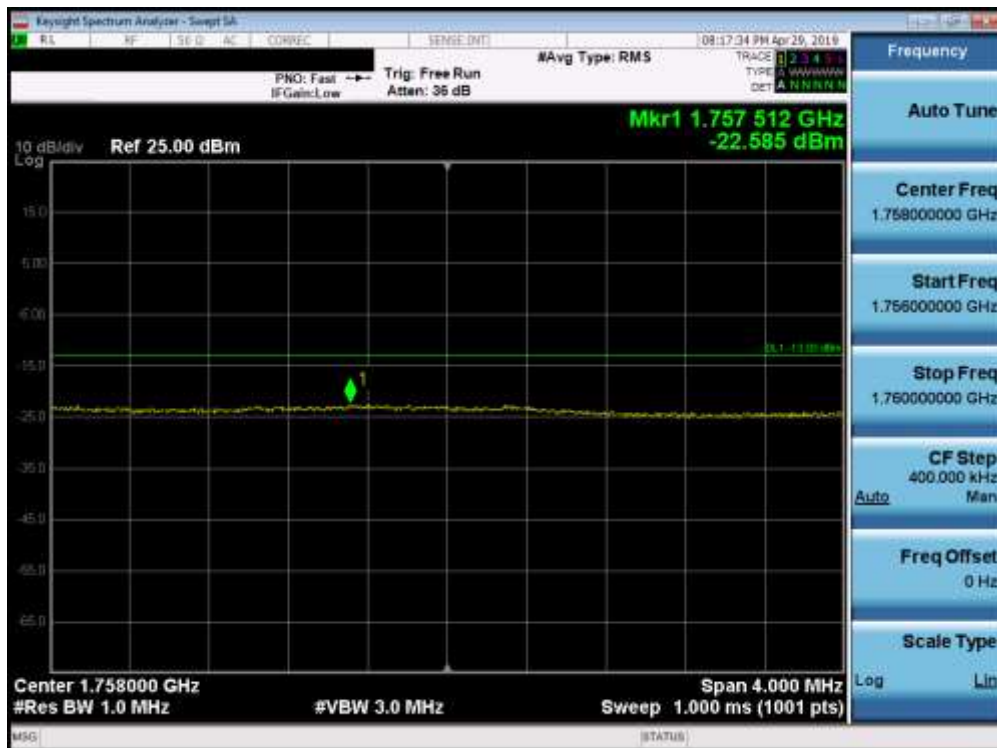
Plot 7-165. Upper Extended Band Edge Plot (Band 4 - 15.0MHz QPSK - Full RB Configuration)
