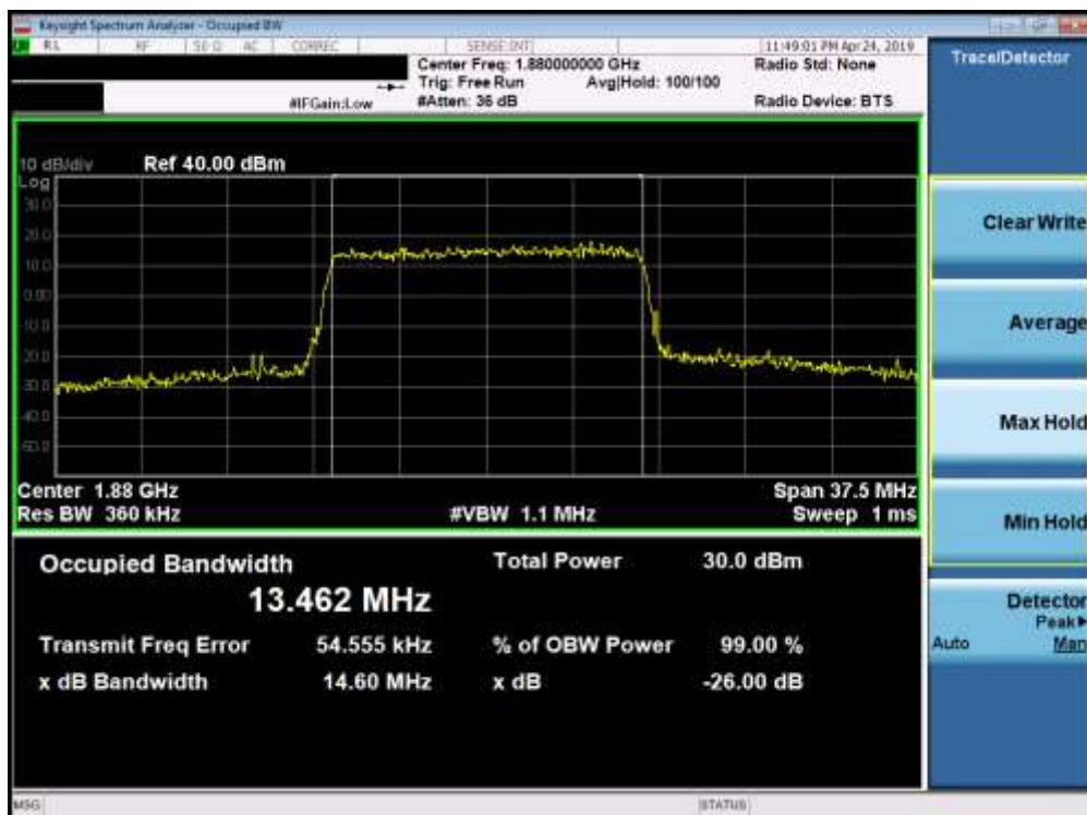
Plot 7-50. Occupied Bandwidth Plot (Band 2 - 15.0MHz 16-QAM - Full RB Configuration)
