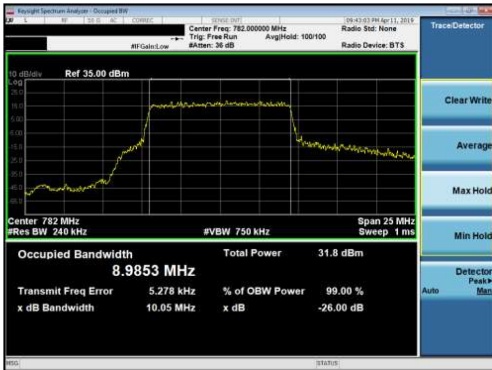
Plot 7-19. Occupied Bandwidth Plot (Band 13 - 10.0MHz QPSK - Full RB Configuration)
