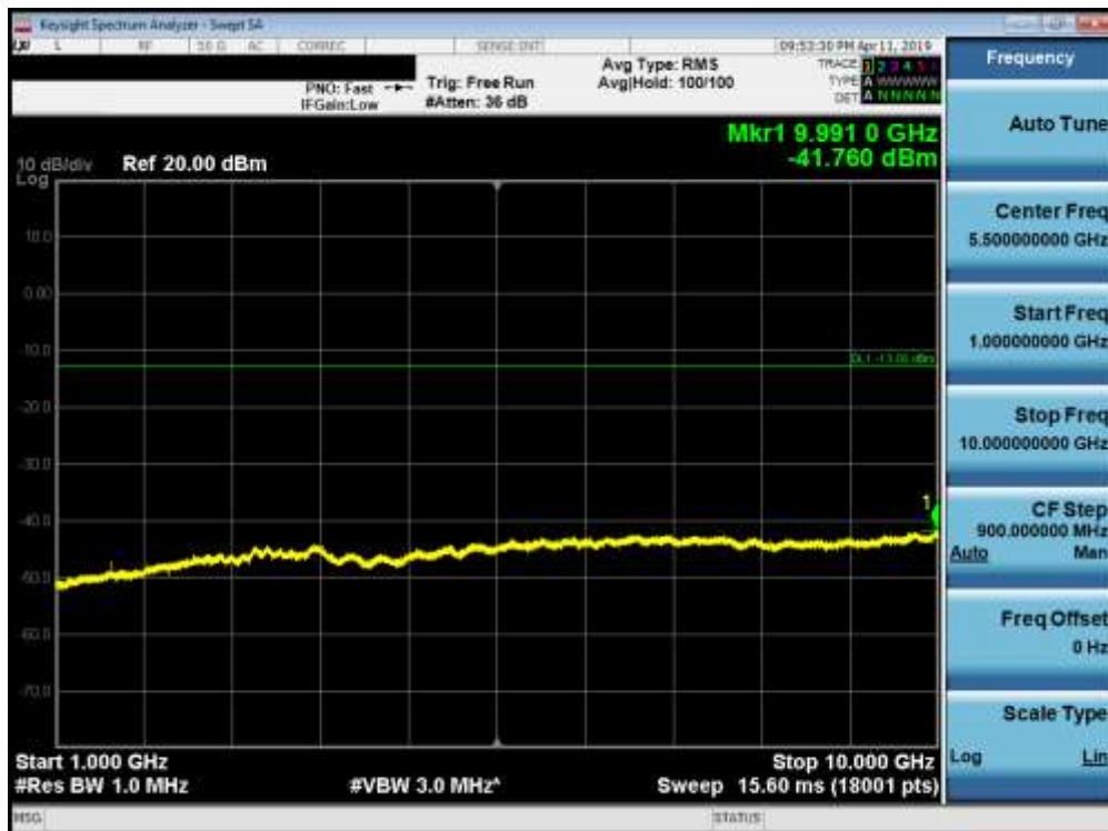
Plot 7-76. Conducted Spurious Plot (Band 13 - 10.0MHz QPSK - RB Size 1, RB Offset 0)
