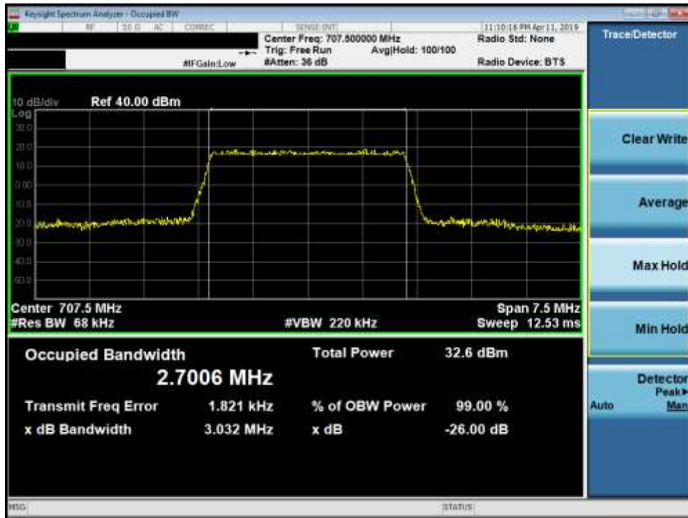
Plot 7-11. Occupied Bandwidth Plot (Band 12 - 3.0MHz QPSK - Full RB Configuration)
