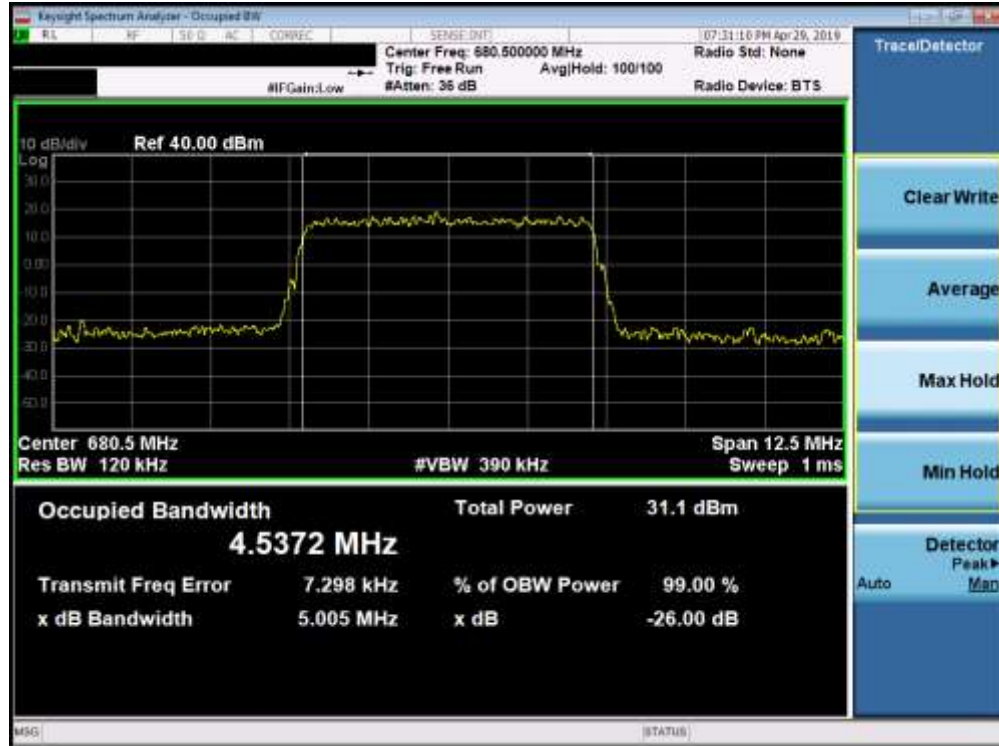
Plot 7-1. Occupied Bandwidth Plot (Band 71 - 5.0MHz QPSK - Full RB Configuration)
