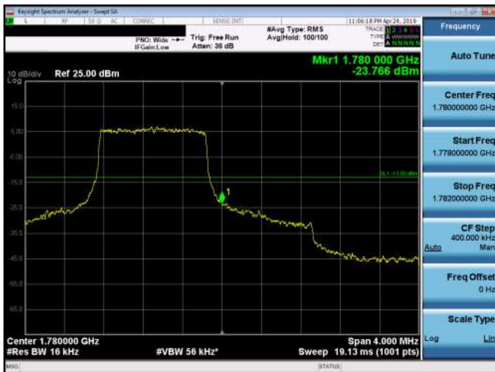
Plot 7-142. Upper Band Edge Plot (Band 66 - 1.4MHz QPSK - Full RB Configuration)
