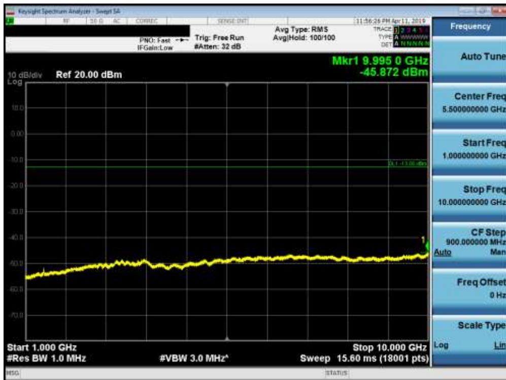
Plot 7-64. Conducted Spurious Plot (Band 12/17 - 10.0MHz QPSK - RB Size 1, RB Offset 0 - Low Channel)
