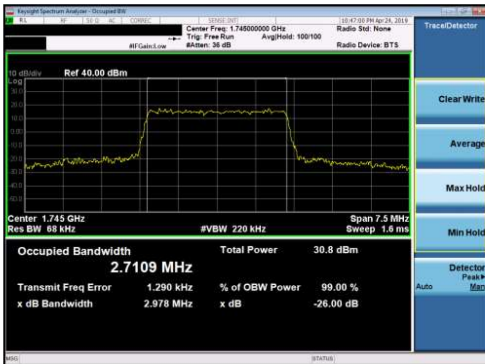
Plot 7-32. Occupied Bandwidth Plot (Band 66/4 - 3.0MHz 16-QAM - Full RB Configuration)
