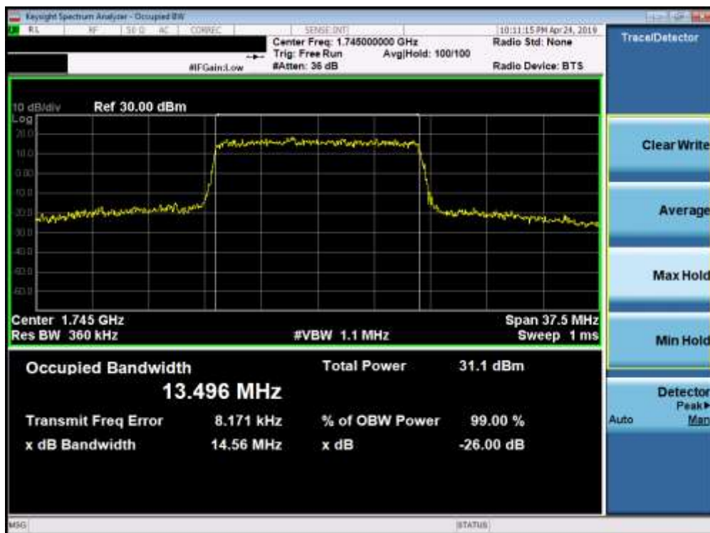
Plot 7-37. Occupied Bandwidth Plot (Band 66/4 - 15.0MHz QPSK - Full RB Configuration)
