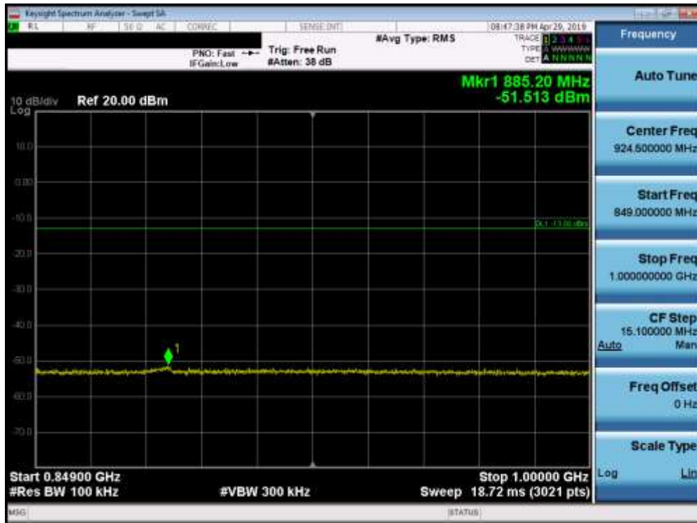
Plot 7-81. Conducted Spurious Plot (Band 5 - 10.0MHz QPSK - RB Size 1, RB Offset 0 - Mid Channel)
