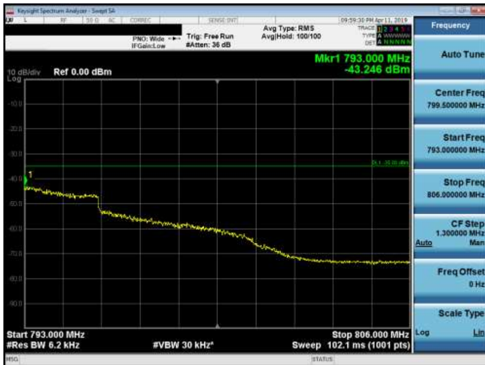
Plot 7-129. Upper Emission Mask Plot (Band 13 - 10.0MHz QPSK - Full RB Configuration)
