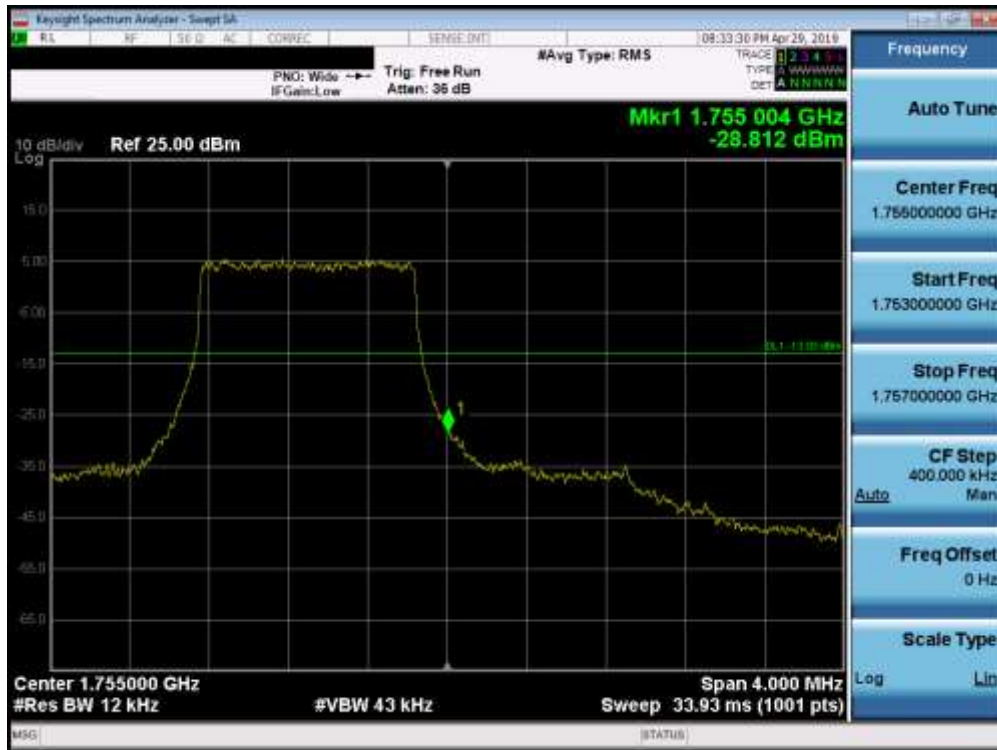
Plot 7-140. Upper Band Edge Plot (Band 4 - 1.4MHz QPSK - Full RB Configuration)
