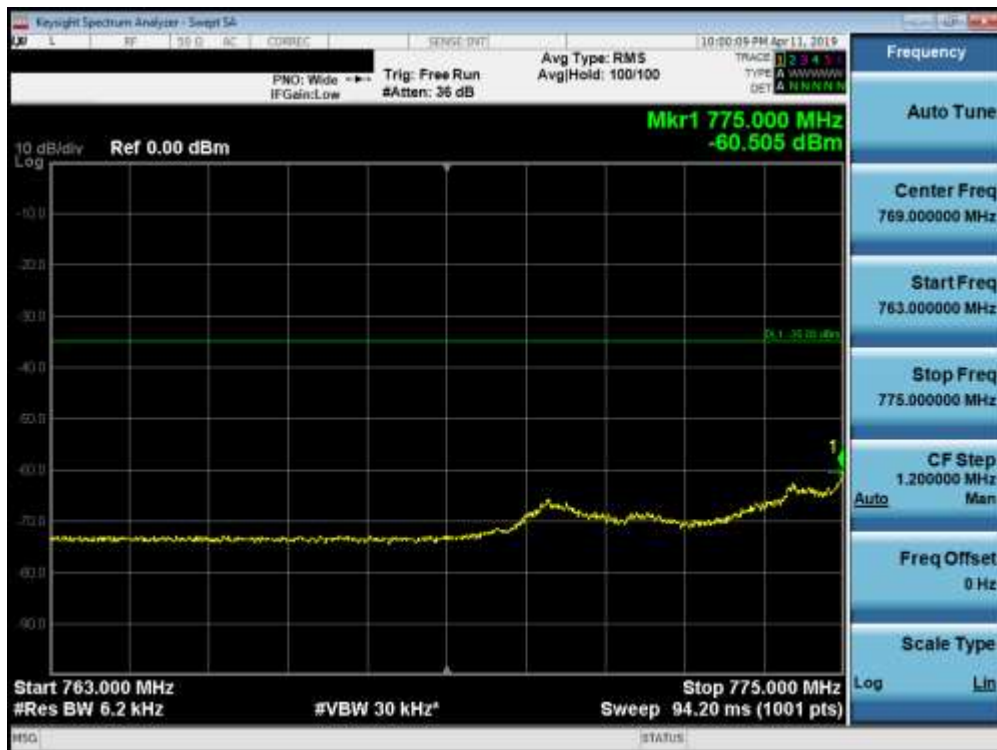
Plot 7-127. Lower Emission Mask Plot (Band 13 - 10.0MHz QPSK - Full RB Configuration)
