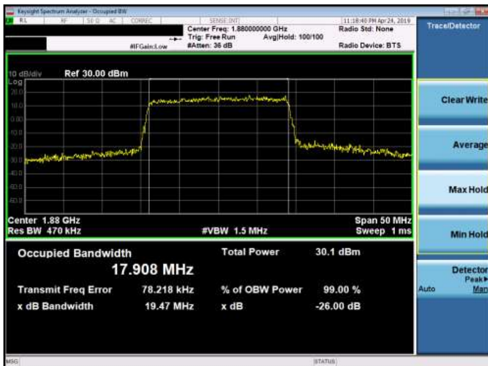
Plot 7-52. Occupied Bandwidth Plot (Band 2 - 20.0MHz 16-QAM - Full RB Configuration)
