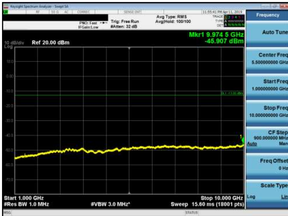
Plot 7-67. Conducted Spurious Plot (Band 12/17 - 10.0MHz QPSK - RB Size 1, RB Offset 0 - Mid Channel)
