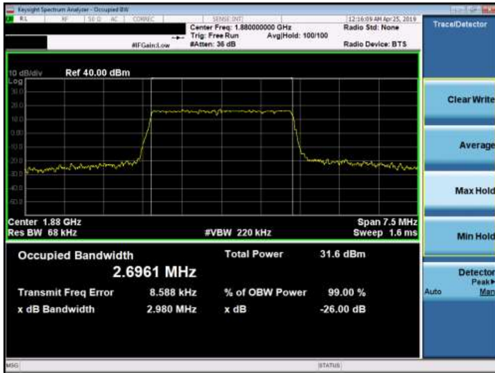
Plot 7-43. Occupied Bandwidth Plot (Band 2 - 3.0MHz QPSK - Full RB Configuration)
