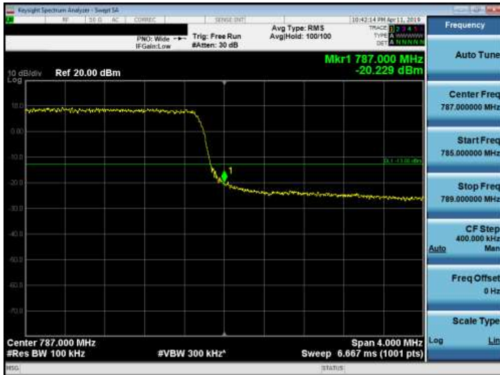
Plot 7-124. Upper Band Edge Plot (Band 13 - 5.0MHz QPSK - Full RB Configuration)
