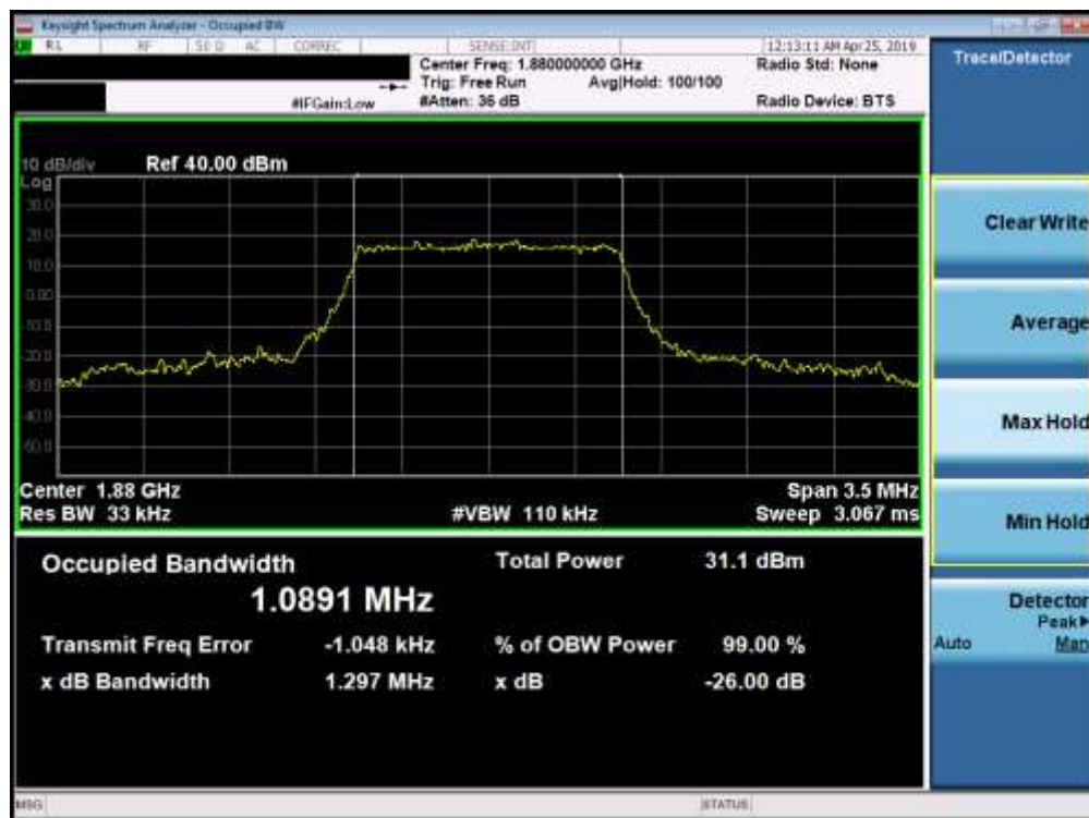
Plot 7-41. Occupied Bandwidth Plot (Band 2 - 1.4MHz QPSK - Full RB Configuration)
