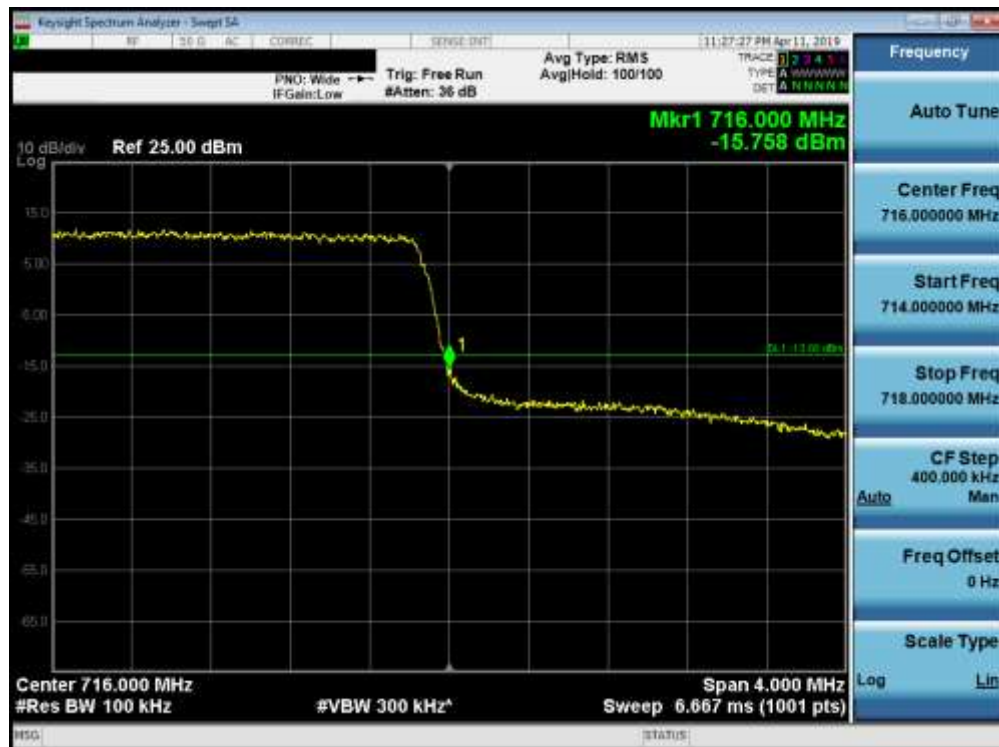
Plot 7-115. Upper Band Edge Plot (Band 12 - 3.0MHz QPSK - Full RB Configuration)
