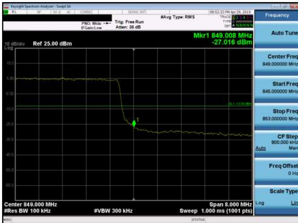
Plot 7-137. Upper Band Edge Plot (Band 5 - 10.0MHz QPSK - Full RB Configuration)
