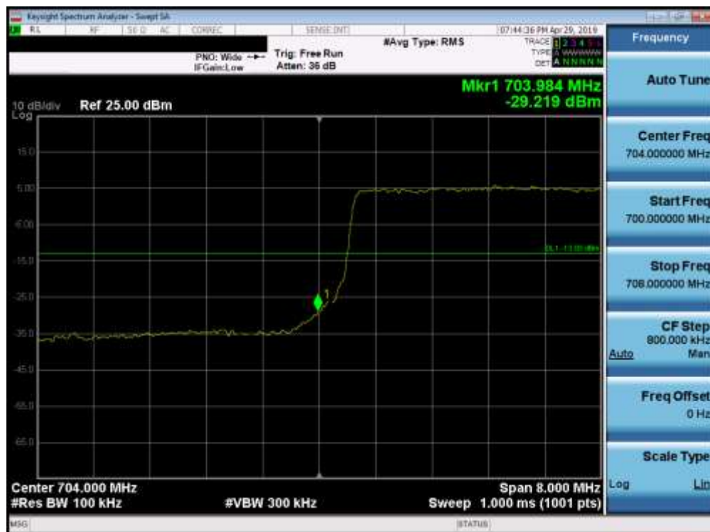
Plot 7-120. Lower Band Edge Plot (Band 17 - 10.0MHz QPSK - Full RB Configuration)
