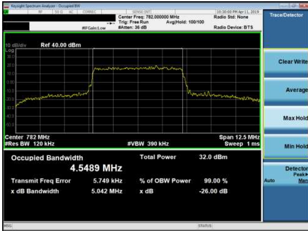
Plot 7-17. Occupied Bandwidth Plot (Band 13 - 5.0MHz QPSK - Full RB Configuration)
