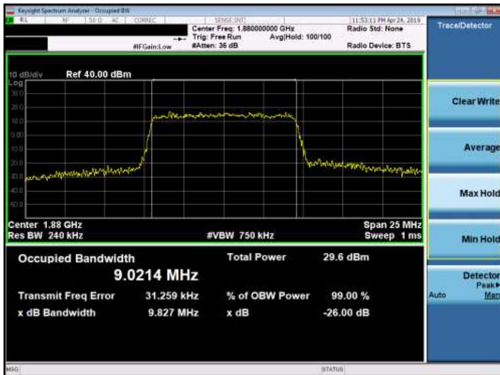
Plot 7-48. Occupied Bandwidth Plot (Band 2 - 10.0MHz 16-QAM - Full RB Configuration)
