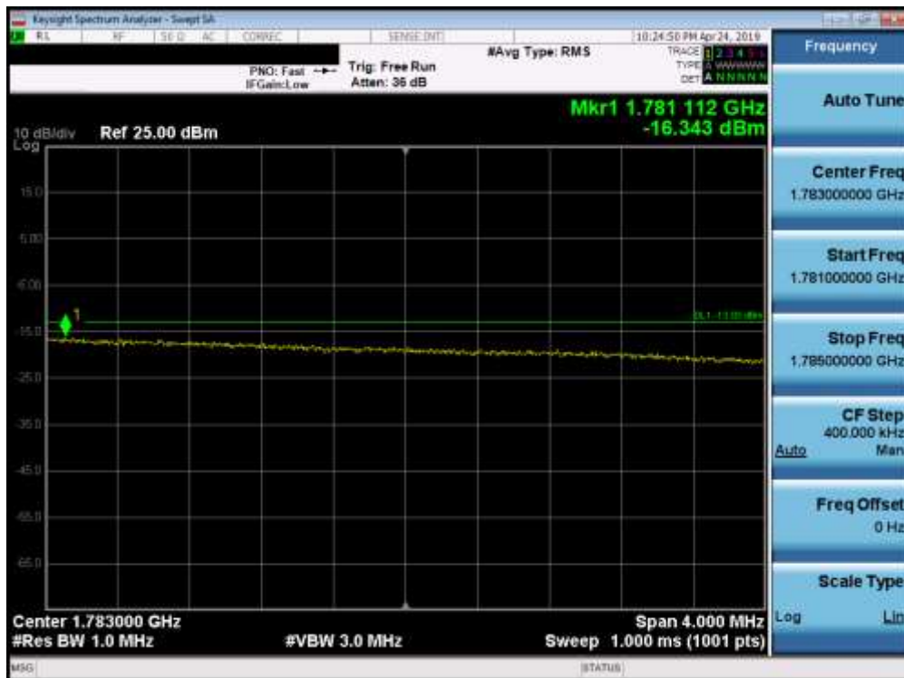
Plot 7-161. Upper Extended Band Edge Plot (Band 66 - 10.0MHz QPSK - Full RB Configuration)
