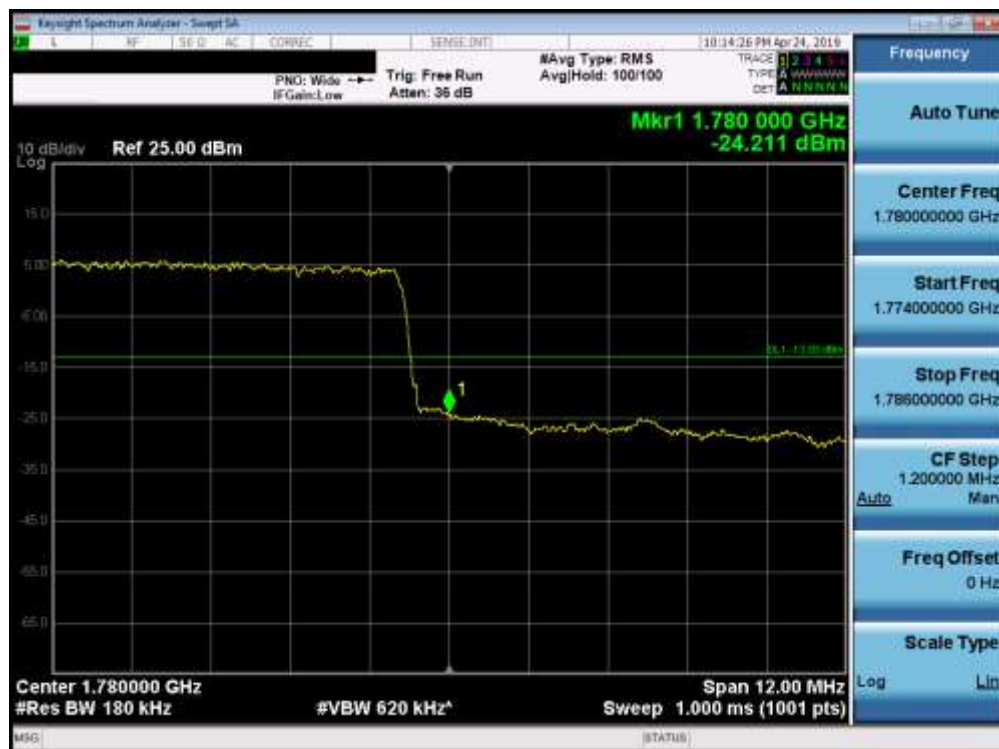
Plot 7-166. Upper Band Edge Plot (Band 66 - 15.0MHz QPSK - Full RB Configuration)
