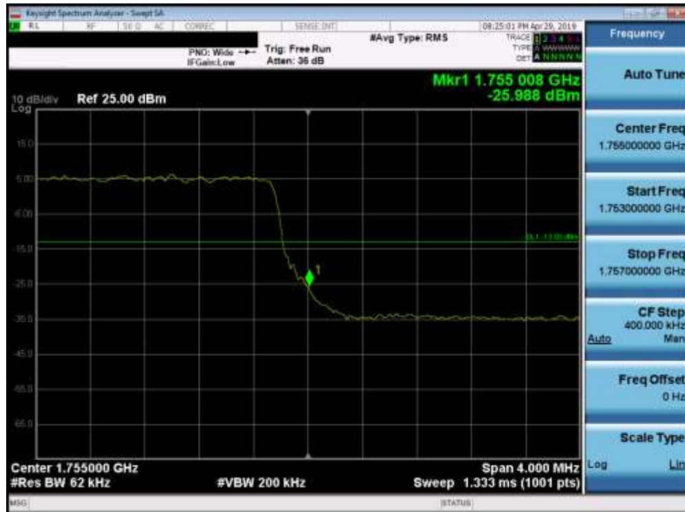
Plot 7-152. Upper Band Edge Plot (Band 4 - 5.0MHz QPSK - Full RB Configuration)
