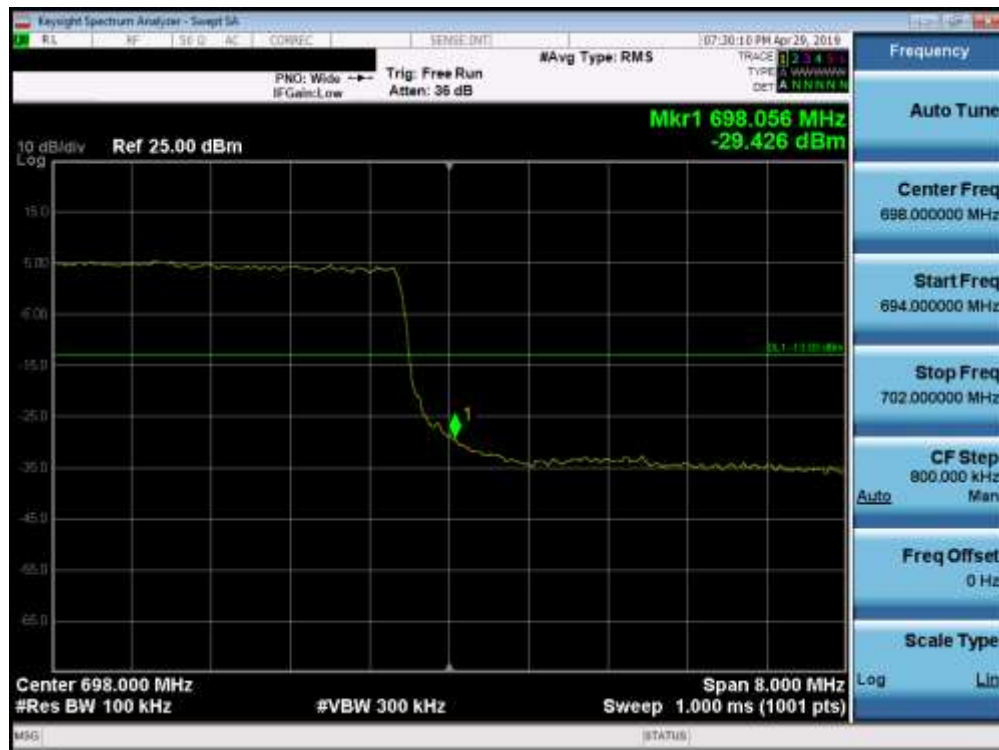
Plot 7-107. Upper Band Edge Plot (Band 71 - 10.0MHz QPSK - Full RB Configuration)
