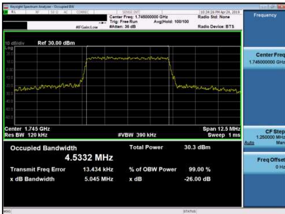
Plot 7-34. Occupied Bandwidth Plot (Band 66/4 - 5.0MHz 16-QAM - Full RB Configuration)
