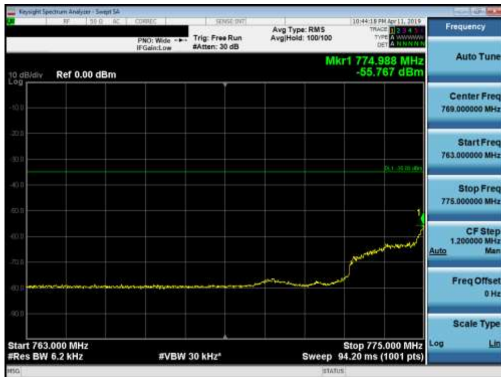
Plot 7-123. Lower Emission Mask Plot (Band 13 - 5.0MHz QPSK - Full RB Configuration)
