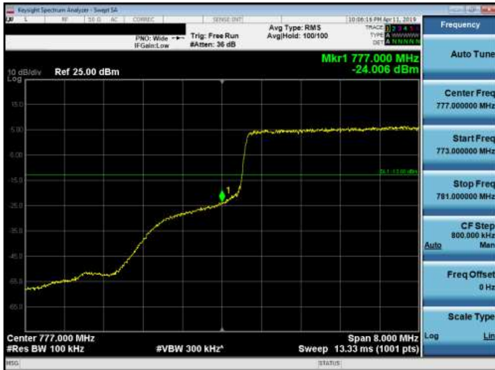
Plot 7-126. Lower Band Edge Plot (Band 13 - 10.0MHz QPSK - Full RB Configuration)
