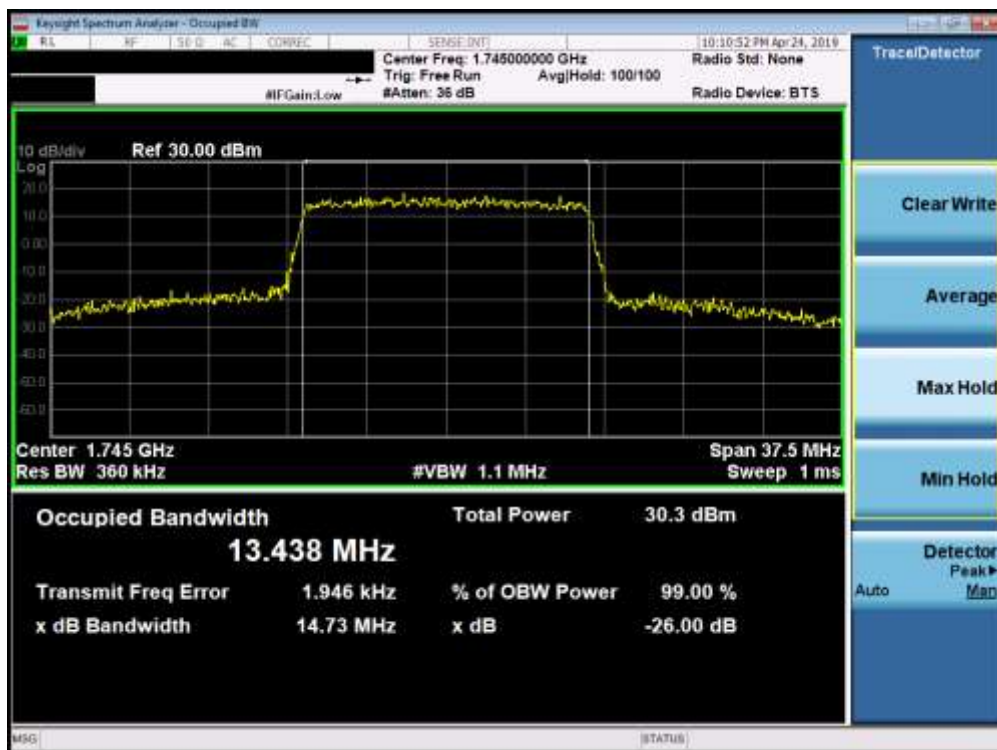
Plot 7-38. Occupied Bandwidth Plot (Band 66/4 - 15.0MHz 16-QAM - Full RB Configuration)
