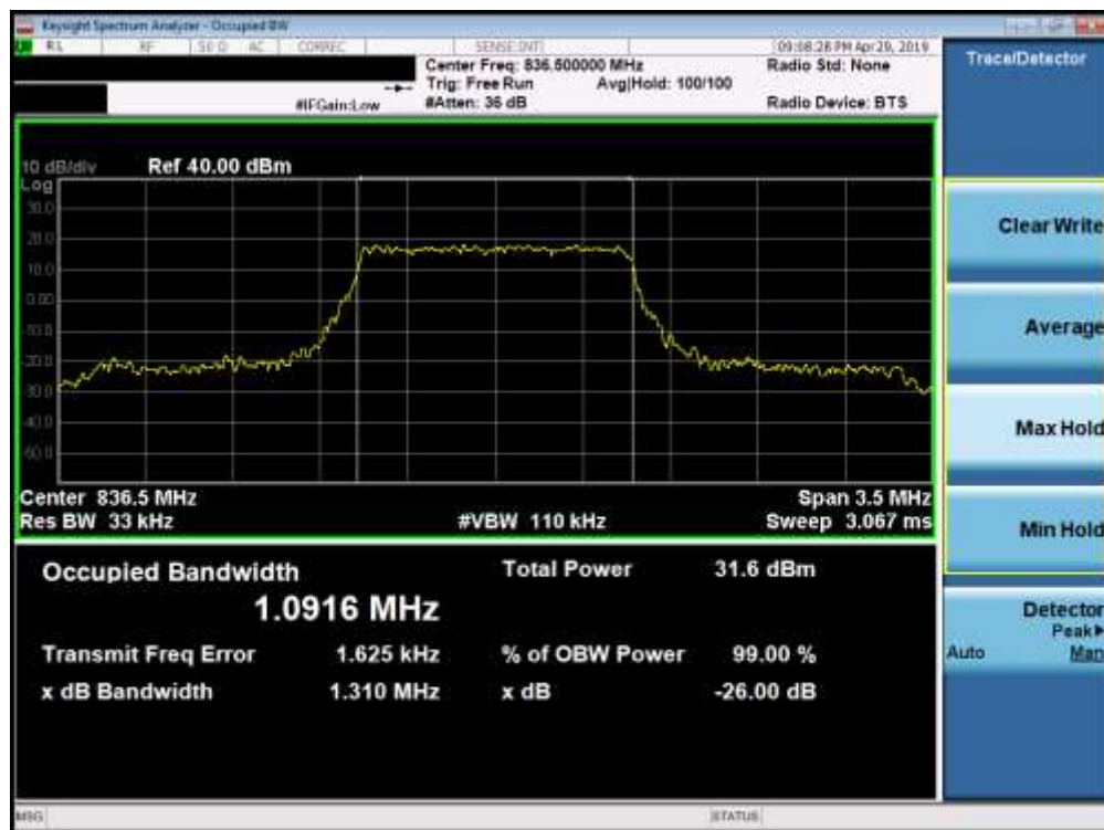
Plot 7-21. Occupied Bandwidth Plot (Band 5 - 1.4MHz QPSK - Full RB Configuration)
