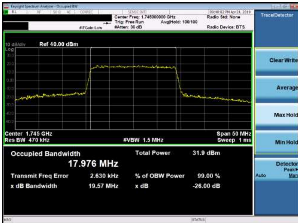
Plot 7-40. Occupied Bandwidth Plot (Band 66/4 - 20.0MHz 16-QAM - Full RB Configuration)
