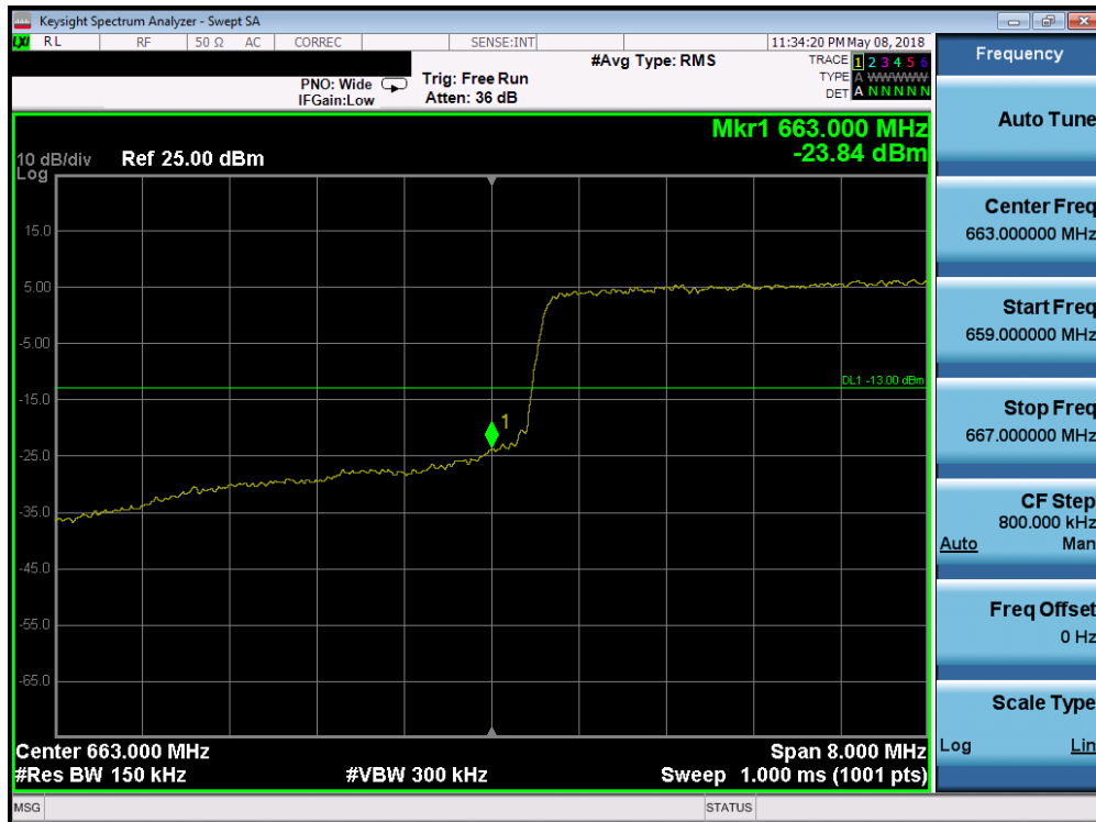
Plot 7-96. Lower Band Edge Plot (Band 71 - 10.0MHz QPSK - Full RB Configuration)
