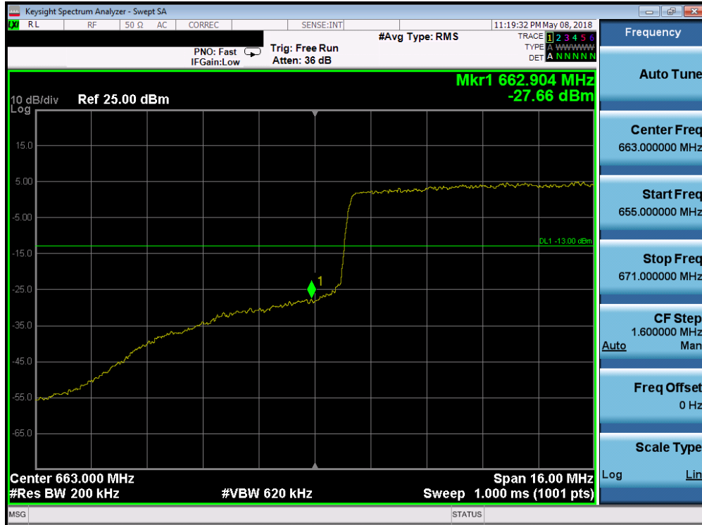
Plot 7-100. Lower Band Edge Plot (Band 71 - 20.0MHz QPSK - Full RB Configuration)
