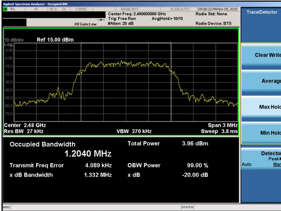
Plot 7-6. 20dB Bandwidth Plot (Bluetooth, 2Mbps – Ch. 78)
