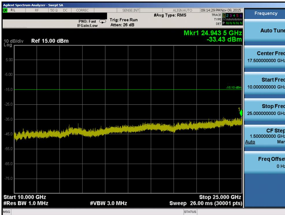
Plot 7-37. Conducted Spurious Plot (Bluetooth, 3Mbps – Ch. 0)
