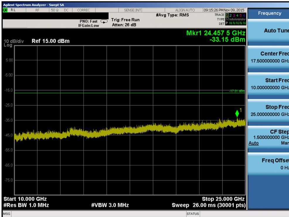
Plot 7-39. Conducted Spurious Plot (Bluetooth, 3Mbps – Ch. 39)
