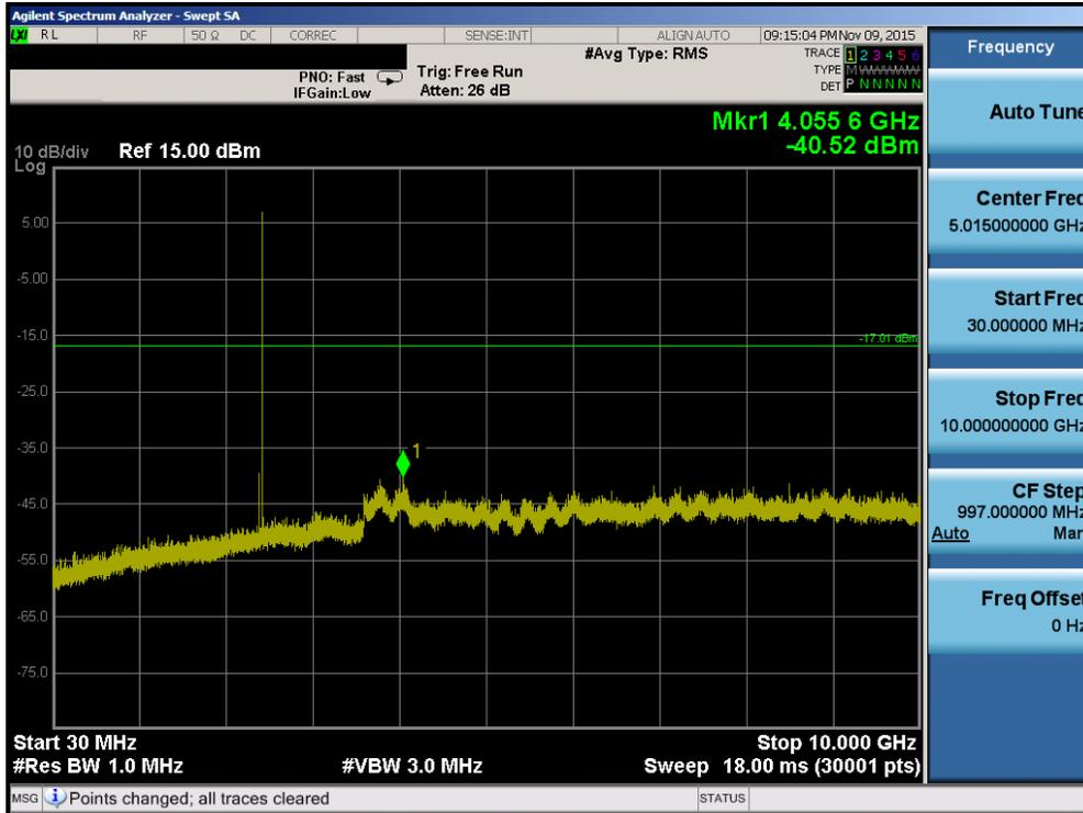
Plot 7-38. Conducted Spurious Plot (Bluetooth, 3Mbps – Ch. 39)
