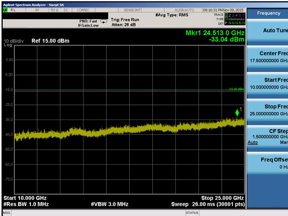
Plot 7-41. Conducted Spurious Plot (Bluetooth, 3Mbps – Ch. 78)
