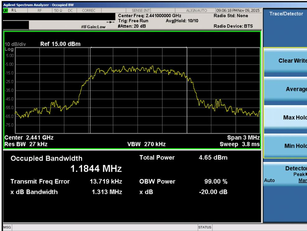
Plot 7-5. 20dB Bandwidth Plot (Bluetooth, 2Mbps – Ch. 39)
