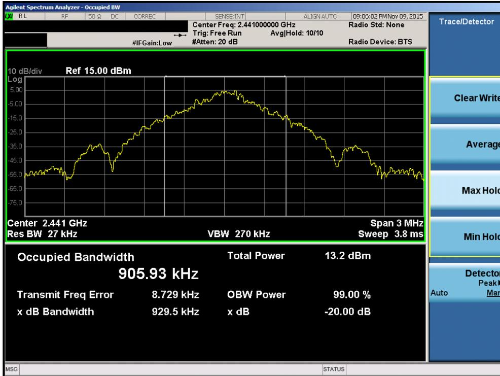
Plot 7-2. 20dB Bandwidth Plot (Bluetooth, 1Mbps – Ch. 39)
