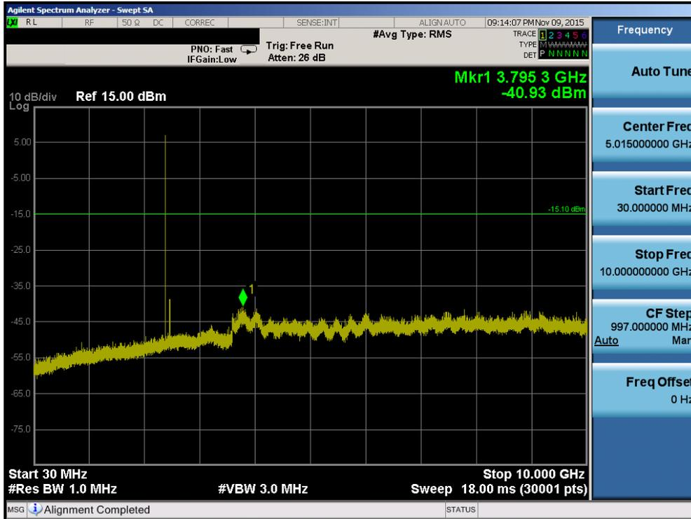
Plot 7-36. Conducted Spurious Plot (Bluetooth, 3Mbps – Ch. 0)
