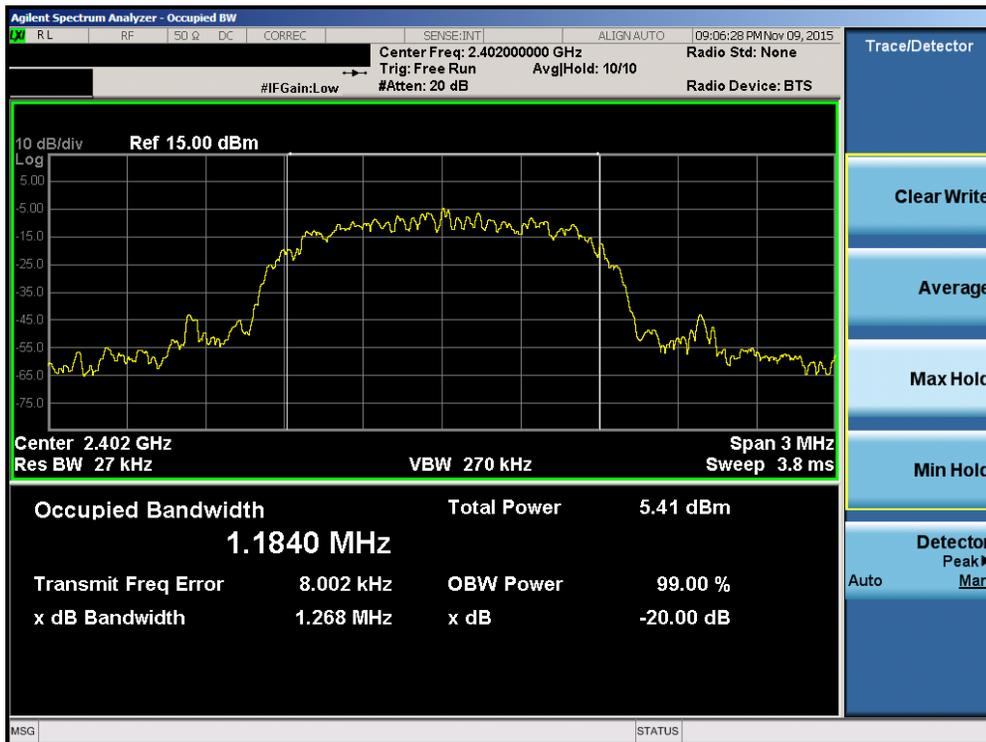
Plot 7-7. 20dB Bandwidth Plot (Bluetooth, 3Mbps – Ch. 0)
