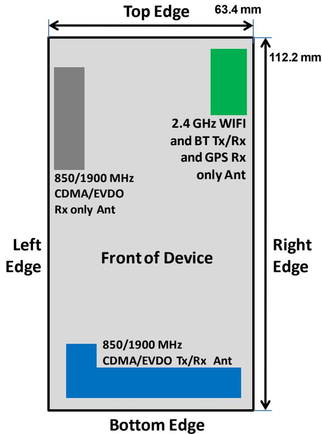
Note: Exact antenna dimensions and separation distances are shown in the Technical Descriptions in the FCC Filing.
