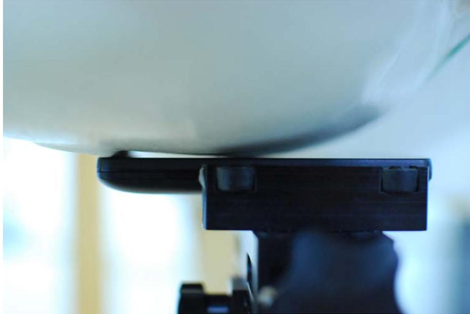
**SAR Test Setup Photo 1 – Right Cheek**
