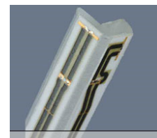
Figure 5-1 E-field Free-space Probe
