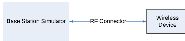
Figure 9-3 Power Measurement Setup
