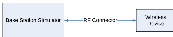
Figure 9-1 Power Measurement Setup
