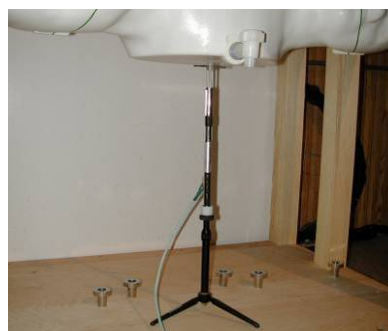
Figure 10-2 System Verification Setup Photo
