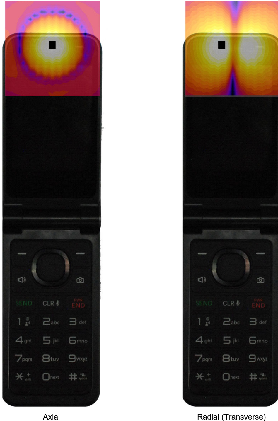
Axial Radial (Transverse) Figure 15-3 T-Coil Scan Overlay Magnetic Field Distributions
