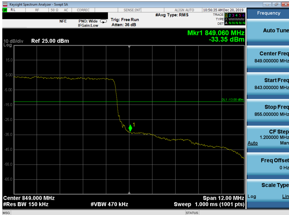
Plot 7-128. Upper Band Edge Plot (Band 26 - 15.0MHz QPSK - Full RB Configuration)
