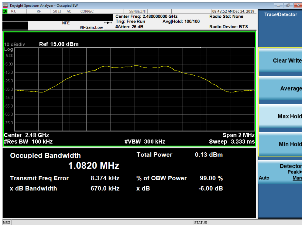
Plot 7-3. 6dB Bandwidth Plot (Bluetooth (LE), – Ch. 39)
