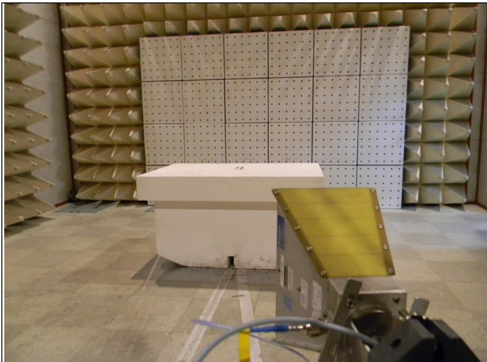
***C. Photo of Field Strength & Spurious Emission Test for NFC***
