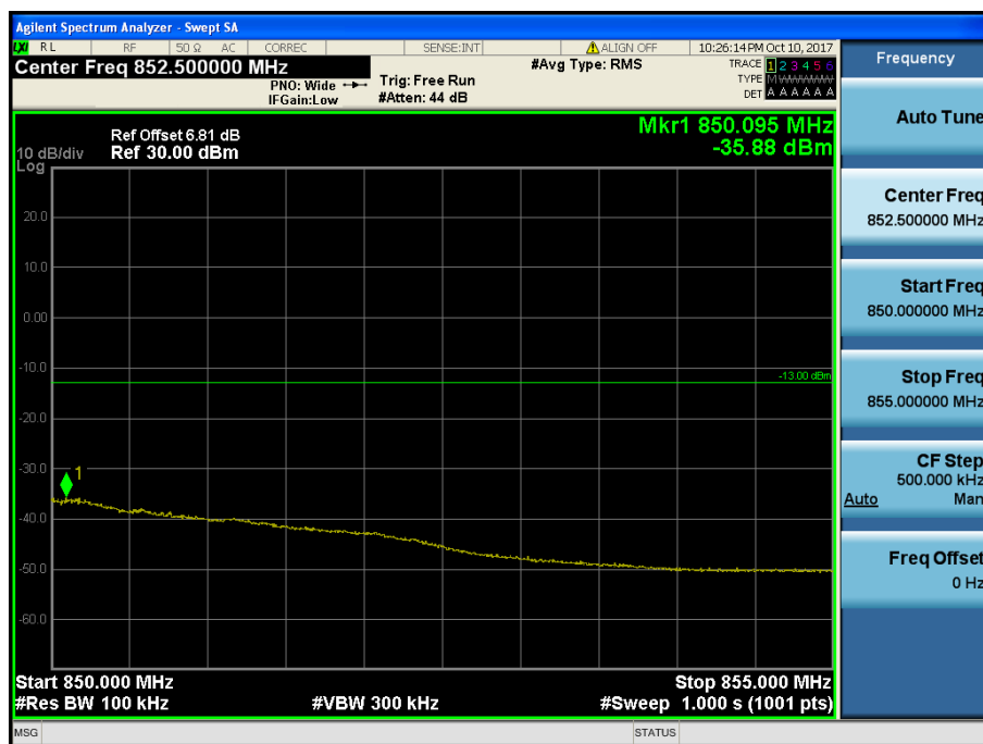
LTE Band 5 / 5MHz / QPSK - RB Size/Offset (12/13)
