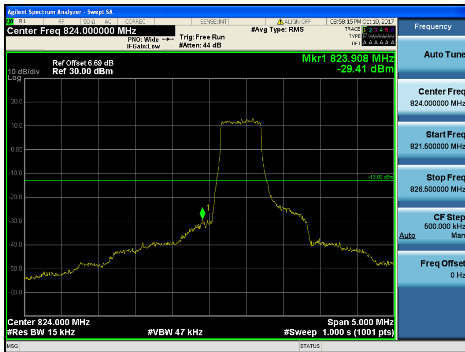
LTE Band 5 / 1.4MHz / QPSK - RB Size/Offset (3/0)
