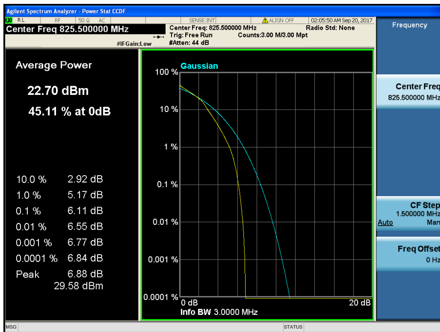
LTE Band 5 / 3 MHz / 16QAM - RB Size 15
