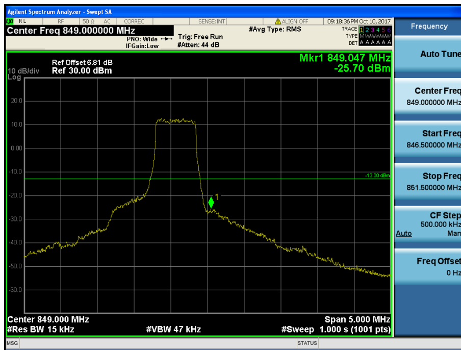
LTE Band 5 / 1.4MHz / QPSK - RB Size/Offset (3/3)
