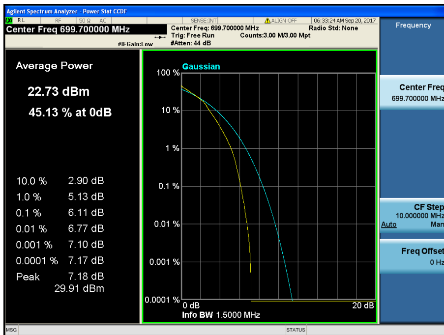
LTE Band 12 / 1.4 MHz / 16QAM - RB Size 6
