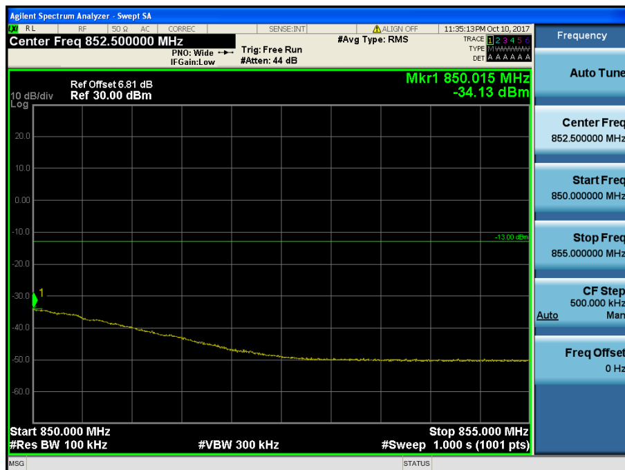
LTE Band 5 / 1.4MHz / 16QAM - RB Size/Offset (6/0)
