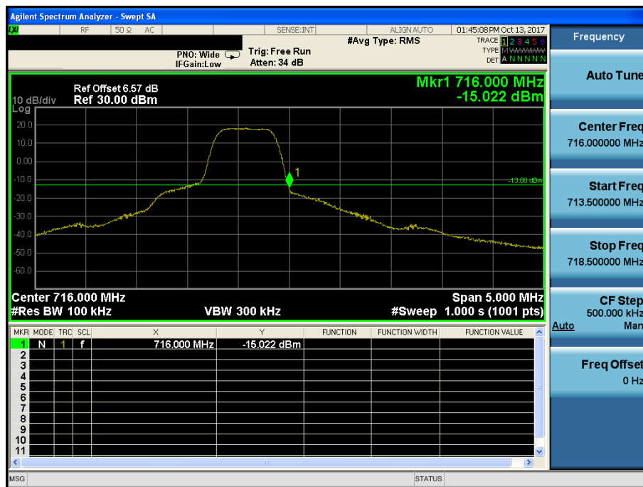
LTE Band 12 / 1.4MHz / QPSK - RB Size/Offset (3/3)
