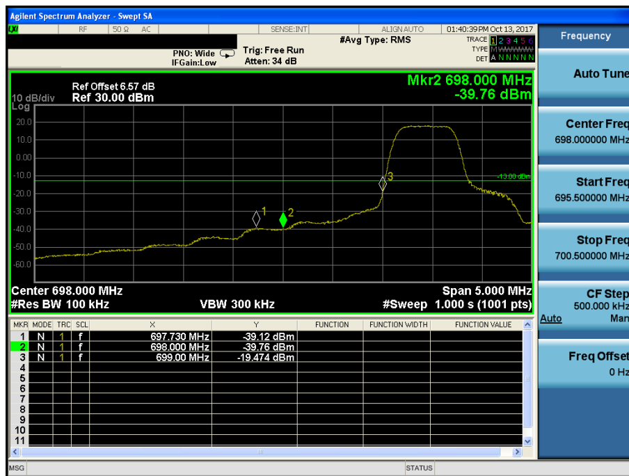
LTE Band 12 / 1.4MHz / QPSK - RB Size/Offset (3/0)
