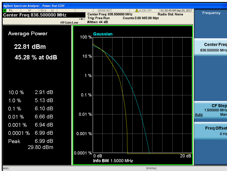
LTE Band 5 / 1.4 MHz / 16QAM - RB Size 6
