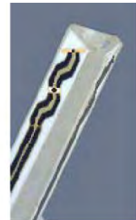
Figure 3.3 Probe Thick-Film Technique
