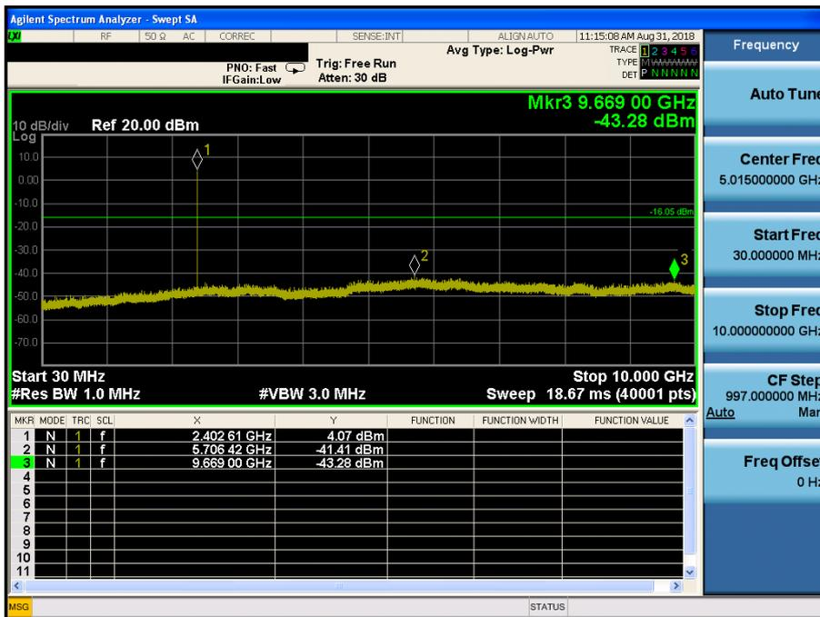
TM 2 Conducted Spurious Emissions 3 (Test Channel : Lowest)
