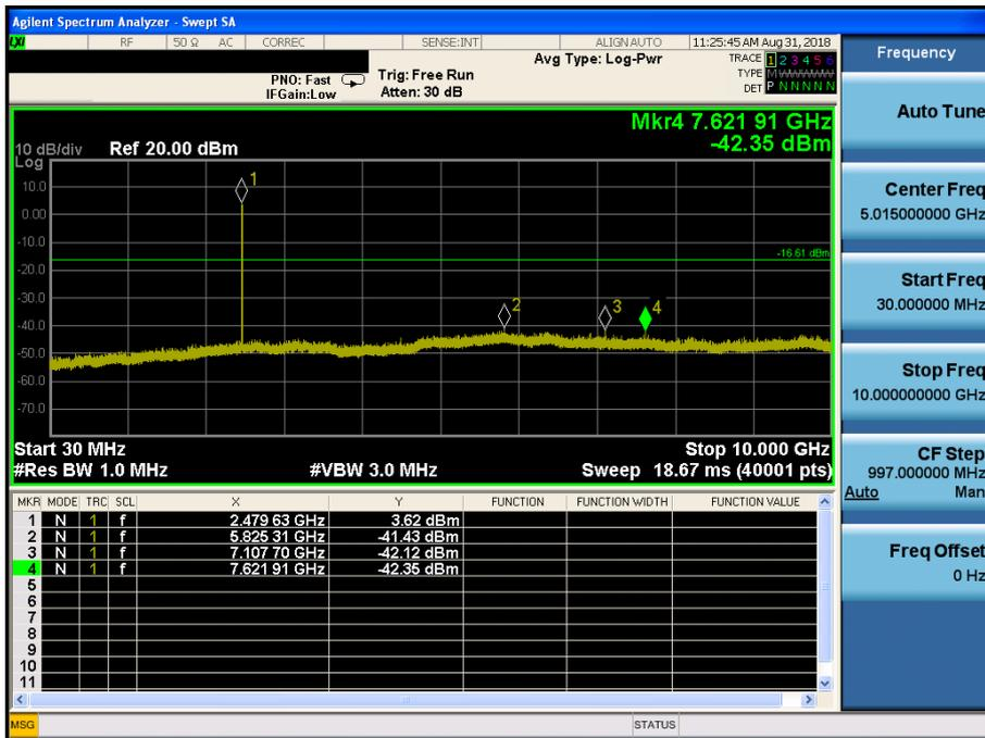
TM 2 Conducted Spurious Emissions 3 (Test Channel : Highest)
