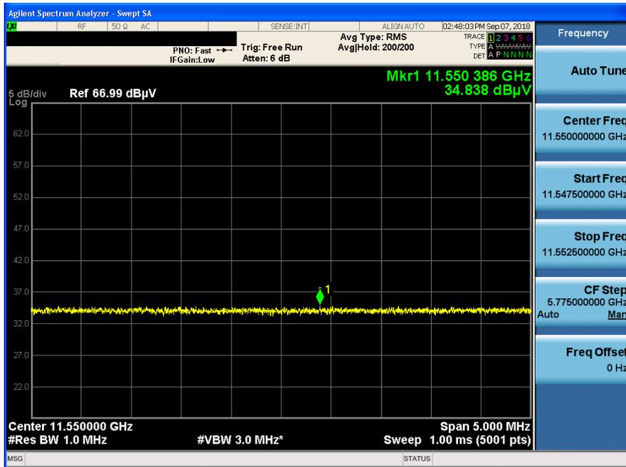
Unwanted Emissions (Radiated) Test Plot : SDM
