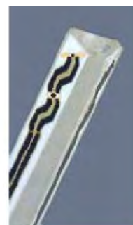
Figure F.2.2 Probe Thick-Film Technique
