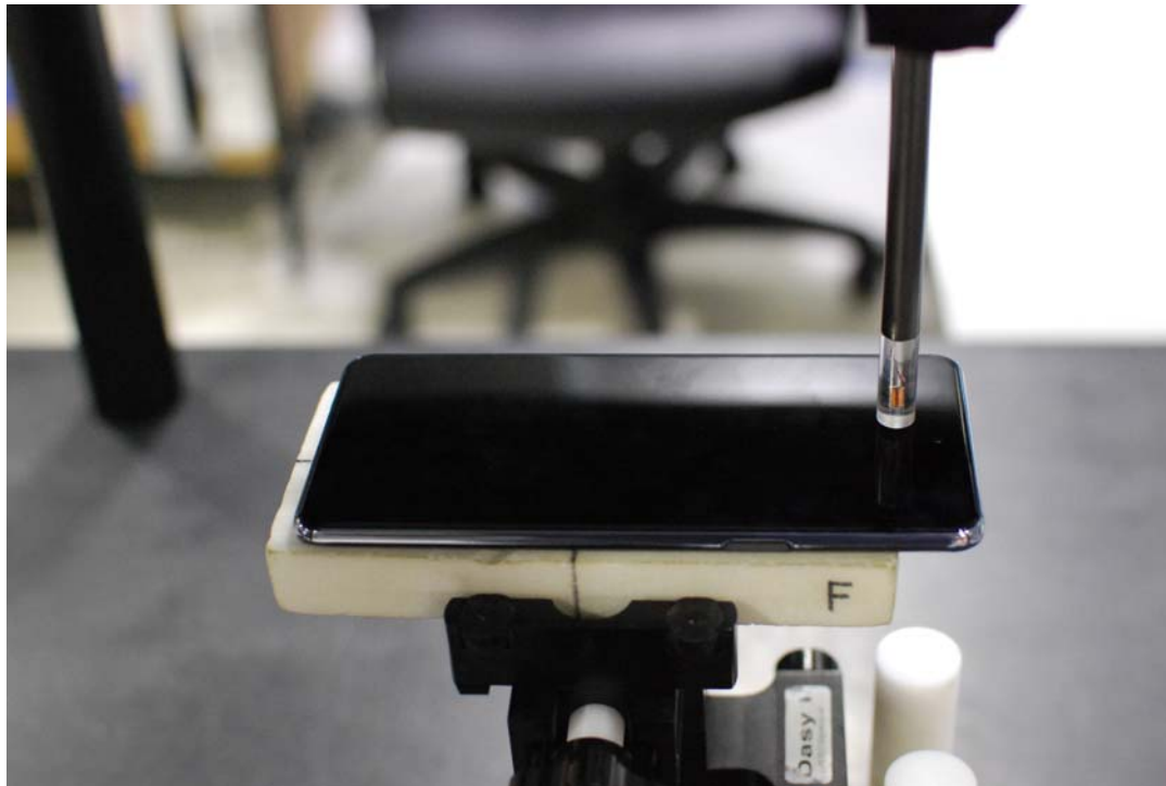
Figure 16-1 Test Setup for Wireless Device
