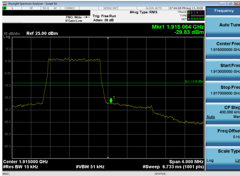
Plot 7-382. Upper Band Edge Plot (LTE Band 25 – 1.4MHz QPSK – Full RB Configuration)
