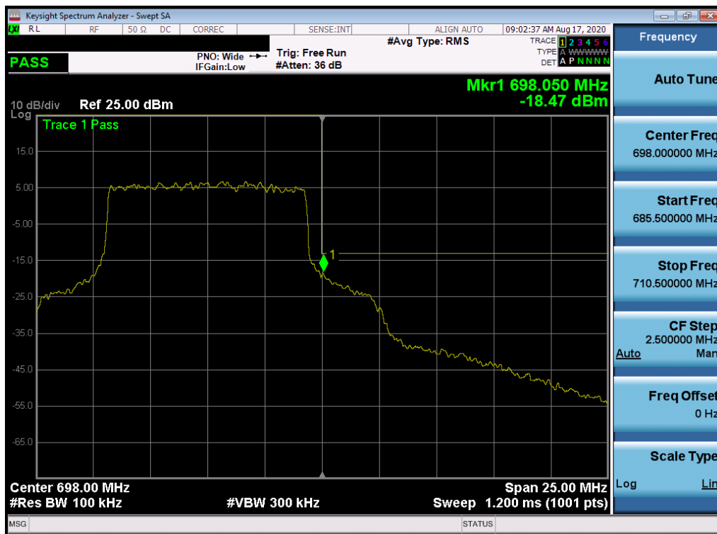
Plot 7-437. Upper Band Edge Plot (NR Band n71 - 10.0MHz - Full RB)
