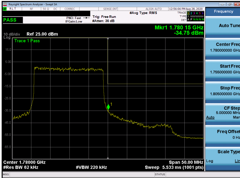
Plot 7-464. Upper Band Edge Plot (NR Band n66 – 20.0MHz - Full RB)
