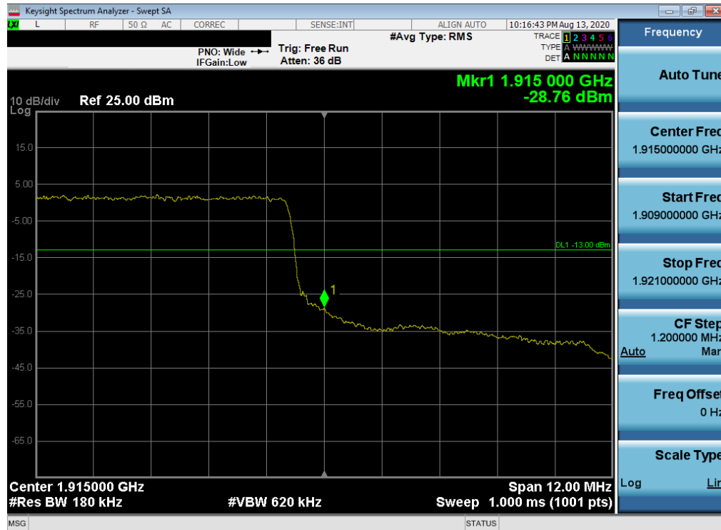
Plot 7-406. Upper Band Edge Plot (LTE Band 25 - 15MHz QPSK – Full RB Configuration)
