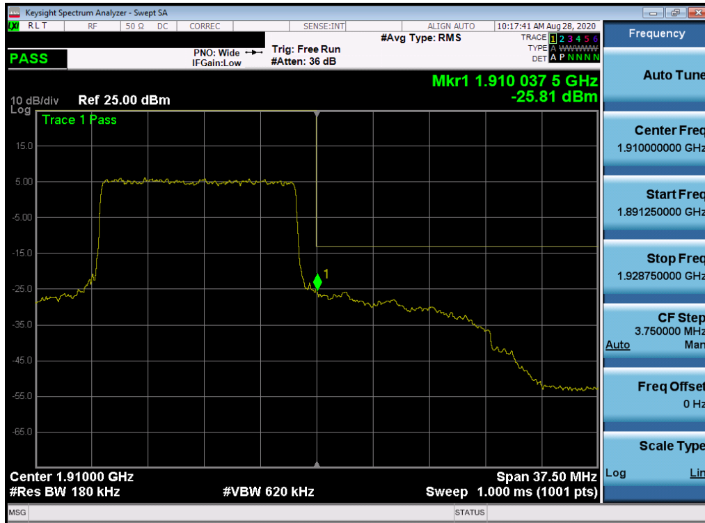
Plot 7-476. Upper Band Edge Plot (NR Band n2 - 15.0MHz - Full RB)
