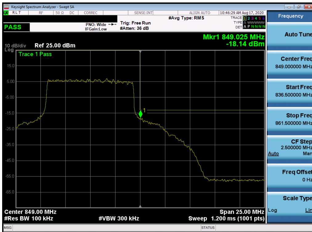
Plot 7-445. Upper Band Edge Plot (NR Band n5 - 10.0MHz - Full RB)
