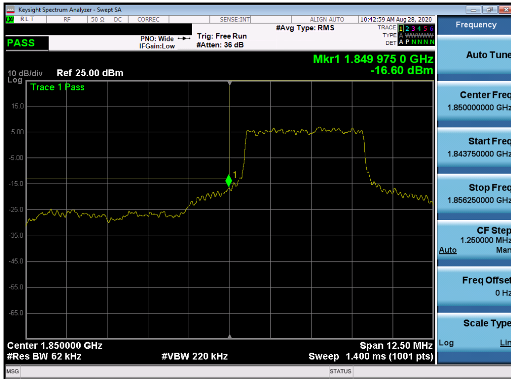
Plot 7-466. Lower Band Edge Plot (NR Band n2 – 5.0MHz - Full RB)
