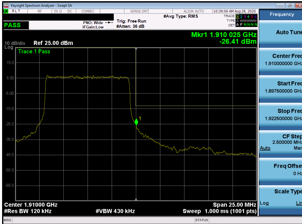
Plot 7-472. Upper Band Edge Plot (NR Band n2 – 10.0MHz - Full RB)
