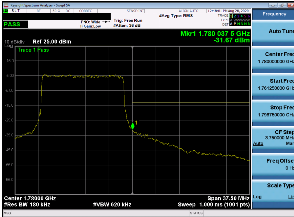
Plot 7-460. Upper Band Edge Plot (NR Band n66 – 15.0MHz - Full RB)
