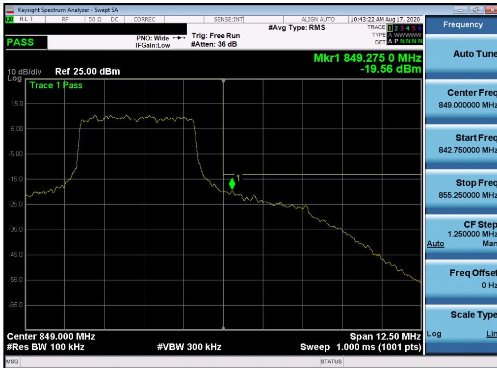
Plot 7-443. Upper Band Edge Plot (NR Band n5 – 5.0MHz - Full RB)
