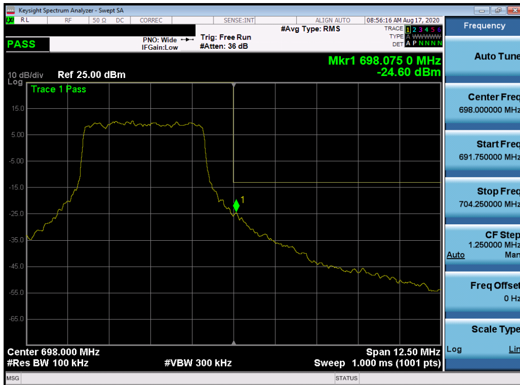
Plot 7-435. Upper Band Edge Plot (NR Band n71 – 5.0MHz - Full RB)
