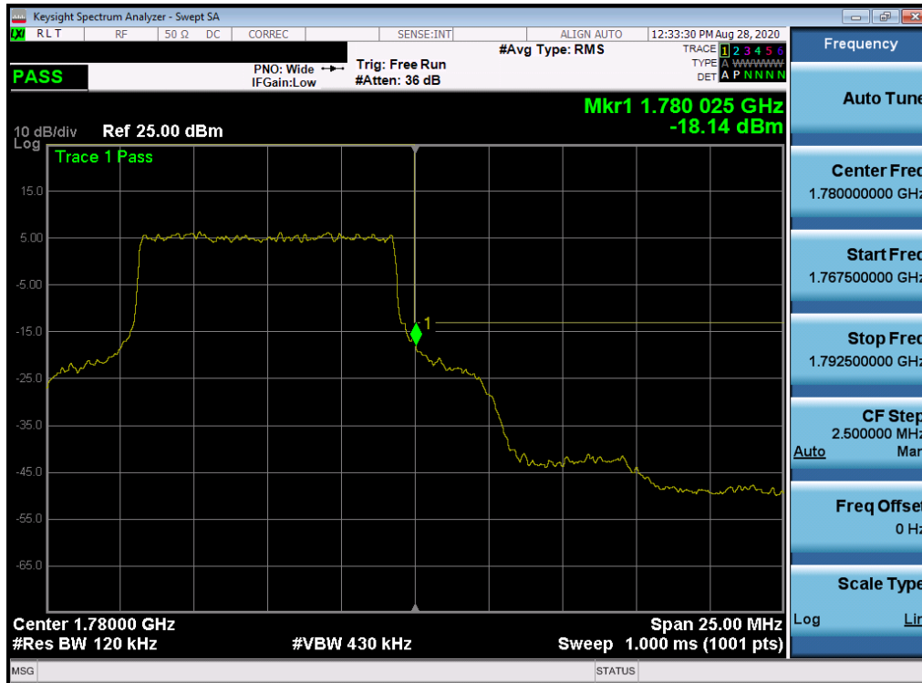
Plot 7-456. Upper Band Edge Plot (NR Band n66 – 10.0MHz - Full RB)
