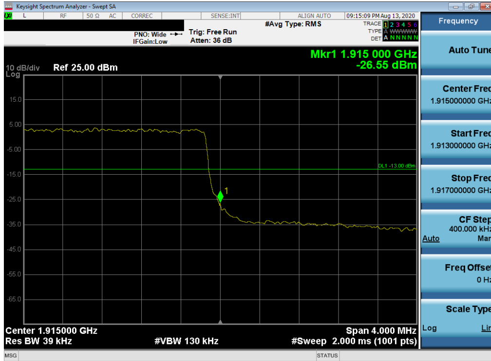
Plot 7-388. Upper Band Edge Plot (LTE Band 25 - 3MHz QPSK – Full RB Configuration)
