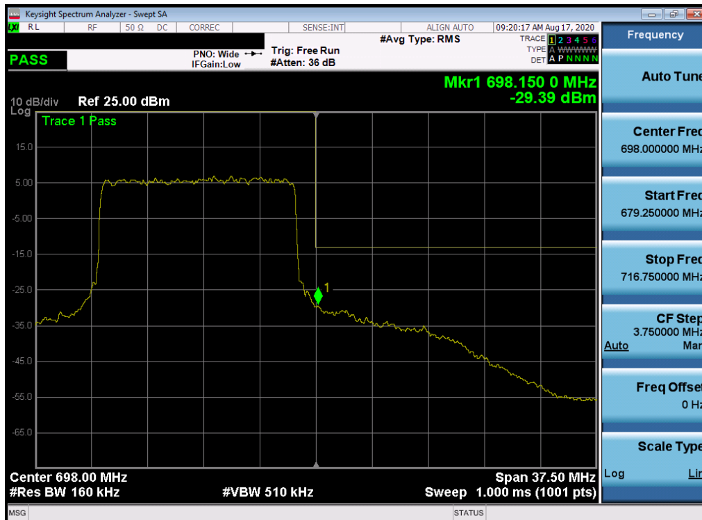
Plot 7-439. Upper Band Edge Plot (NR Band n71 – 15.0MHz - Full RB)
