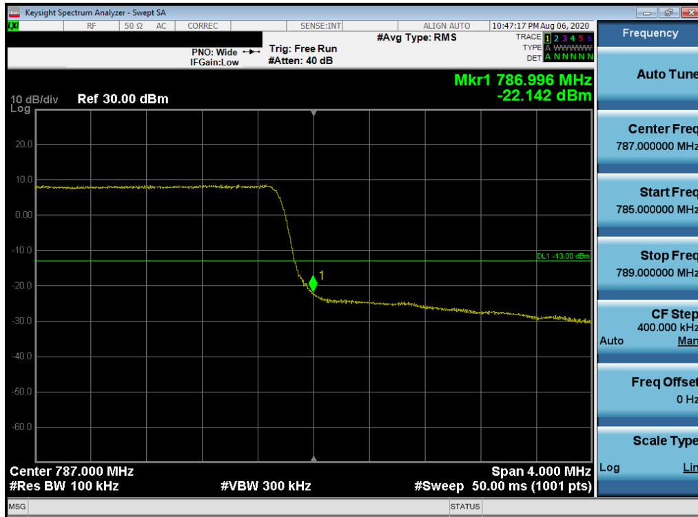
Plot 7-318. Upper Band Edge Plot (LTE Band 13 - 5MHz QPSK – Full RB Configuration)
