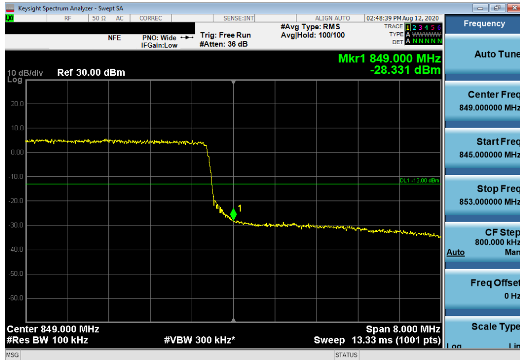
Plot 7-339. Upper Band Edge Plot (LTE Band 26/5 - 10MHz QPSK – Full RB Configuration)
