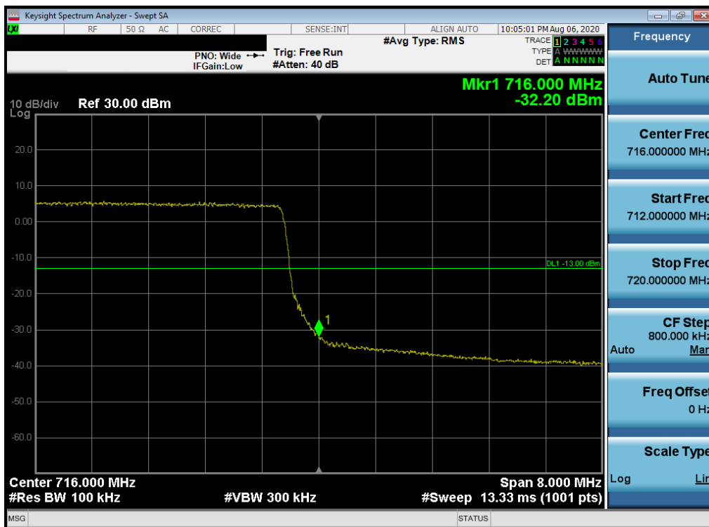
Plot 7-315. Upper Band Edge Plot (LTE Band 12/17 - 10MHz QPSK – Full RB Configuration)
