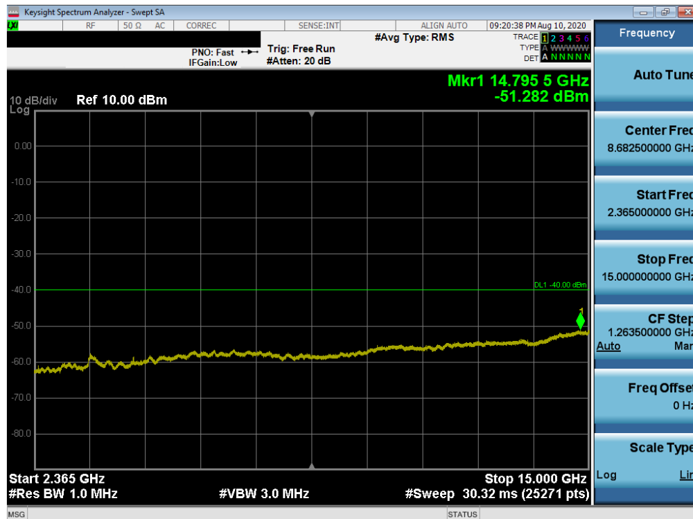
Plot 7-247. Conducted Spurious Plot (LTE Band 30 - 5MHz QPSK - RB Size 1, RB Offset 0 - High Channel)
