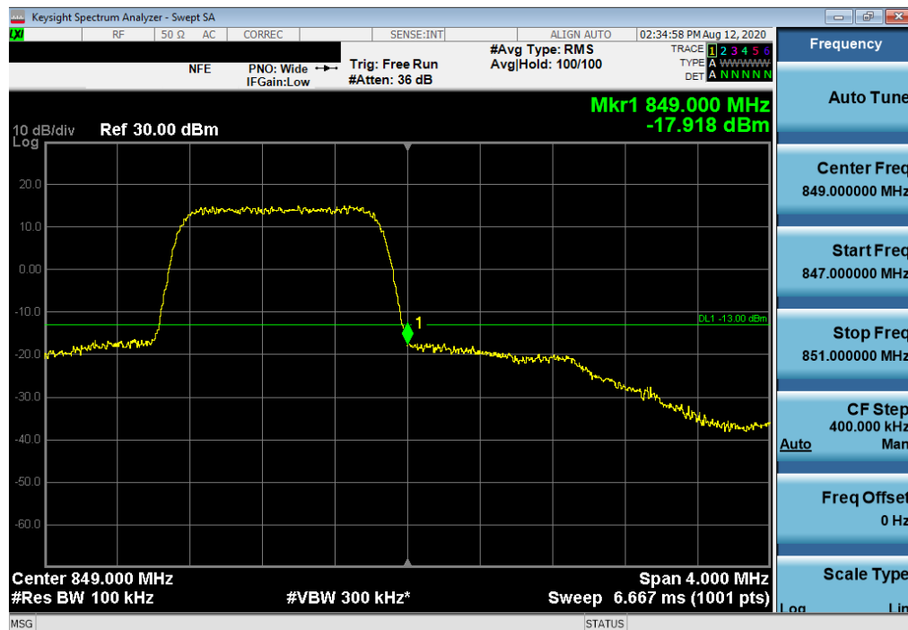
Plot 7-333. Upper Band Edge Plot (LTE Band 26/5 – 1.4MHz QPSK – Full RB Configuration)
