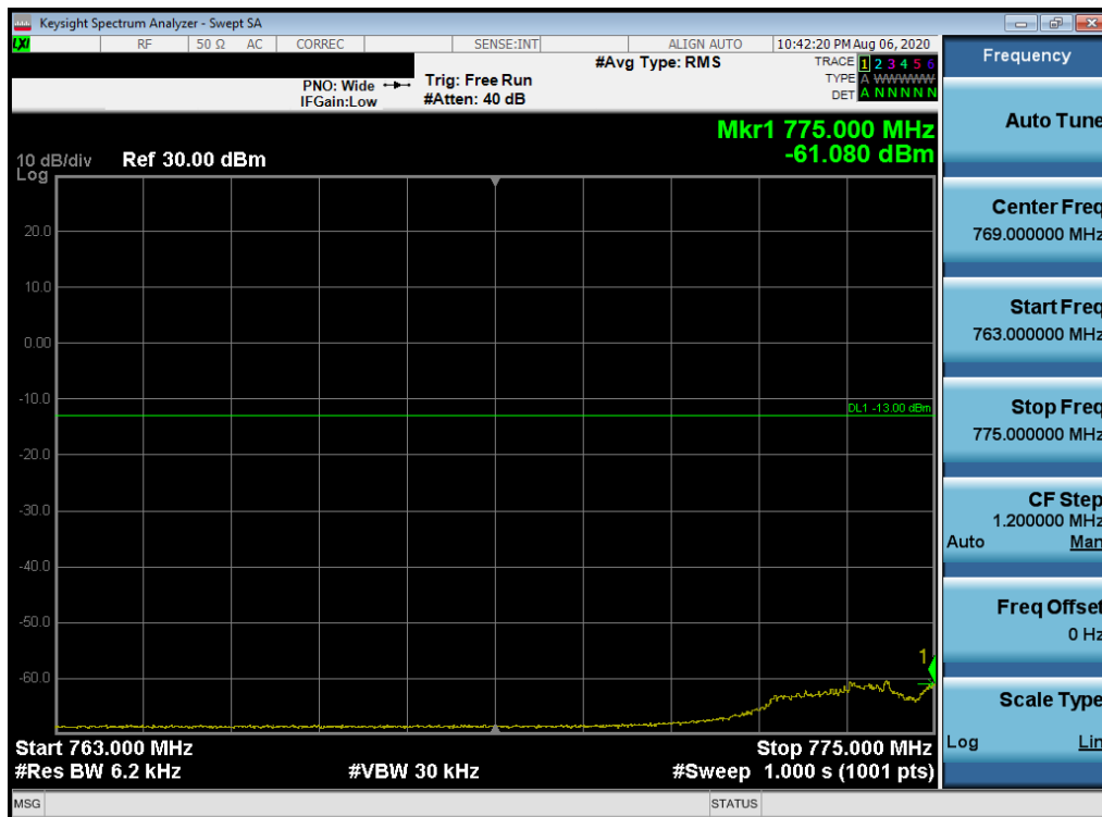
Plot 7-317. Lower Emission Mask Plot (LTE Band 13 - 5MHz QPSK – Full RB Configuration)
