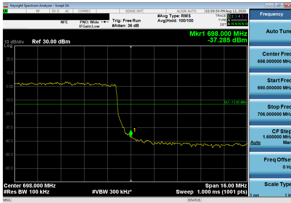
Plot 7-331. Upper Band Edge Plot (LTE Band 71 - 20MHz QPSK – Full RB Configuration)
