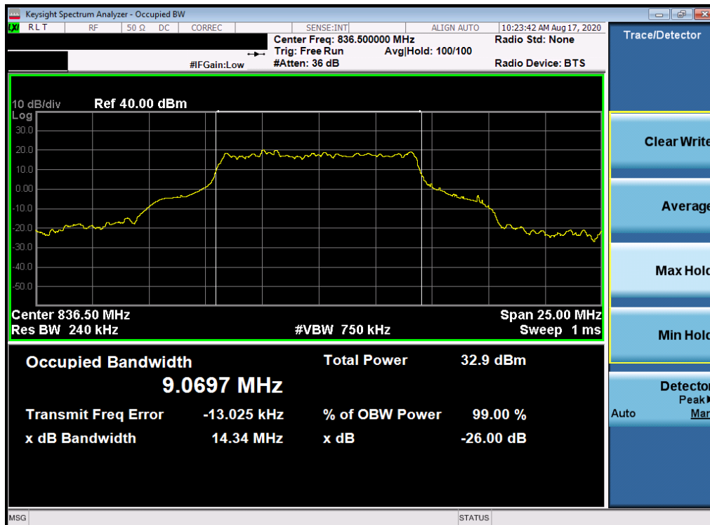
Plot 7-125. Occupied Bandwidth Plot (NR Band n5 - 10.0MHz DFT-s-OFDM BPSK - Full RB)
