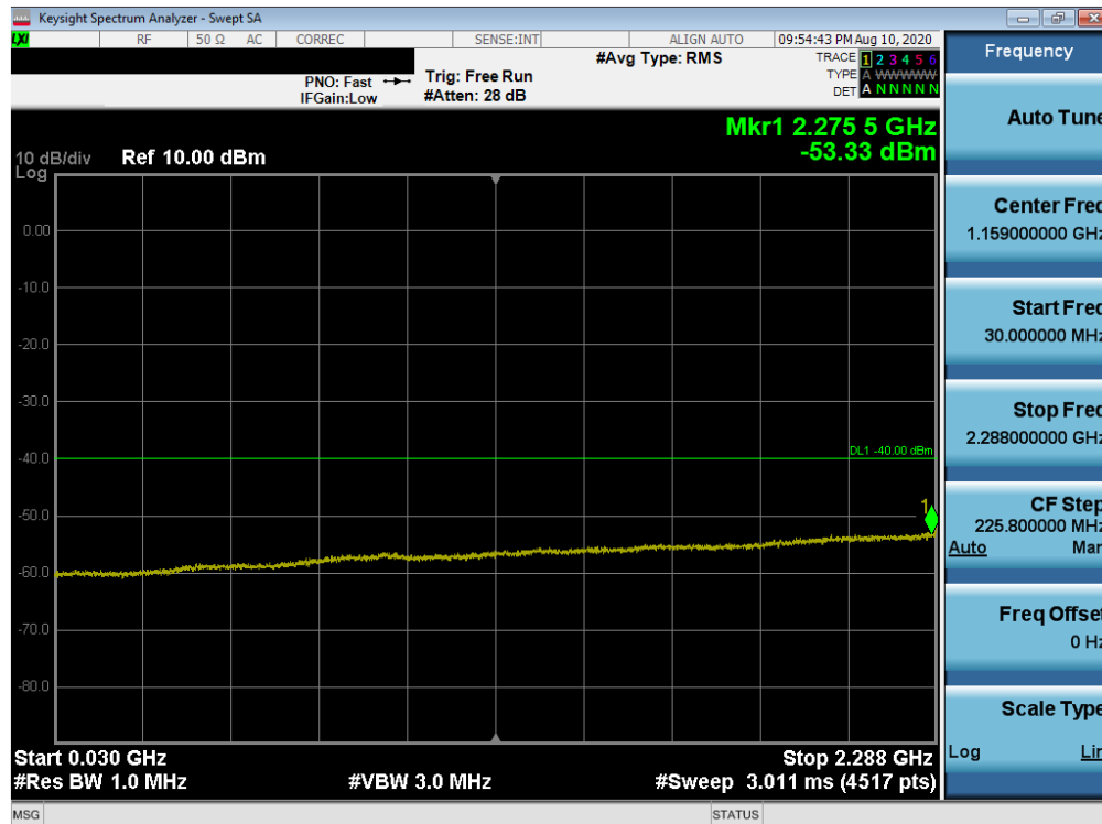
Plot 7-240. Conducted Spurious Plot (LTE Band 30 - 5MHz QPSK - RB Size 1, RB Offset 0 - Low Channel)
