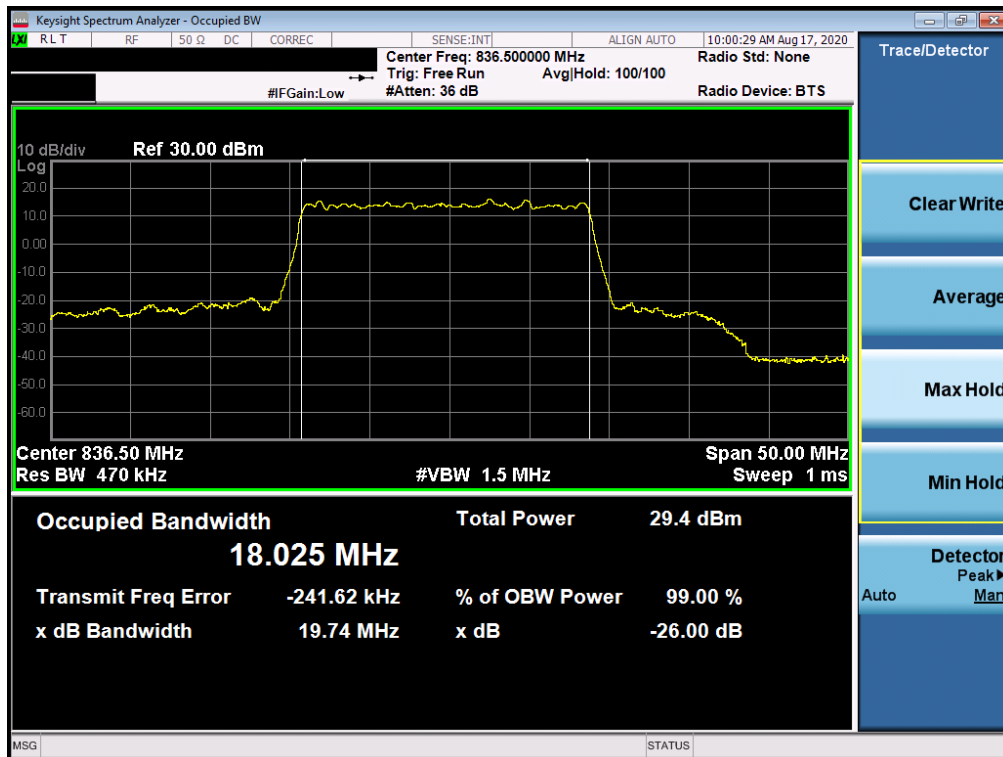
Plot 7-139. Occupied Bandwidth Plot (NR Band n5 - 20.0MHz CP-OFDM 256QAM - Full RB)
