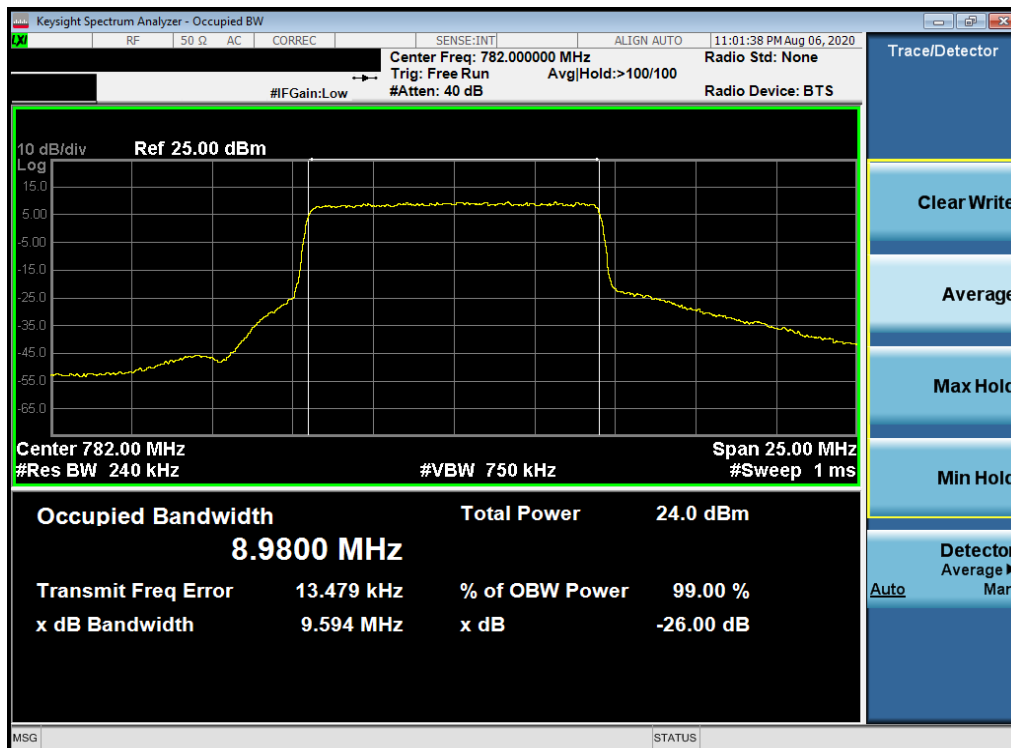
Plot 7-16. Occupied Bandwidth Plot (LTE Band 13 - 10MHz QPSK - Full RB Configuration)
