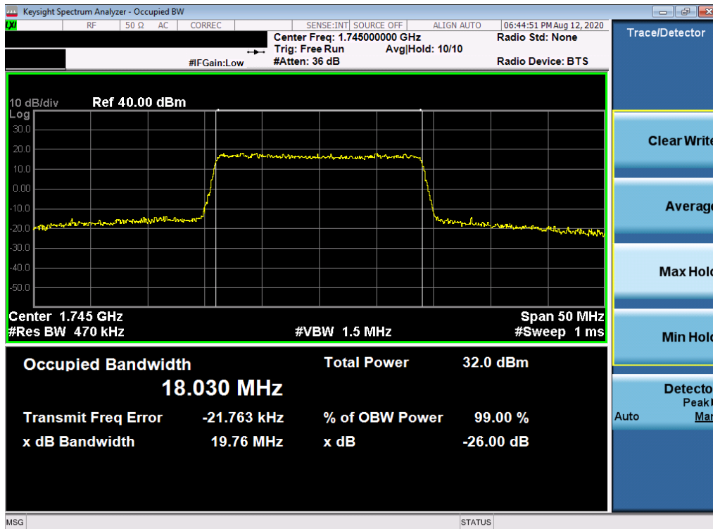
Plot 7-62. Occupied Bandwidth Plot (LTE Band 66/4 - 20MHz 16-QAM - Full RB Configuration)
