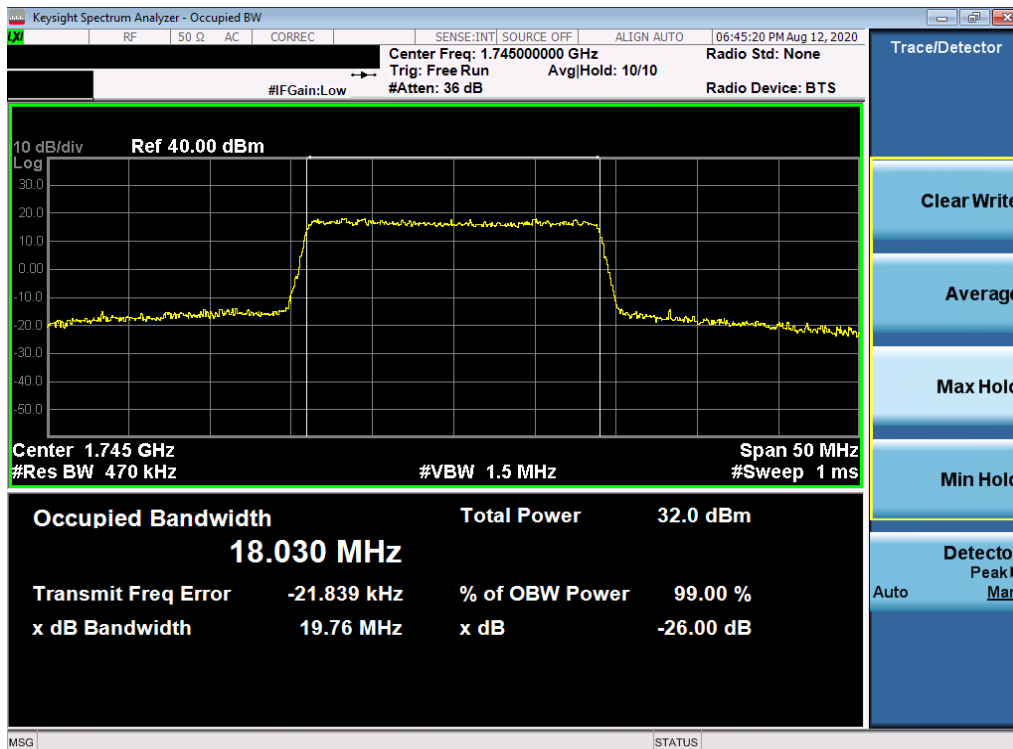
Plot 7-63. Occupied Bandwidth Plot (LTE Band 66/4 - 20MHz 64-QAM - Full RB Configuration)
