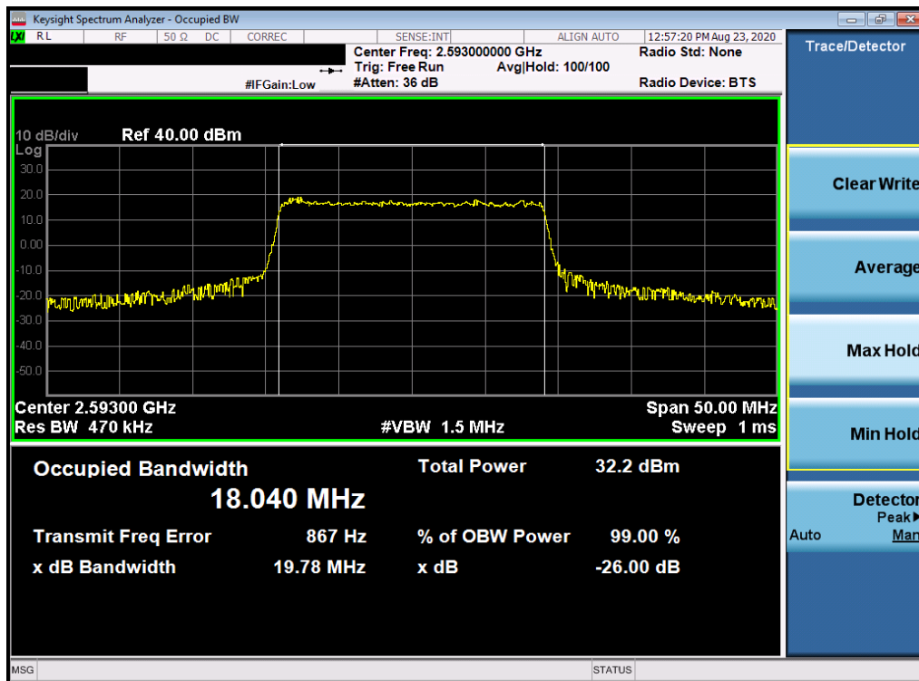
Plot 7-99. Occupied Bandwidth Plot (LTE Band 41(PC3) - 20MHz 64-QAM - Full RB Configuration)
