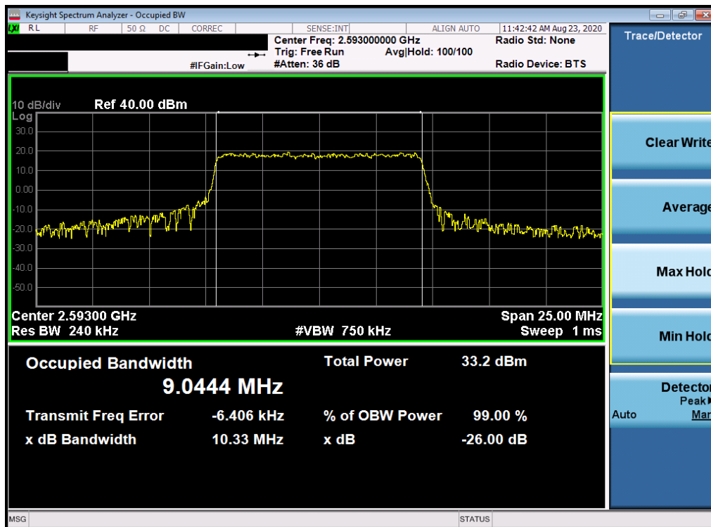
Plot 7-91. Occupied Bandwidth Plot (LTE Band 41(PC3) - 10MHz QPSK - Full RB Configuration)
