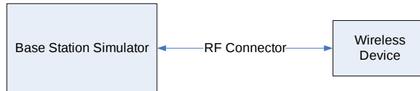
Figure 9-2 Power Measurement Setup
