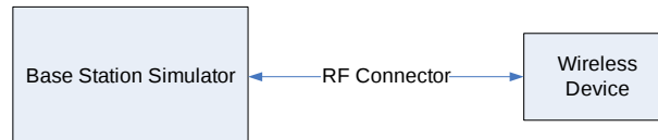
Figure 9-1 Power Measurement Setup
