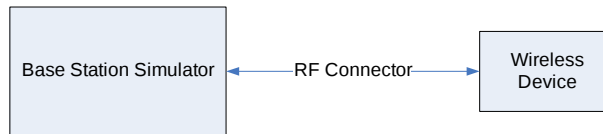
Figure 9-3 Power Measurement Setup
