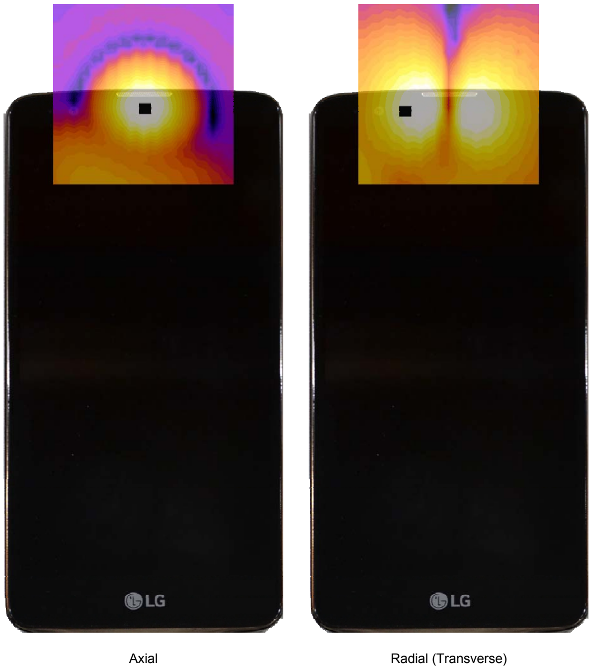
Figure 14-3 T-Coil Scan Overlay Magnetic Field Distributions
