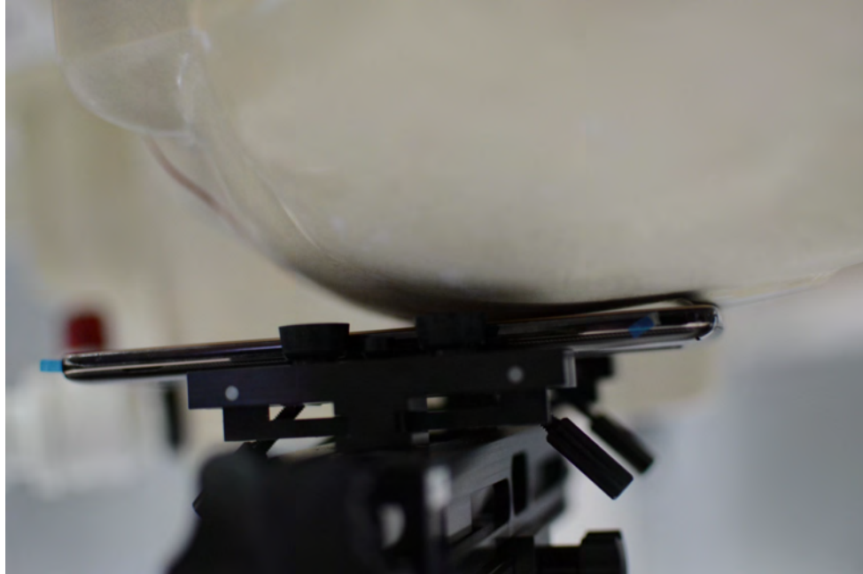
SAR Test Setup Photo 3: Left Cheek
