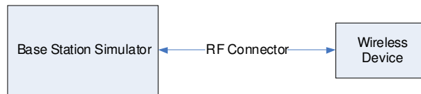
Figure 9-3 Power Measurement Setup
