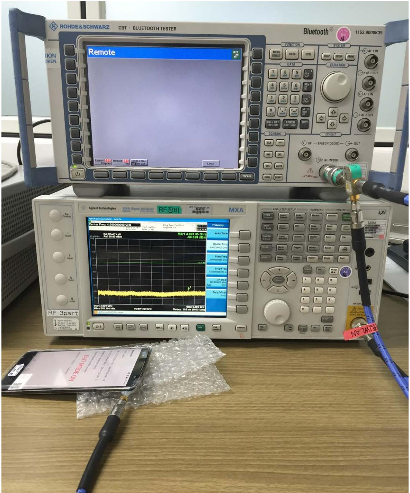
■ Conducted WLAN Test Setup Photo
