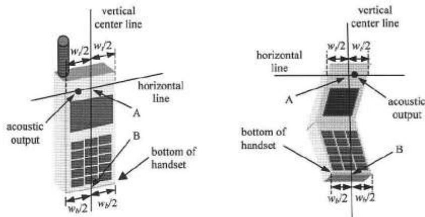
Figure 6-3. Handset vertical and horizontal reference lines
