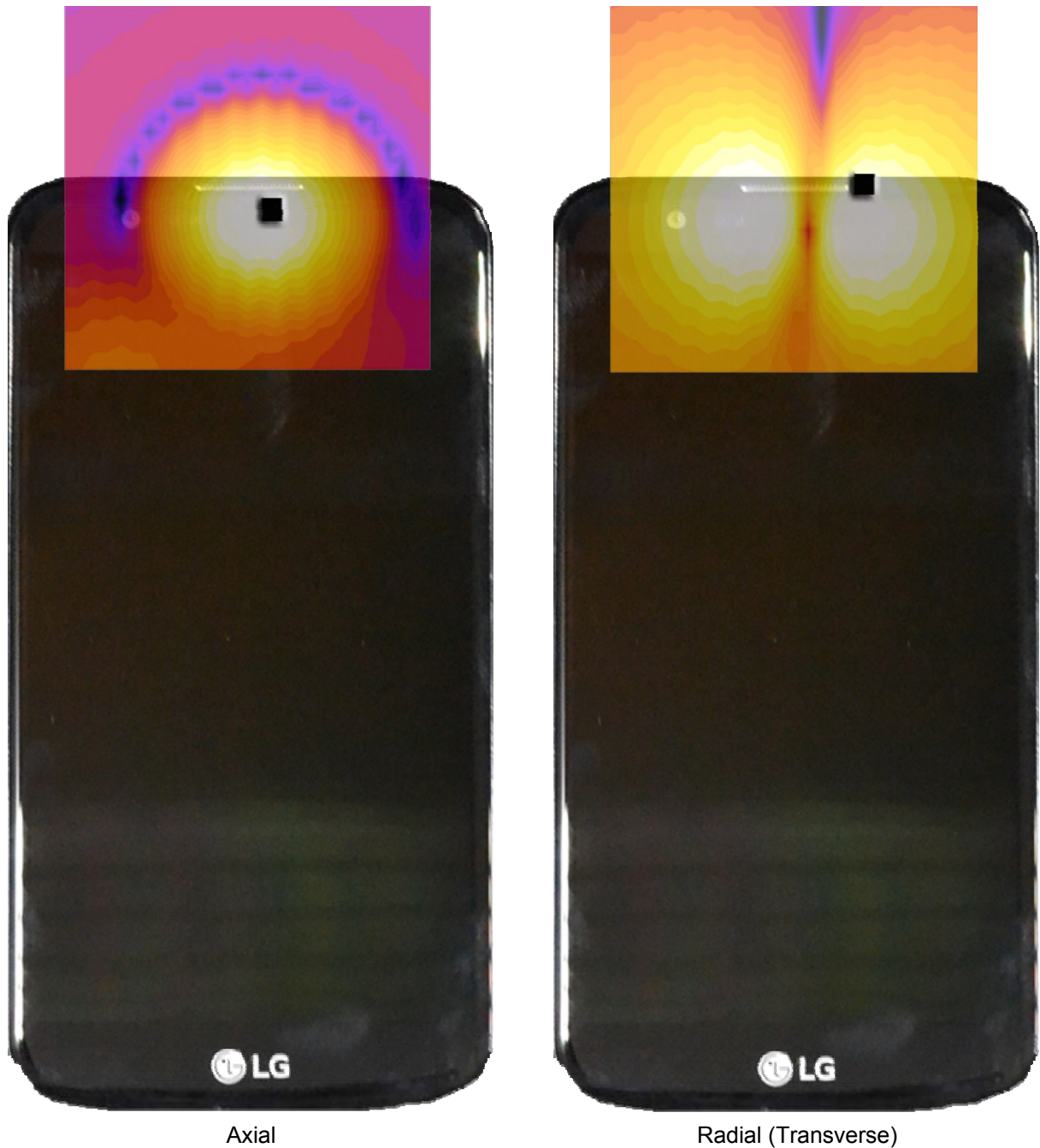
Figure 14-3 T-Coil Scan Overlay Magnetic Field Distributions
