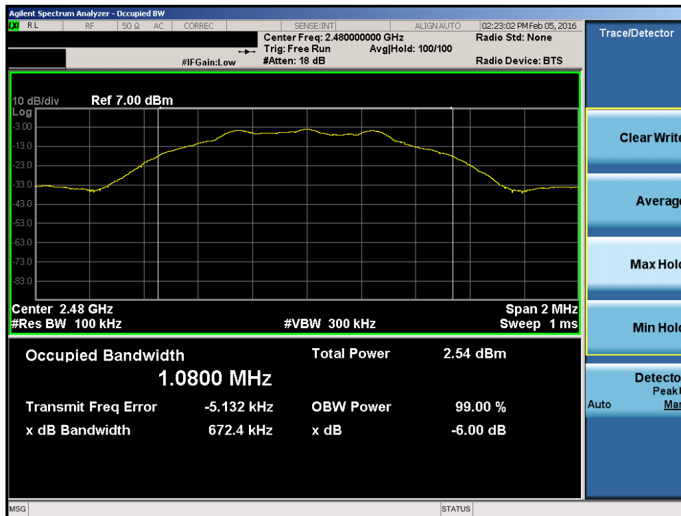
Plot 7-3. 6dB Bandwidth Plot (Bluetooth (LE) – Ch. 39)
