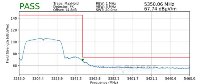
**Plot 7-16. Radiated Upper Band Edge Plot (Peak – UNII Band 2A)**
