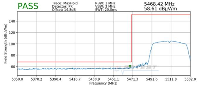
**Plot 7-18. Radiated Lower Band Edge Plot (Peak – UNII Band 2C)**
