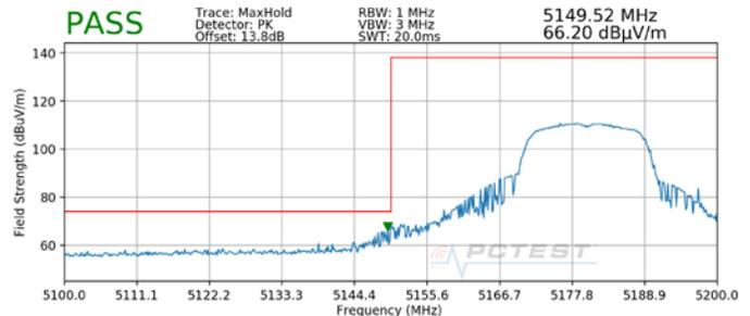
**Plot 7-7. Radiated Lower Band Edge Plot (Peak – UNII Band 1)**
