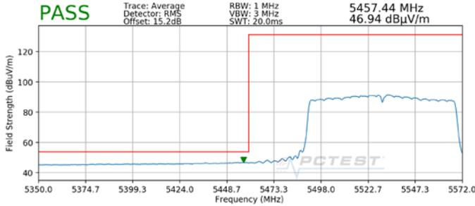
**Plot 7-24. Radiated Lower Band Edge Plot (Average – UNII Band 2C)**
