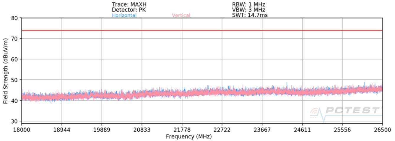
**Plot 7-5. Radiated Spurious Plot 18GHz - 26.5GHz (802.11a)**
