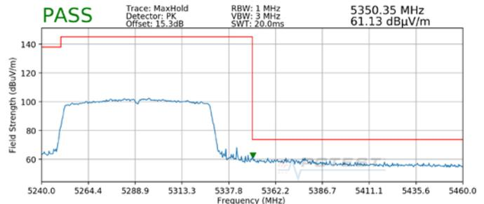
**Plot 7-23. Radiated Upper Band Edge Plot (Peak – UNII Band 2A)**
