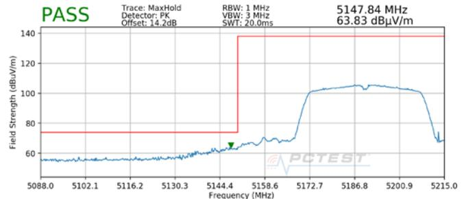
**Plot 7-14. Radiated Lower Band Edge Plot (Peak – UNII Band 1)**
