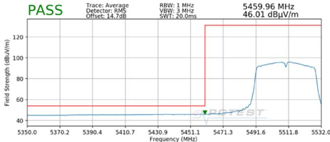
**Plot 7-17. Radiated Lower Band Edge Plot (Average – UNII Band 2C)**
