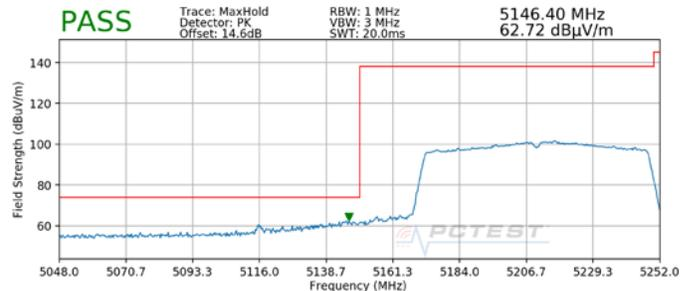
**Plot 7-21. Radiated Lower Band Edge Plot (Peak – UNII Band 1)**
