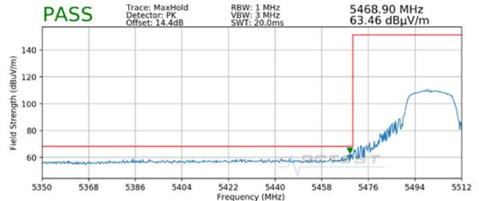
**Plot 7-11. Radiated Lower Band Edge Plot (Peak – UNII Band 2C)**
