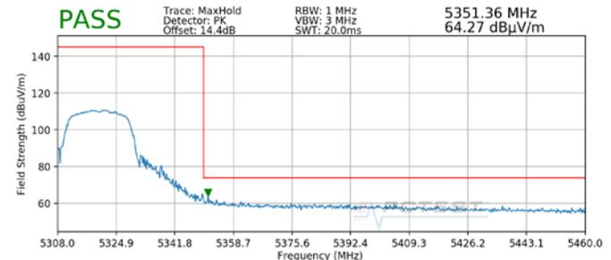
**Plot 7-9. Radiated Upper Band Edge Plot (Peak – UNII Band 2A)**
