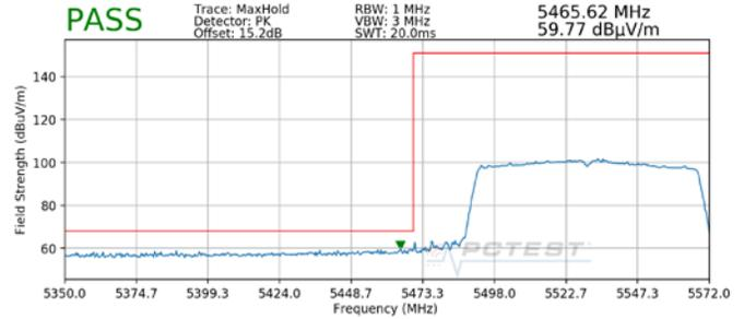
**Plot 7-25. Radiated Lower Band Edge Plot (Peak – UNII Band 2C)**
