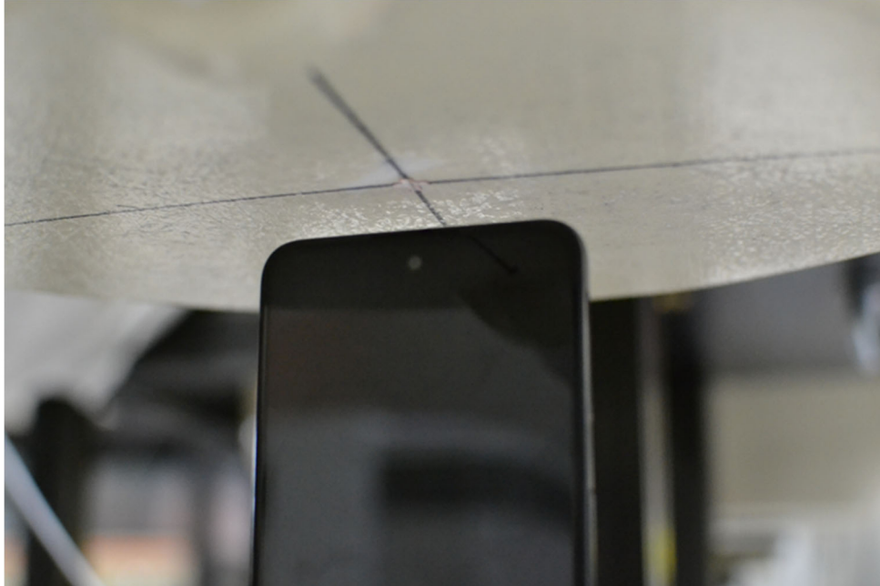
SAR Test Setup Photo 13 – Top Edge at 10 mm
