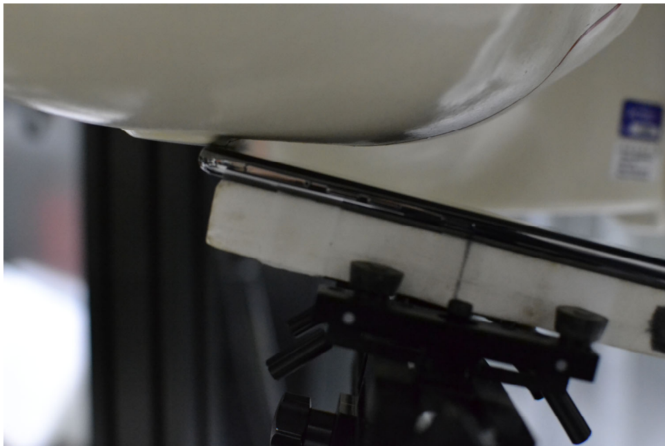
SAR Test Setup Photo 2 – Right Tilt
