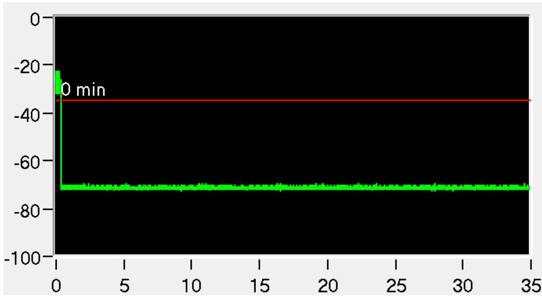
Figure 9-3. 5510MHz Band 2C Client Beacon Test – Monitoring live spectrum – Elapse time 30 minutes
