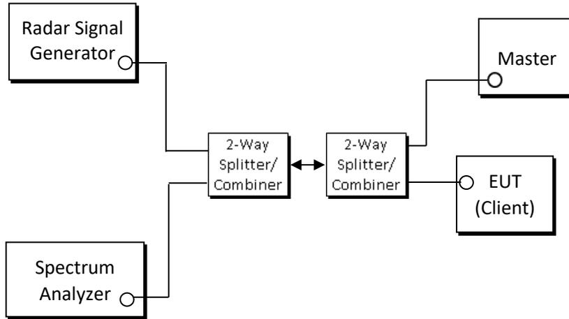
**Figure 8-1. Test Setup**
