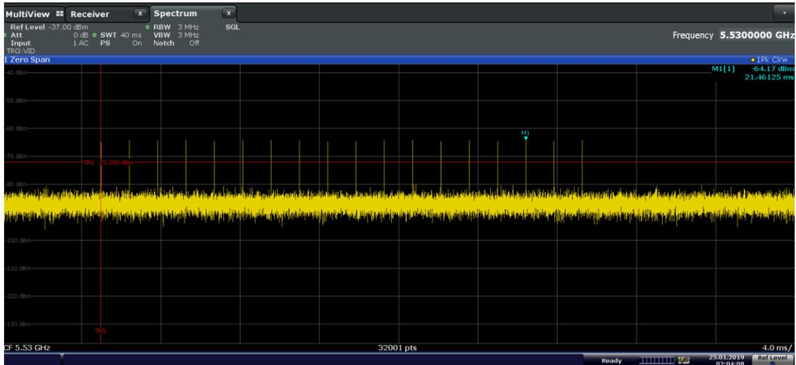
Figure 7-3. 5530MHz – Radar Pulse Type 0 (80MHz)
