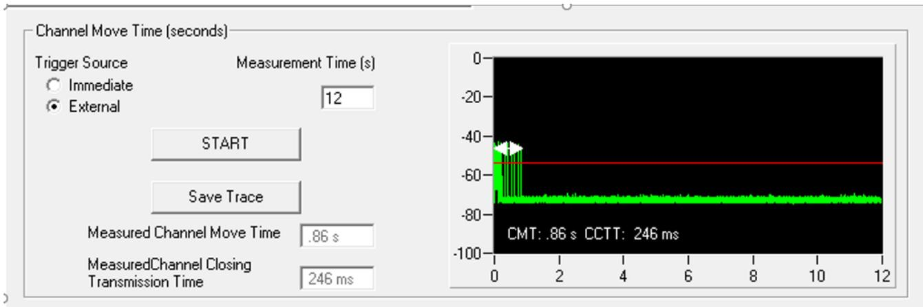
Figure 9-2. 5510MHz Band 2C Move Time and Channel Closing Transmission Time
