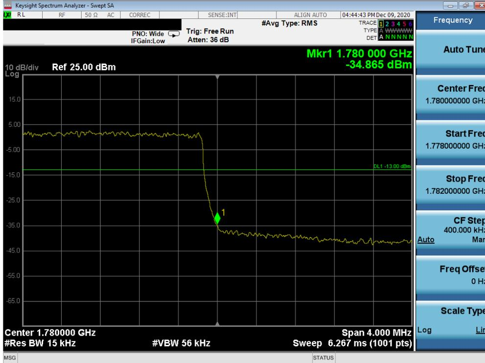
Plot 7-117. Upper Band Edge Plot (LTE Band 66 - 3MHz QPSK – Full RB Configuration)
