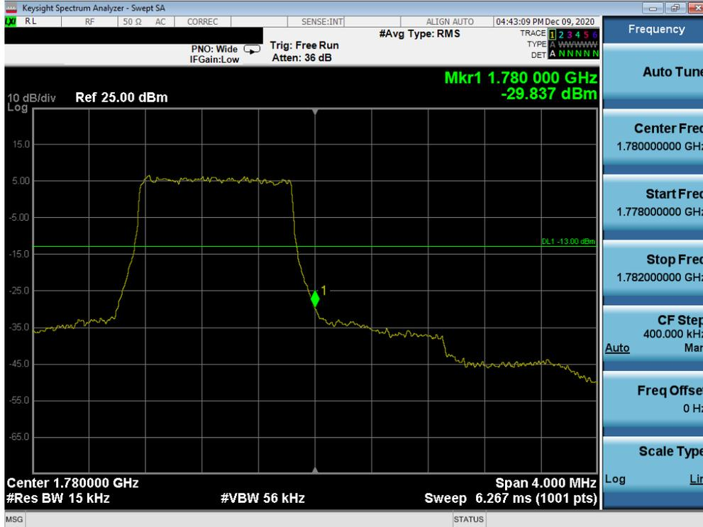
Plot 7-123. Upper Band Edge Plot (LTE Band 66 – 1.4MHz QPSK – Full RB Configuration)
