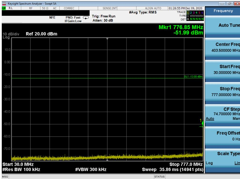
Plot 7-68. Conducted Spurious Plot (LTE Band 13 - 10MHz QPSK - RB Size 1, RB Offset 0)
