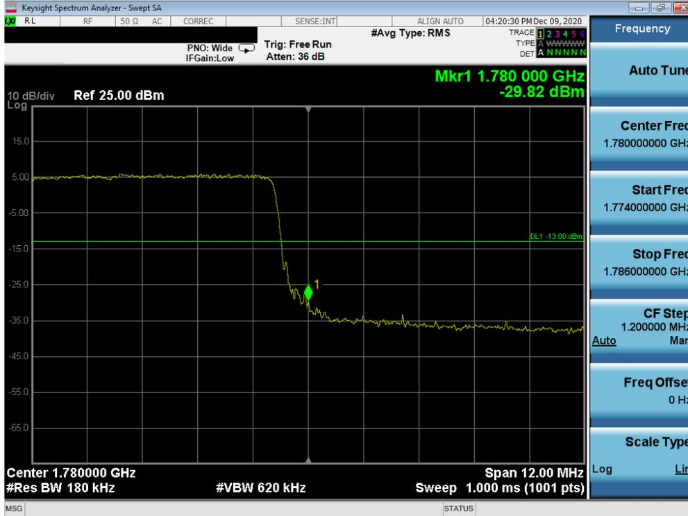
Plot 7-99. Upper Band Edge Plot (LTE Band 66 - 15MHz QPSK – Full RB Configuration)
