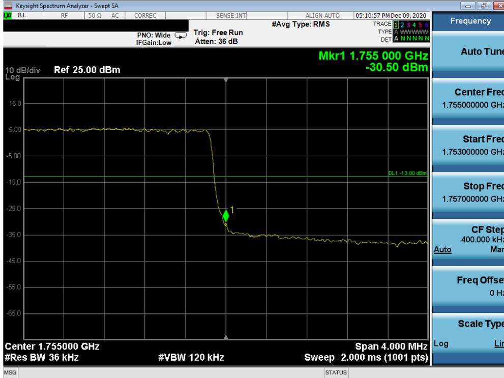
Plot 7-115. Upper Band Edge Plot (LTE Band 4 - 3MHz QPSK – Full RB Configuration)
