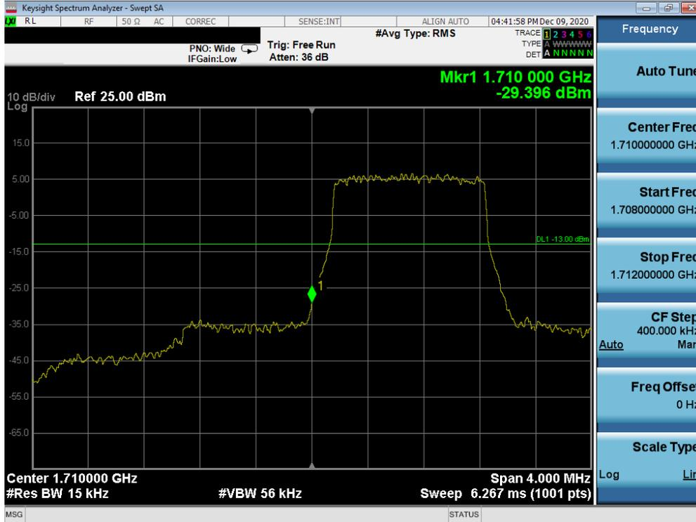
Plot 7-119. Lower Band Edge Plot (LTE Band 66/4 – 1.4MHz QPSK – Full RB Configuration)
