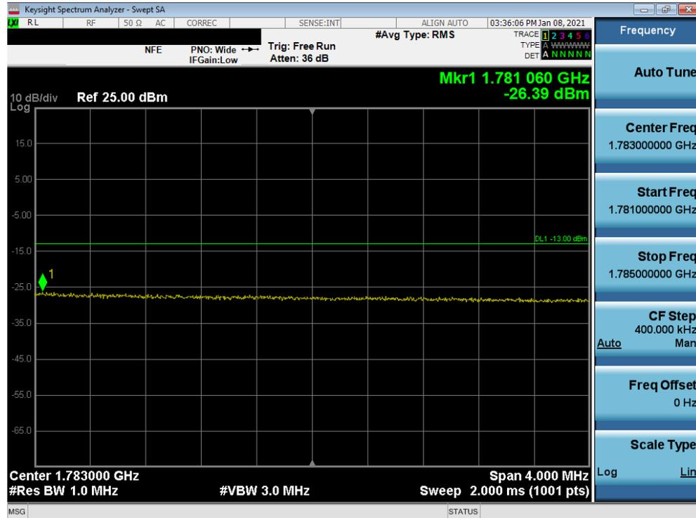
Plot 7-92. Upper Extended Band Edge Plot (LTE Band 4 - 20MHz QPSK – Full RB Configuration)
