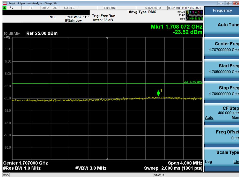
Plot 7-96. Lower Extended Band Edge Plot (LTE Band 66/4 - 15MHz QPSK – Full RB Configuration)
