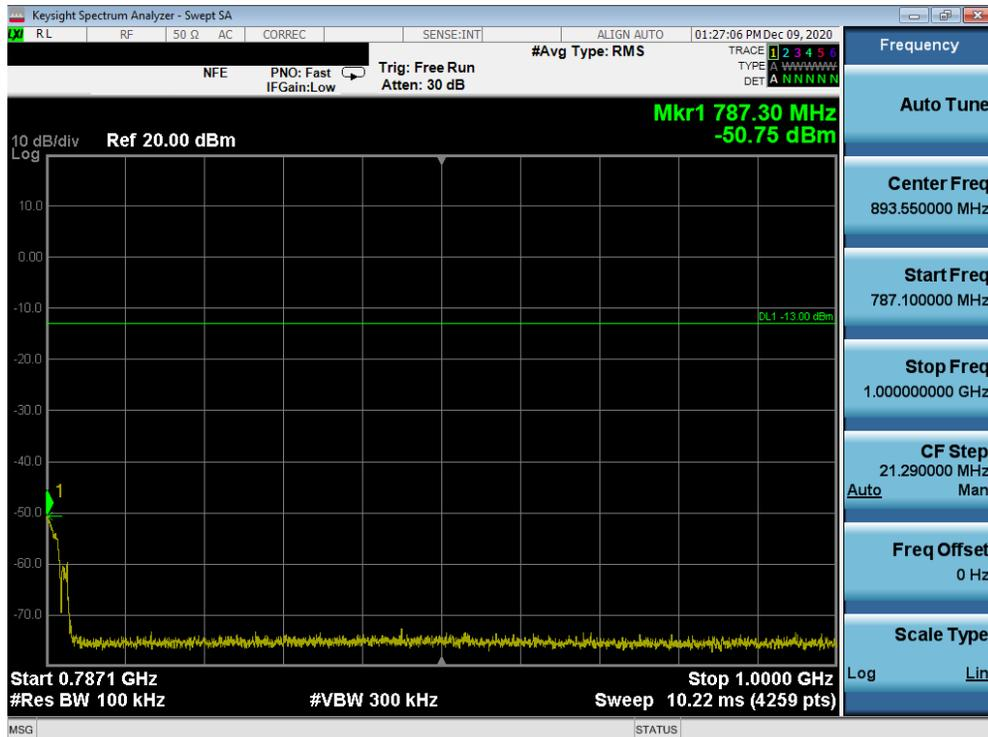
Plot 7-69. Conducted Spurious Plot (LTE Band 13 - 10MHz QPSK - RB Size 1, RB Offset 0)
