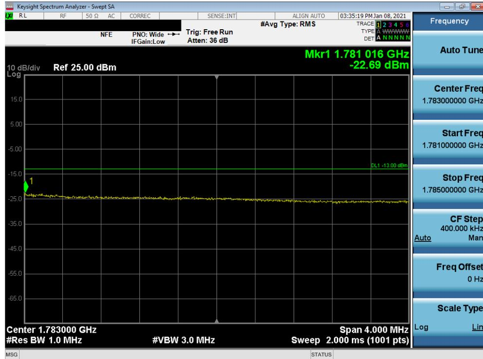
Plot 7-100. Upper Extended Band Edge Plot (LTE Band 66 - 15MHz QPSK – Full RB Configuration)
