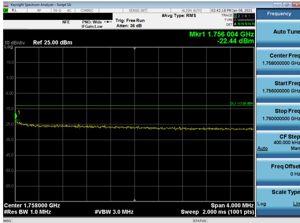
Plot 7-104. Upper Extended Band Edge Plot (LTE Band 4 - 10MHz QPSK – Full RB Configuration)
