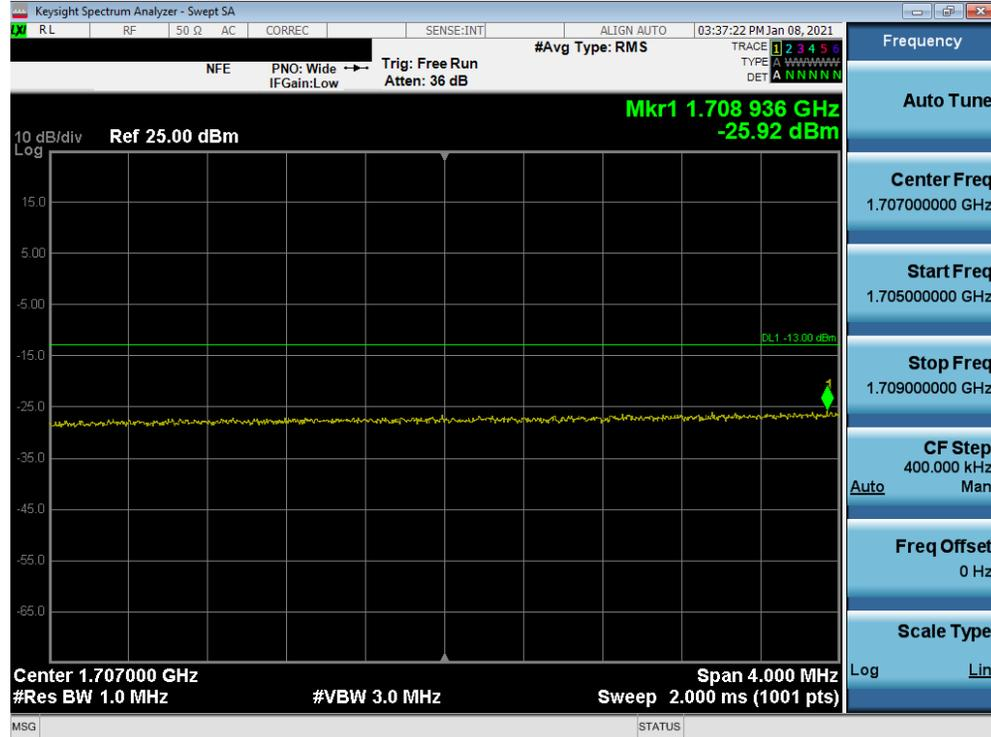
**Plot 7-90. Lower Extended Band Edge Plot (LTE Band 66/4 - 20MHz QPSK – Full RB Configuration)**
