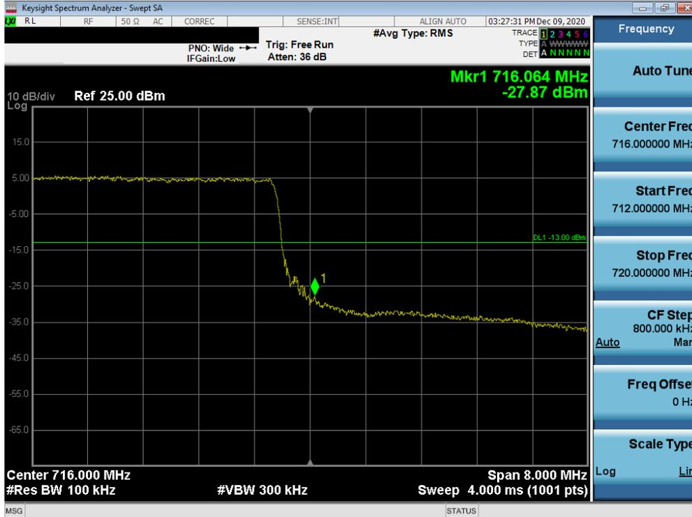
Plot 7-126. Upper Band Edge Plot (LTE Band 12 - 10MHz QPSK – Full RB Configuration)
