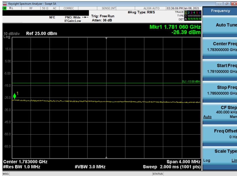
Plot 7-94. Upper Extended Band Edge Plot (LTE Band 66 - 20MHz QPSK – Full RB Configuration)
