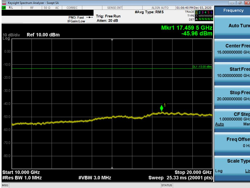
Plot 7-88. Conducted Spurious Plot (WCDMA Ch. 1513- High Channel)
