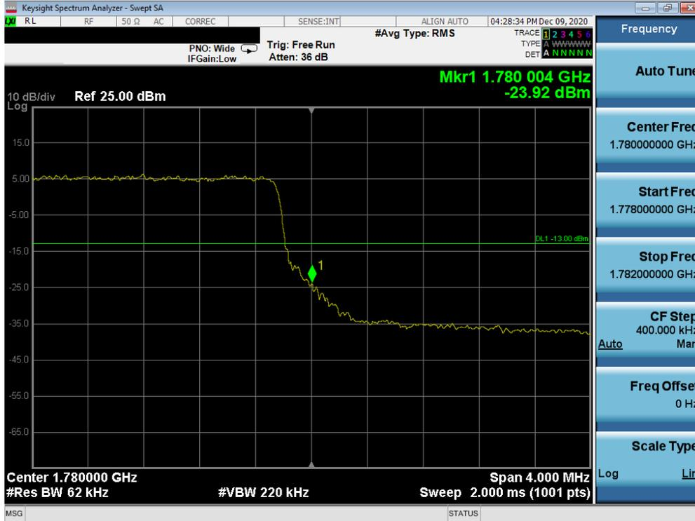
Plot 7-111. Upper Band Edge Plot (LTE Band 66 - 5MHz QPSK – Full RB Configuration)
