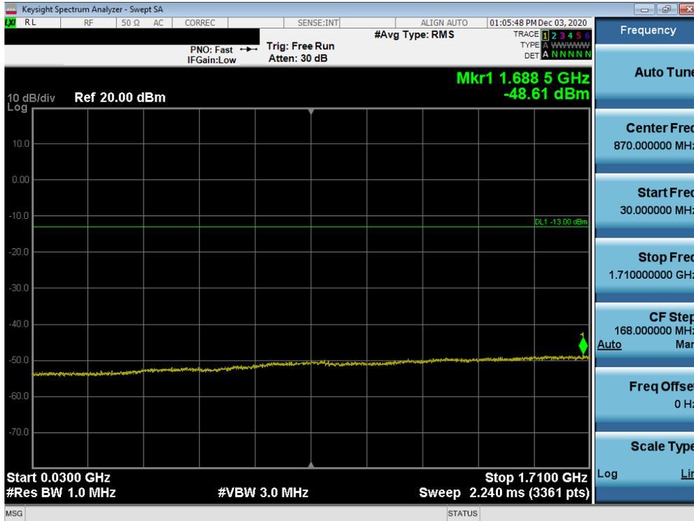
Plot 7-86. Conducted Spurious Plot (WCDMA Ch. 1513- High Channel)
