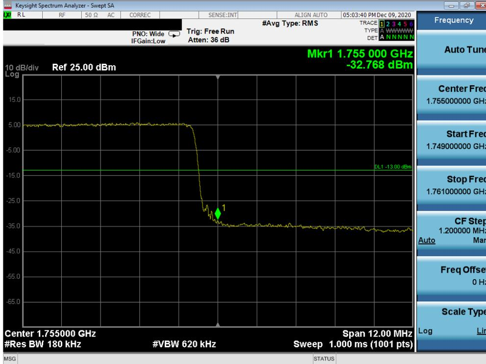
Plot 7-97. Upper Band Edge Plot (LTE Band 4 - 15MHz QPSK – Full RB Configuration)
