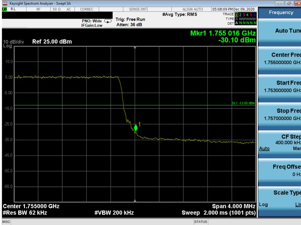
Plot 7-109. Upper Band Edge Plot (LTE Band 4 - 5MHz QPSK – Full RB Configuration)
