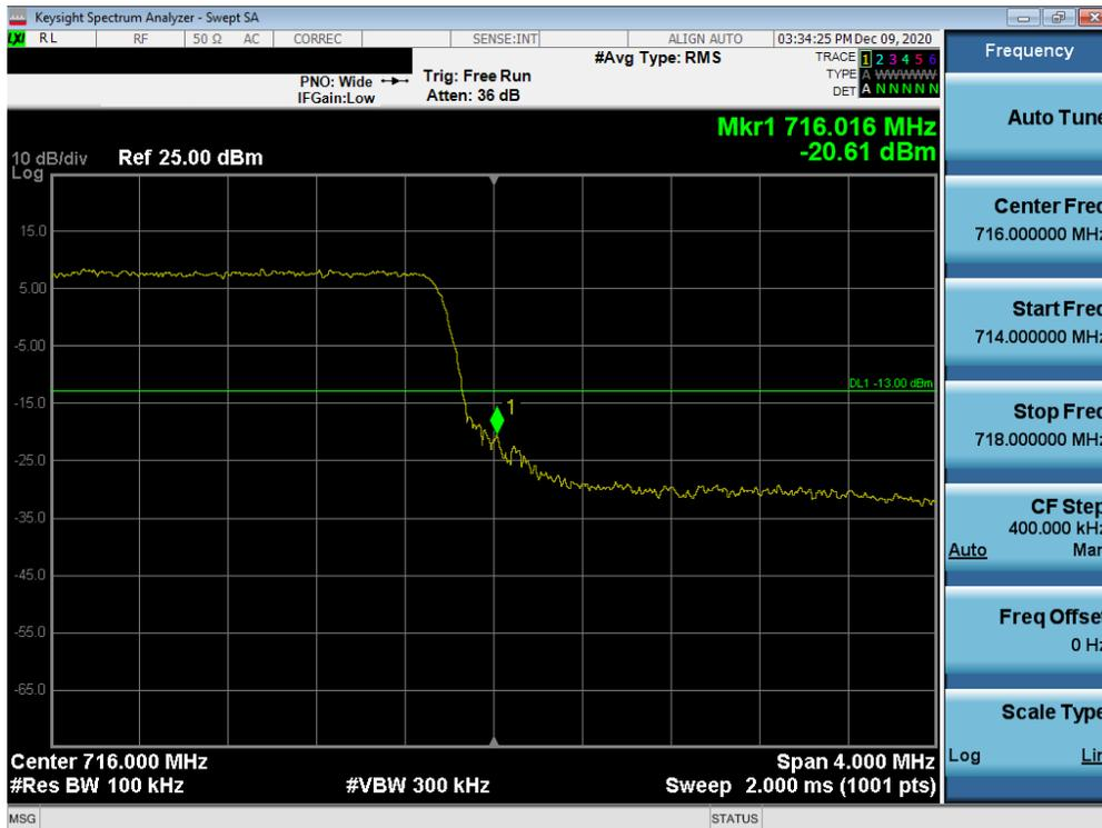
Plot 7-128. Upper Band Edge Plot (LTE Band 12 - 5MHz QPSK – Full RB Configuration)
